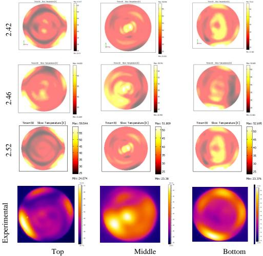
Fig. 7 Comparison of simulated and experimental temperature profile at 2.42, 2.46 and 2.52 GHz frequencies
