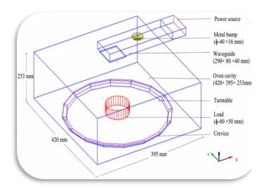
Fig. 1 Geometric model of microwave oven
