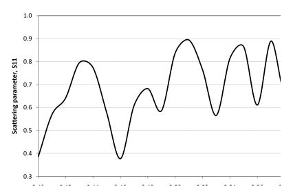
Fig. 4 Simulated scattering parameter S<sub>11</sub> at various frequencies of magnetron
