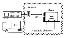
Fig. 3. Set up for magnetron frequency determination
