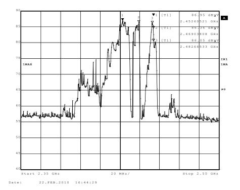
Fig. 5 Frequency spectrum of microwave oven
