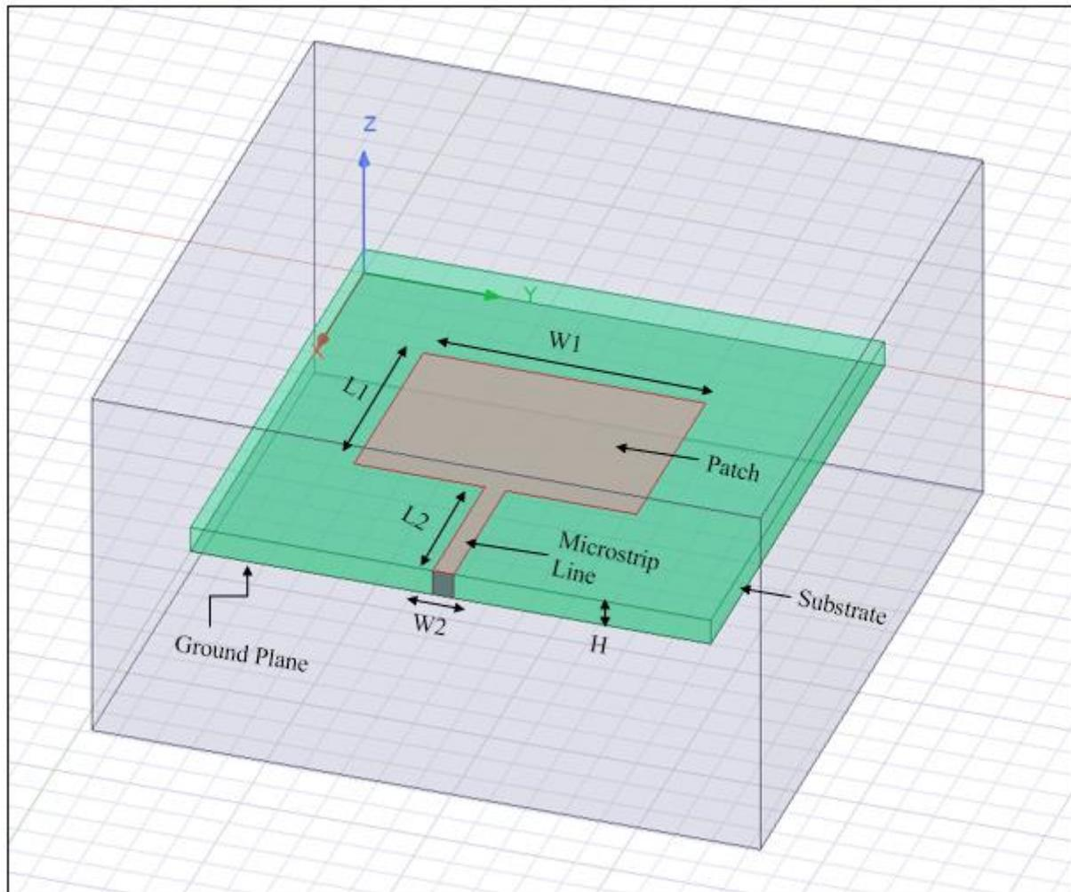
**Figure 2: A Microstrip Patch Antenna Design using Ansys HFSS.**
