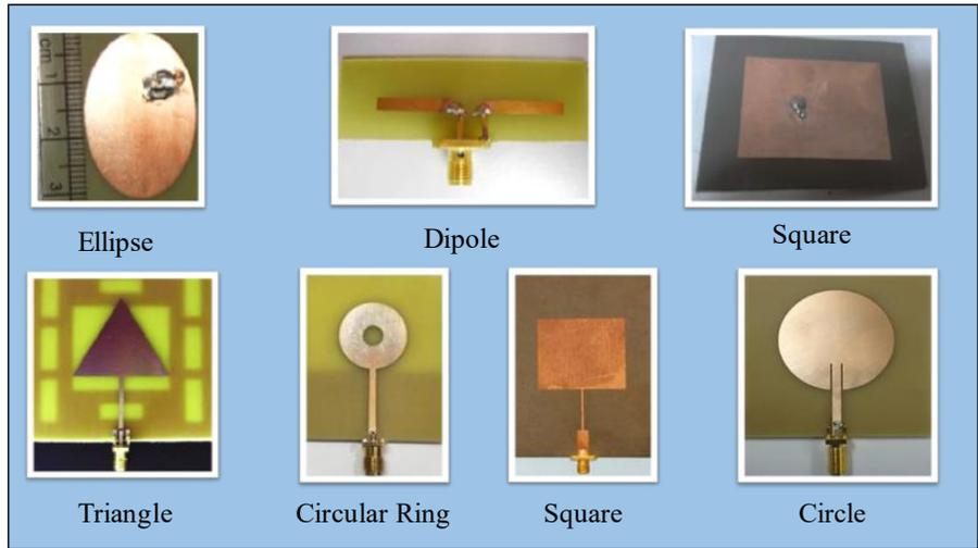
**Figure 3: Different Shapes of Microstrip Patch Elements.**
