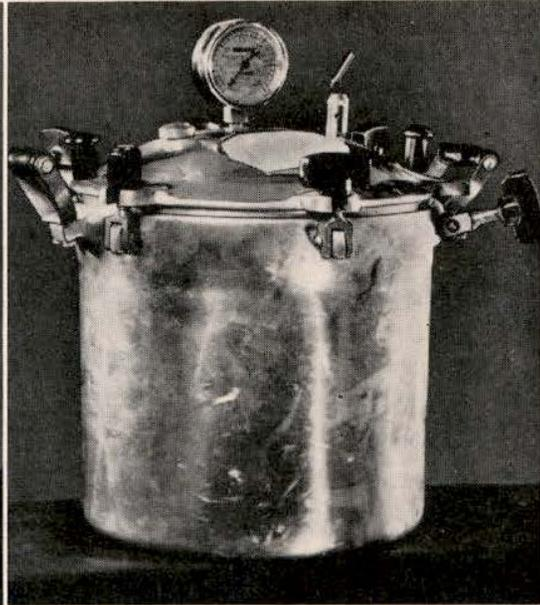
FIG. 2.—Cooker II, twelve-quart aluminum conventional-type seal using yoke bolts and wing nuts. Satisfactory dial on pressure gauge. Safety valve and petcock combined. Small knob at left of pressure gauge is a safety plug.
