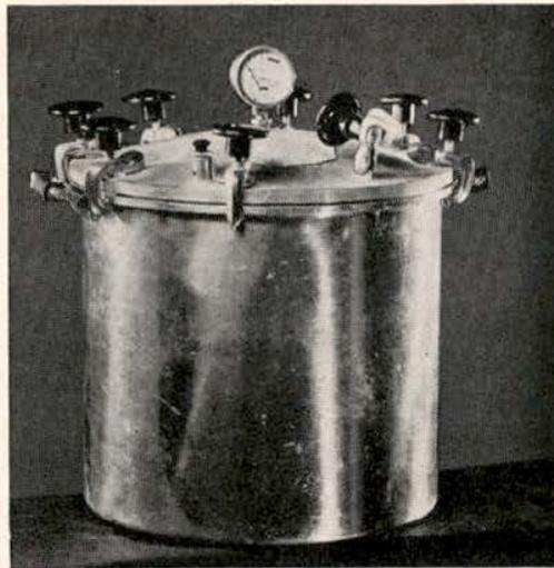
FIG. 3.—Cooker III, eighteen-quart aluminum, bead-and-groove-type seal using "C" clamps. Pressure gauge dial unsatisfactory because pointer movement is too small. Combined safety valve and petcock not the best because petcock must be held open to release air and steam.
