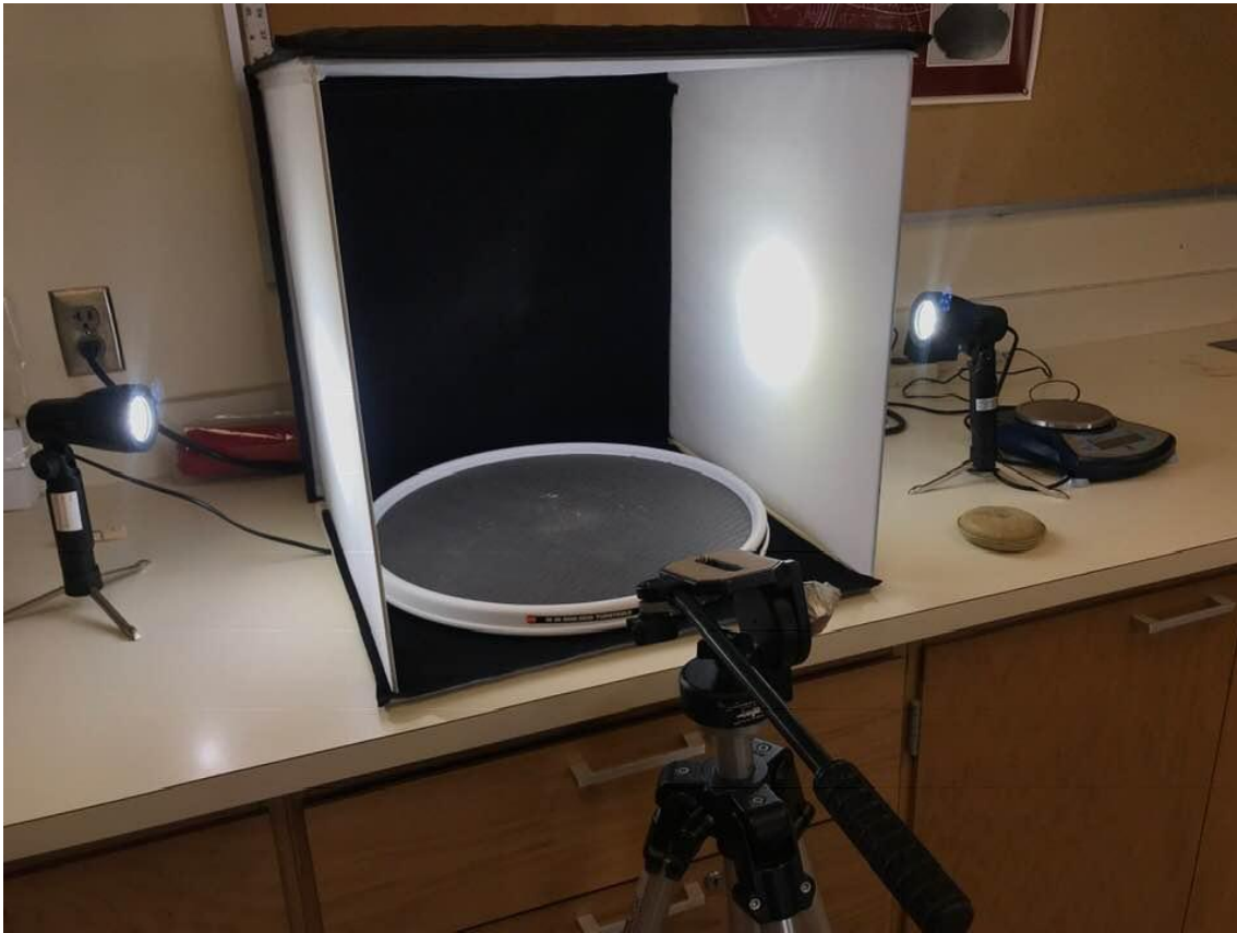
Fig 3.9. Example of a laboratory setup for photogrammetry with a light box, turntable, tripod, and artificial lighting.
