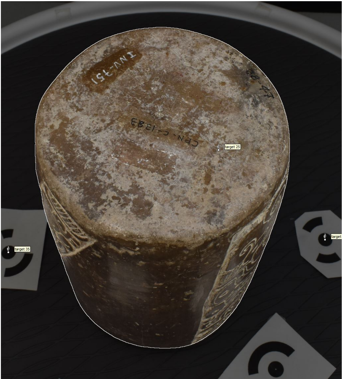
Fig 3.13. Masked photo that restricts point generation during the dense cloud process, note the white outline on the object, everything outside it is left out of processing.
