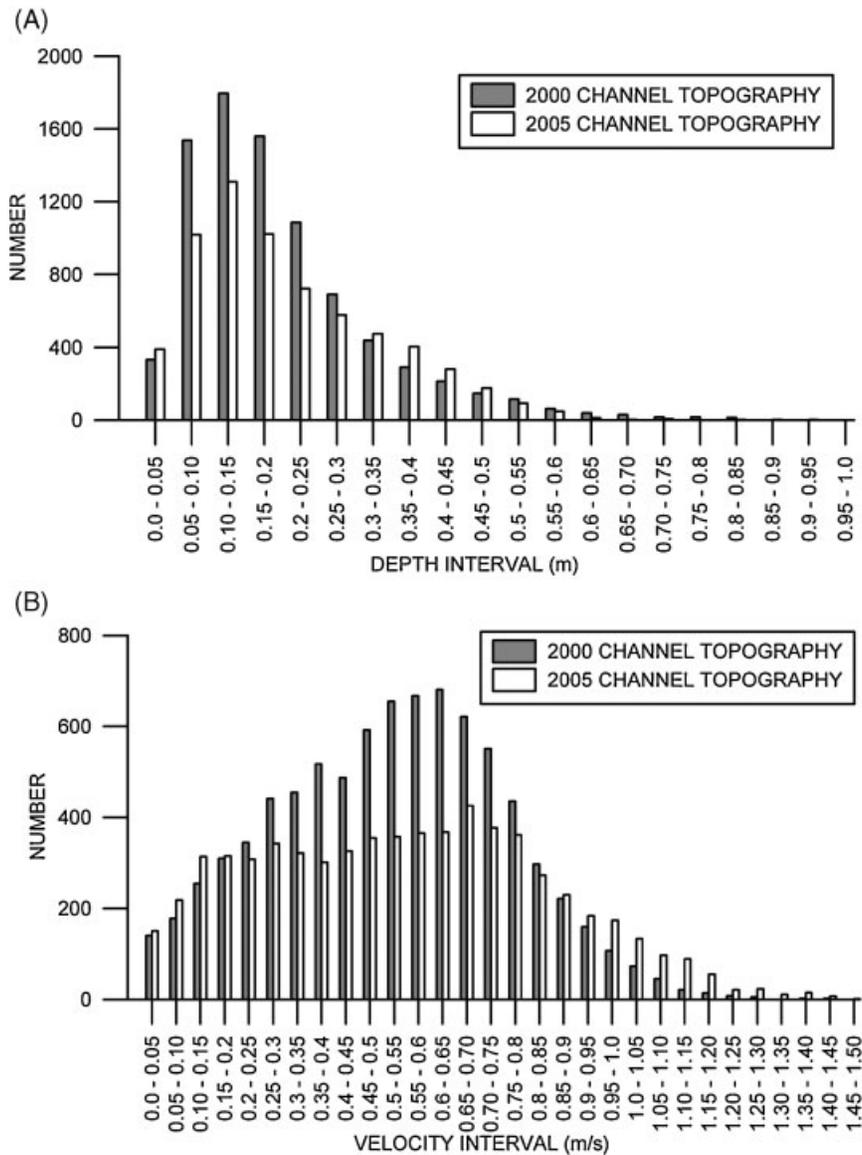
Figure 9. (A) Distributions of depths available in the Rowe Sanctuary reach computed by the hydraulic model for a streamflow of  $21 \text{ m}^3\text{s}^{-1}$  using the topography collected in 2000 and 2005. (B) Distributions of velocities available in the Rowe Sanctuary reach computed by the hydraulic model for a streamflow of  $21 \text{ m}^3\text{s}^{-1}$  using the topography collected in 2000 and 2005
