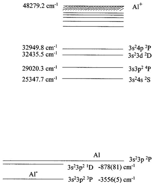
FIG. 1. Level diagram of the aluminum negative ion and atom. All energies shown are between the lowest of the fine-structure states and the Al  $3s^23p(^2P_{1/2})$  ground state.
