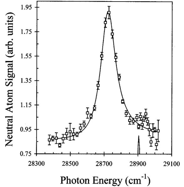
FIG. 3. Photodetachment data below the  $\text{Al } 3s^2 4s(^2S)$  threshold along with the result of a Beutler-Fano profile fit to the observed resonance. The best-fit parameters are  $q=12.4$ ,  $\Gamma=108 \text{ cm}^{-1}$ , and  $E_{\text{res}}=28717 \text{ cm}^{-1}$  with a reduced  $\chi^2$  of 2.65. The marker indicates the energy of the atomic state with respect to the  $3s^2 3p^2(^3P_0)$  negative ion state. The width of the marker indicates the uncertainty in the threshold position.
