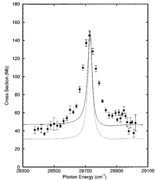
FIG. 5. Theoretically predicted total photodetachment cross section for  $\text{Al}^-$  in the photon energy region just below the first excited state threshold. Both dipole length (solid curve) and velocity (dashed curve) results are shown. Relative experimental data from Fig. 3 have been fit to the dipole length theoretical results using two parameters: the magnitude of the background cross section and the scaling factor to put the data on an absolute basis.
