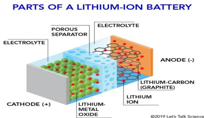
Fig 2.5 Schematic structure of a lithium-ion battery.
