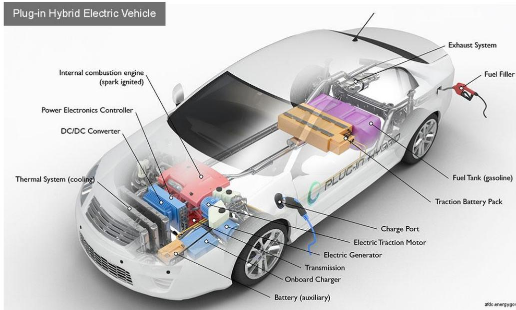
Fig 2.3 Key components of a plug-in hybrid electric vehicle.
