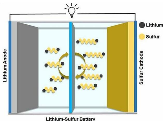
Fig 2.8 Schematic structure of a lithium-sulfur battery.
