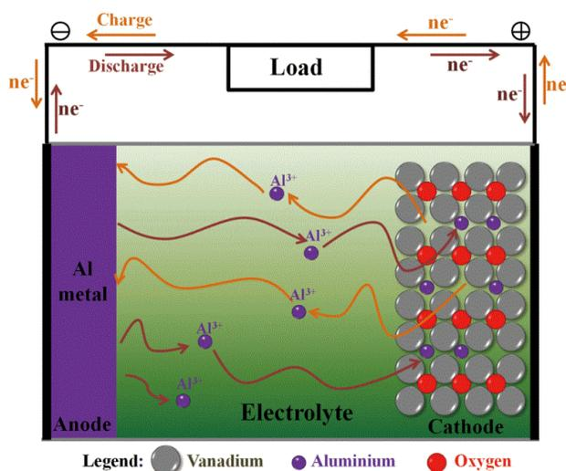
Fig 2.7 Schematic structure of an aluminum-ion battery.
