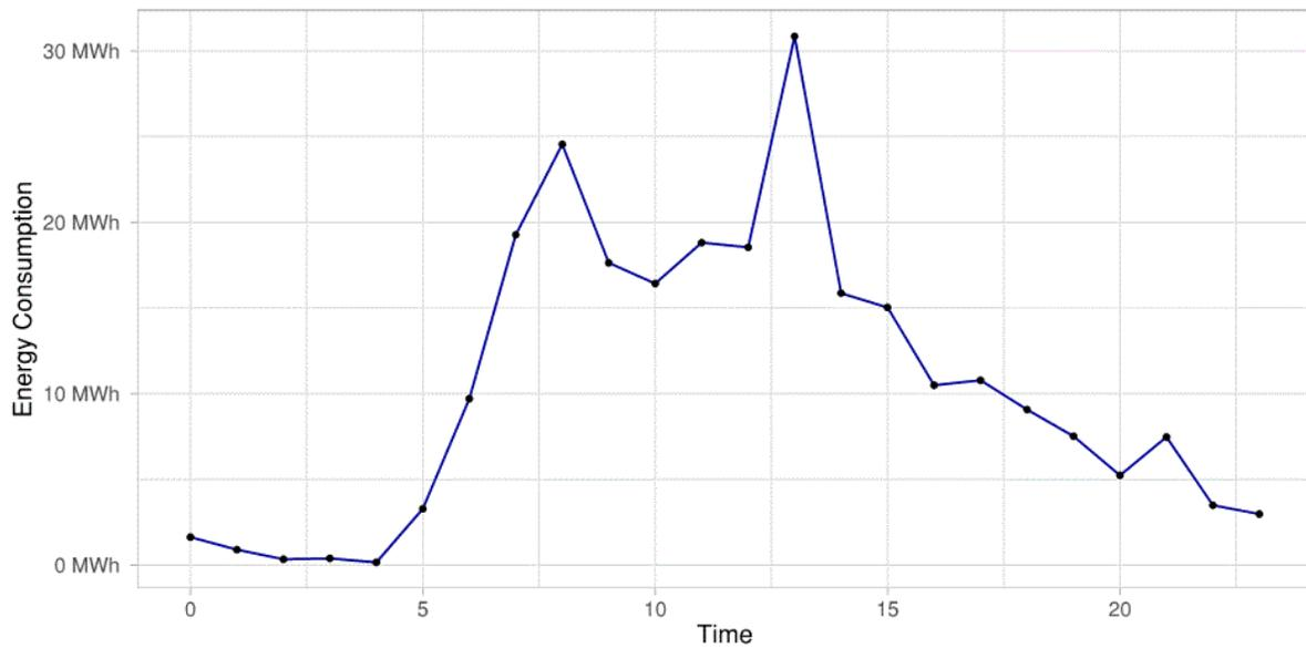
Fig. 4.11 Sum of kWh charged for given hour of the day since 2013.
