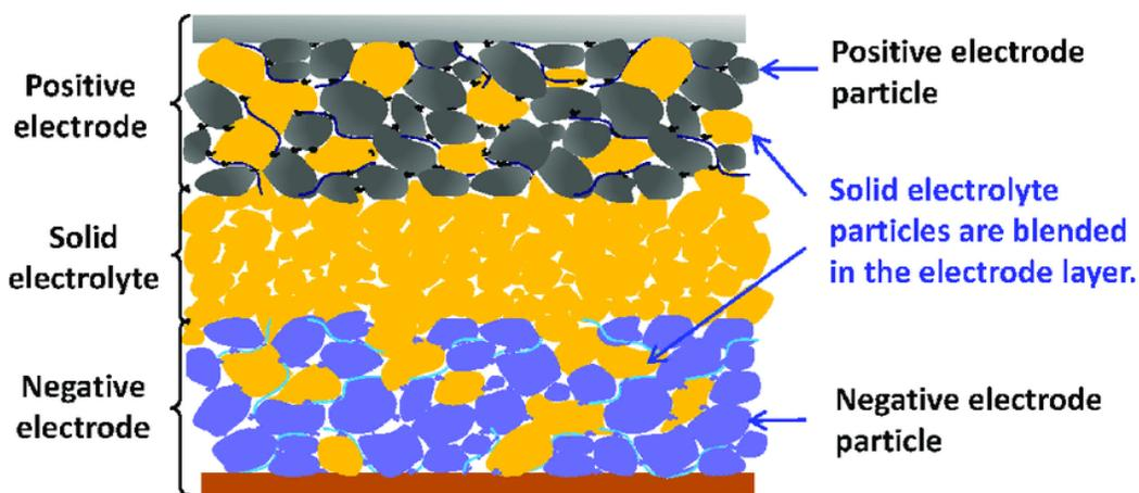
Fig 2.6 Schematic structure of a solid-state battery.
