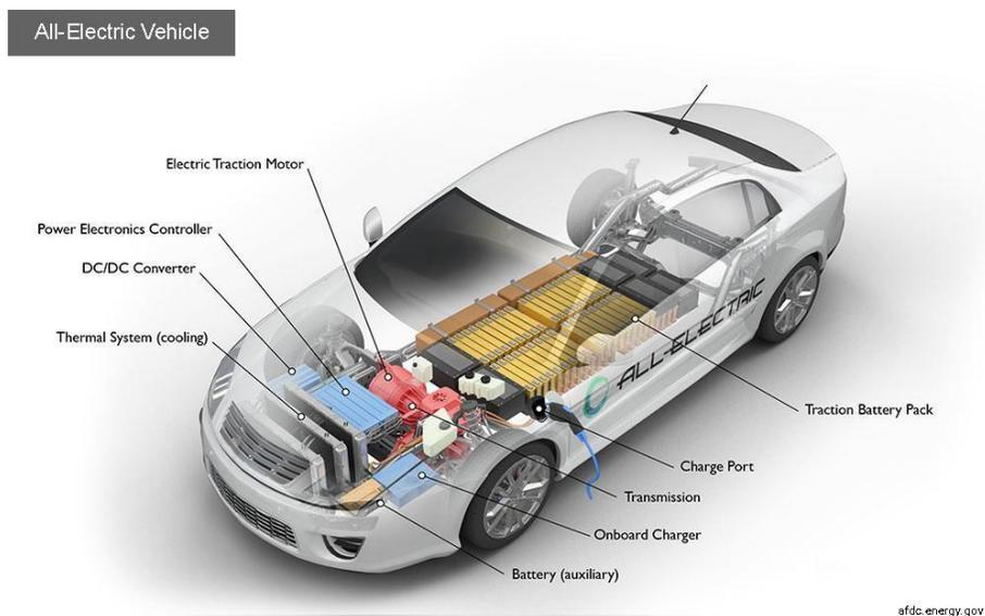
Fig 2.2 Key components of an all-electric vehicle.
