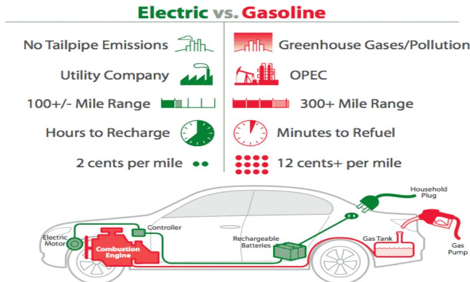
Fig 2.1 Major difference between electric vehicles and conventional vehicles.
