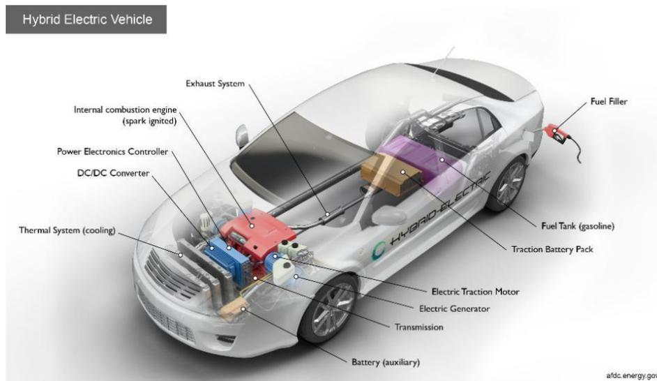
Fig 2.4 Key components of a hybrid electric vehicle.
