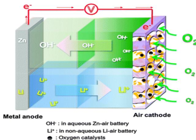
Fig 2.9 Schematic structure of a metal-air battery.
