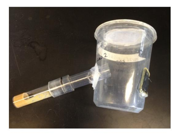
Fly cages are made with plastic cups with one panel window consisted of rubber square with a "X" shape opening to prevent flies from escaping and easy removal of flies with insertion of a aspirator. There is another opening with an extended tube attached with hot glue for food media access. The cover of cages are cut and cover with cheese cloth to ensure air circulations.
