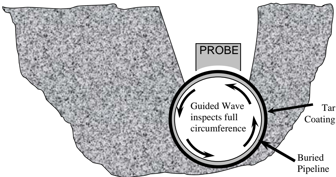
Figure 1: Full body inspection from the top surface of the pipe. There is no need to remove good coating or fully excavate the pipe to perform a complete inspection.
