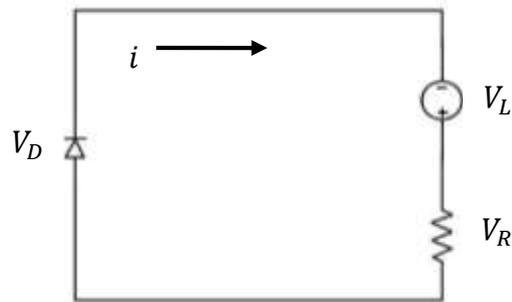
Figure 2-15. Circuit representing diode and load during switch off-state.
