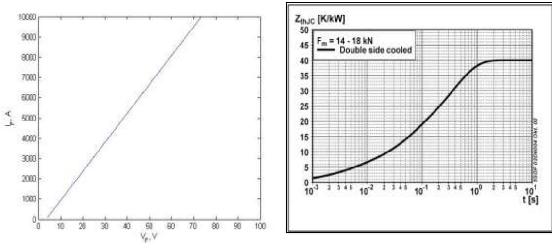
Figure 2-6. Si diode data used in thermal calculation. a) A V-I characteristic curve extrapolated to a current of 10 kA. b) Transient thermal impedance curve provide in diode
