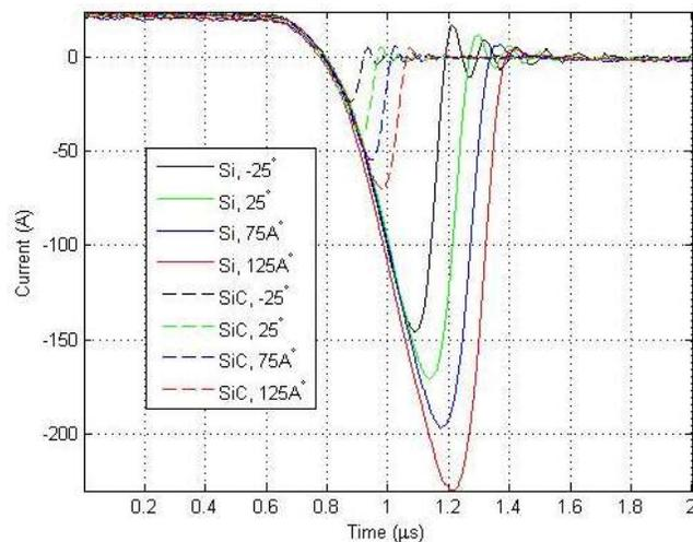
Figure 2-18. Comparison of reverse recovery waveforms for Si and SiC diodes at varying temperature and  $I_{F0} = 25\text{ A}$ .
