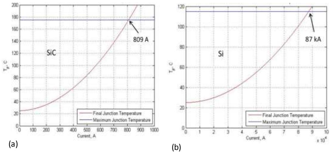
Figure 2-7. Device final junction temperature as a function of current. a) Cree SiC diode. b) ABB Si diode.
