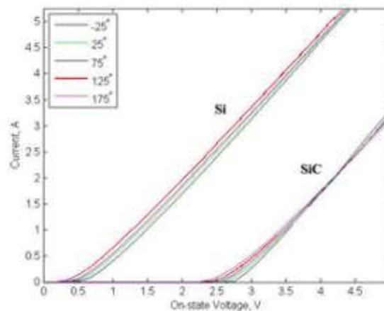
Figure 2-10. Temperature Dependence of Si and SiC low current V-I Characteristic.
