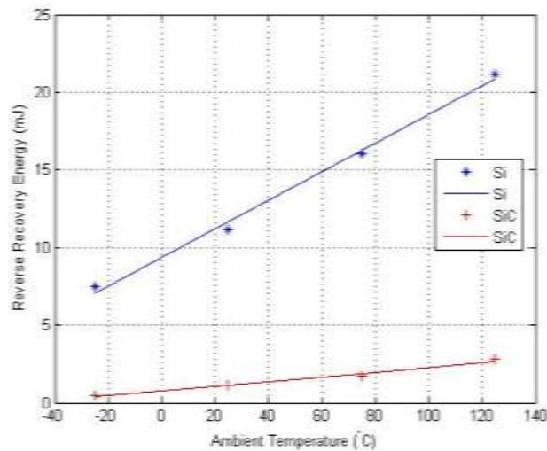
Figure 2-19. Data points and linear fit for reverse recovery energy,  $E_{rr}$ , at -25°C, 25°C, 75°C, and 125°C and  $I_{F0} = 25$  A for Si and SiC diodes.
