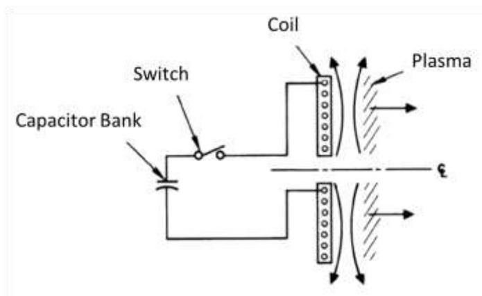
Figure 1-1. Schematic drawing illustrating IPPT operation- side view.
