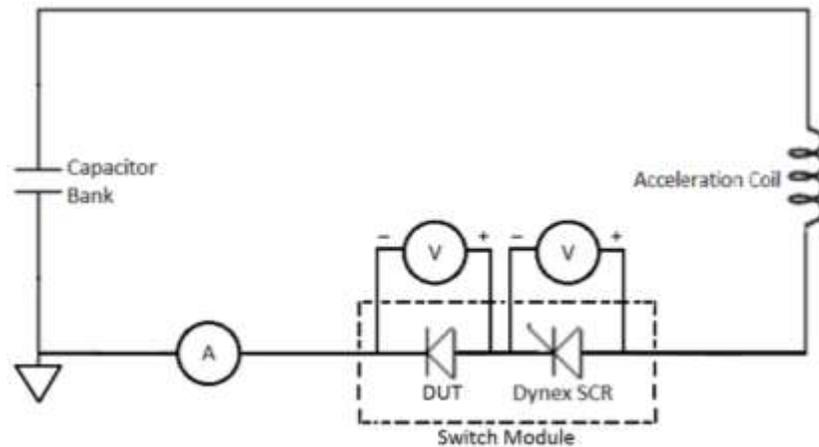
Figure 5-7. Circuit setup for ABB and Cree diode FPT testing.
