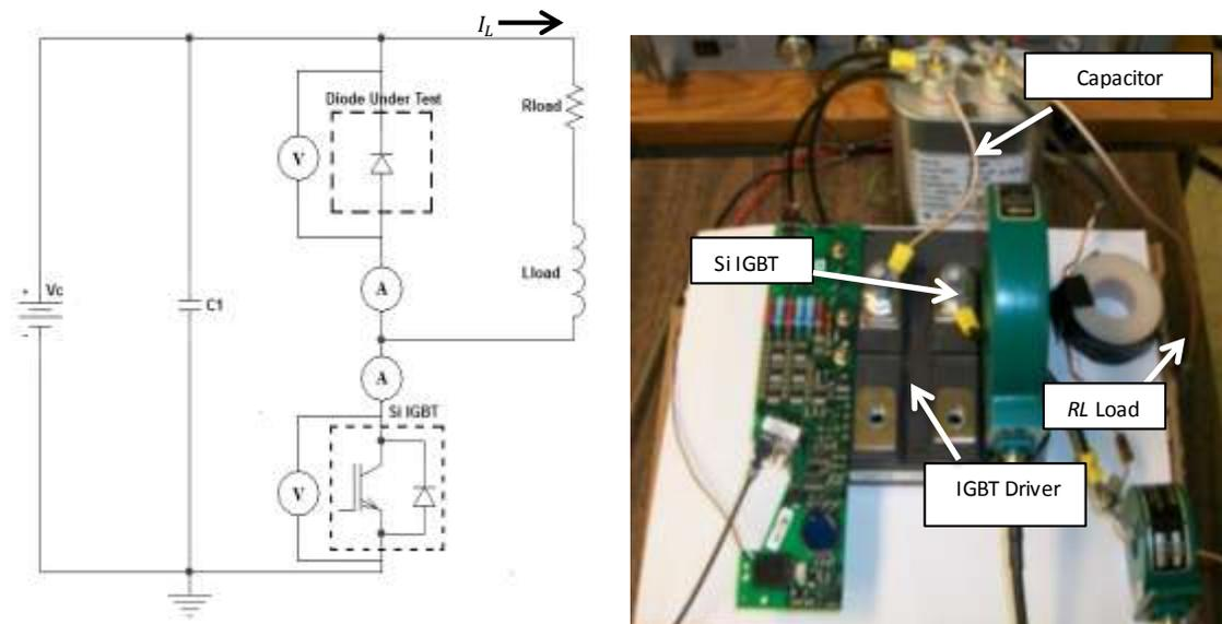
Figure 2-14. Diode dynamic characterization setup. a) Schematic representation of the double-pulse test circuit. b) Physical lab setup.
