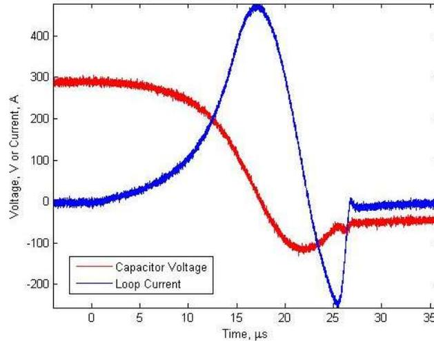
Figure 5-5. Dynex Diode Switching Waveforms. The capacitor bank voltage and loop current are shown on the same figure to demonstrate the effect of the diode reverse recovery on capacitor voltage reversal. The nominal charge voltage is 250 V.
