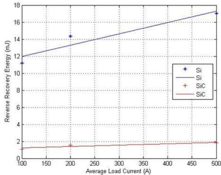
Figure 2-21. Data points and linear fit of reverse recovery energy,  $E_{rr}$ , at 25°C for  $I_{F0} = 25$  A, 37.5 A, and 50 A for Si and SiC.
