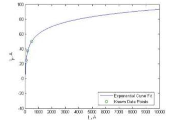
Figure 2-17. Exponential curve fit showing relationship between initial load current,  $I_{Lo}$ , and diode forward current,  $I_F$ .
