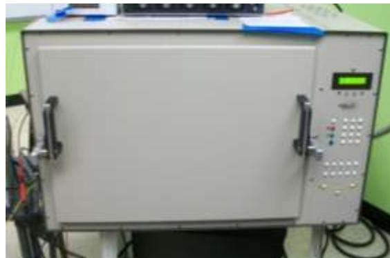
Figure 2-9. Sun Electronic Systems thermal chamber used to heat or cool device under test to the desired temperature.
