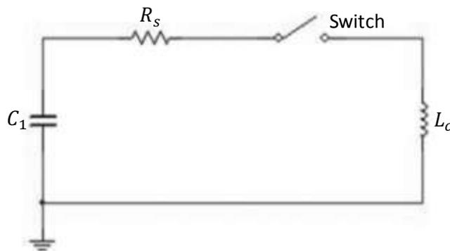
Figure 1-3. Series  $RLC$  circuit representing a basic IPPT circuit.
