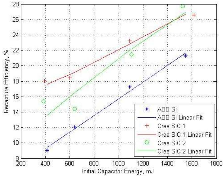
Figure 5-12. Percent energy recapture efficiency as a function of initial capacitor voltage for Si and SiC diodes.
