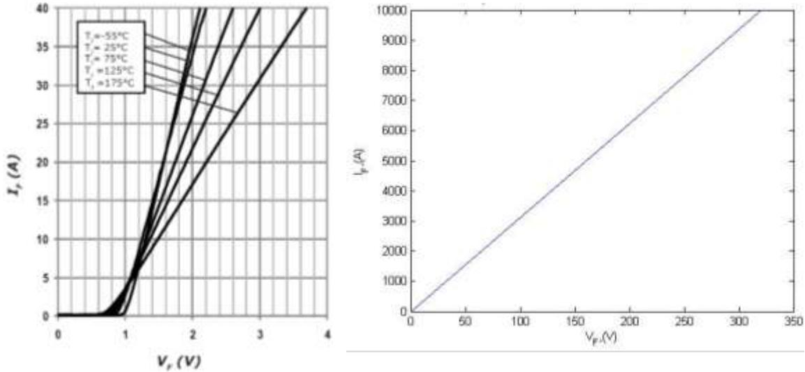
Figure 2-2. V-I characteristic curves for Cree C4D20120A SiC diode. a) Manufacturer-provided V-I curves. b) Curve at  $25^\circ\text{C}$  extrapolated to a current of 100 kA.
