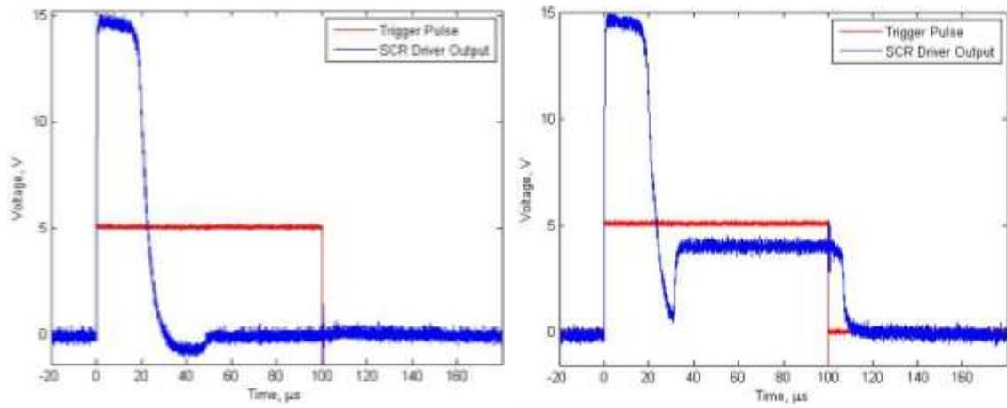
Figure 5-1. SCR driver output pulse. a) With no backporch, the pulse is approximately 20  $\mu\text{s}$  long, as fixed by the circuit. b) With the backporch on, the duration of the backporch is set by the length of the trigger. pulse.
