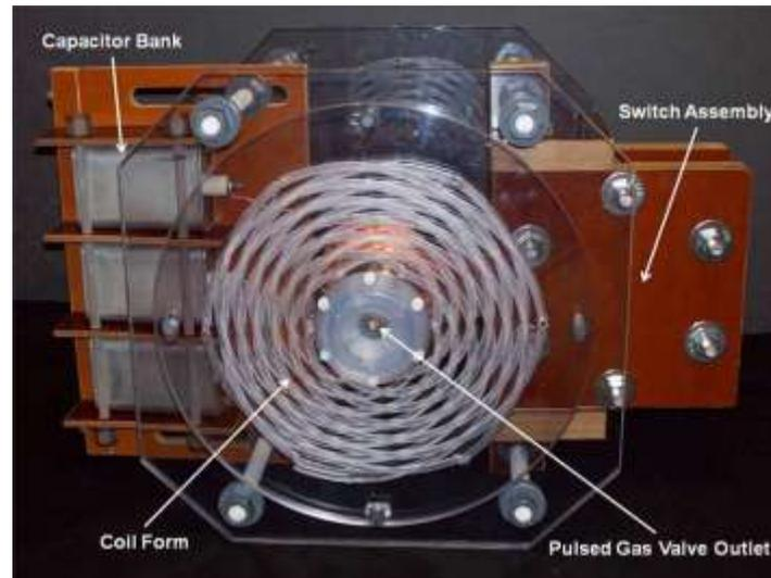
Figure 4-1. Photograph of Flat-Plate Thruster Lexan frame structure. The unfinished capacitor bank, switch assembly block, and Lexan acceleration coil form are shown temporarily mounted on the frame to give the reader an idea of the thruster configuration.
