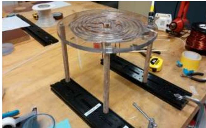
Figure 4-2. Setup for fabrication of the Flat-Plate Thruster acceleration coil. Phenolic post are used to elevate and secure the coil. The post are screwed in to optical rails which, in turn, are secured to the table using 'C' clamps.
