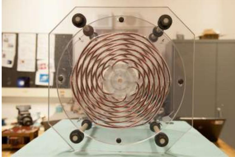
Figure 4-3. Flat-Plate Thruster Acceleration Coil (front view). The pulsed gas valve holder is attached in the center of the coil form, and aids in holding the leads in place.
