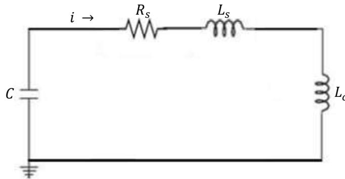
Figure 3-1. Basic RLC electrical circuit model for IPPT.
