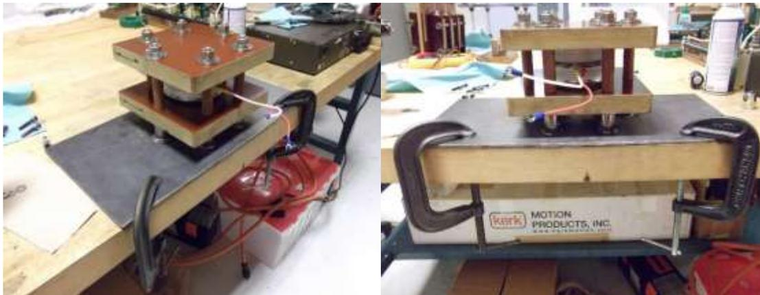
Figure 4-11. Flat-Plate Thruster switch module construction. a) Isometric view. b) Front view.
