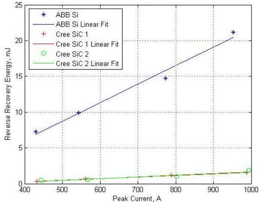
Figure 5-10. Reverse recovery energy loss as a function of peak current for the three diodes tested.
