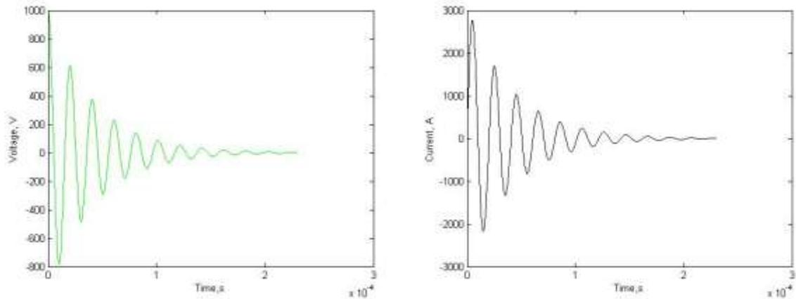
Figure 3-3. Simulated current and voltage waveforms for the circuit in Figure 3-1. The estimated ringing frequency is 50 kHz. a) Capacitor voltage. b) Loop current.
