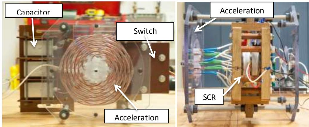
Figure 4-16. Switch module connection- physical view. a) Front view of assembled FPT. b) Side view of assembled thruster showing switch module position.
