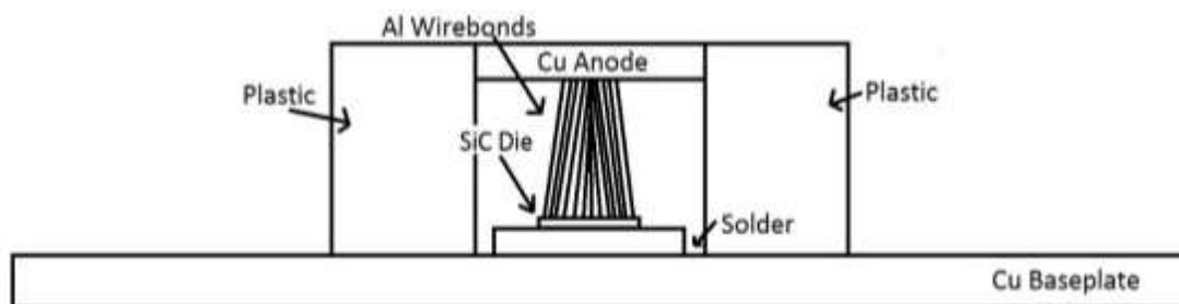
Figure 2-3. Schematic representation of Cree SiC diode cross-section.
