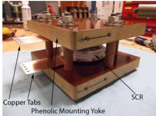
Figure 4-13. Flat-Plate Thruster Dynex configuration switch module.
