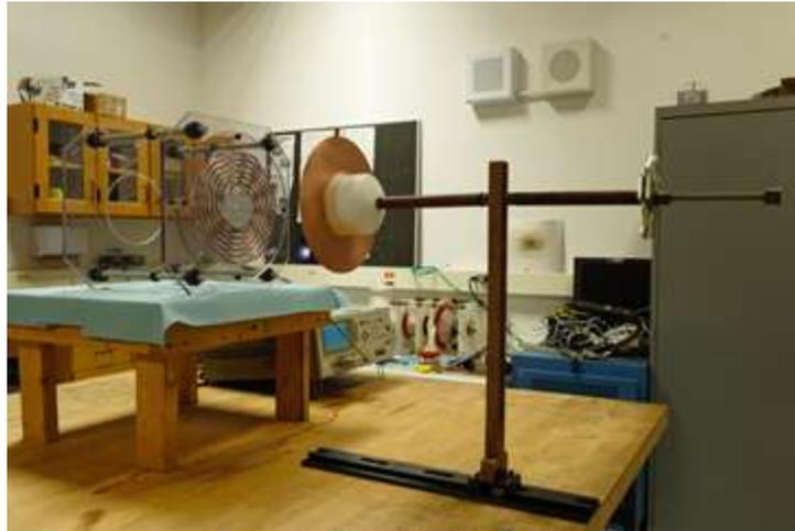
Figure 4-4. Inductance Measurement setup. The copper disk simulates the plasma current sheet, and inductance measurements are taken to determine the coil self-inductance and electromagnetic decoupling length of the manufactured FPT acceleration coil.
