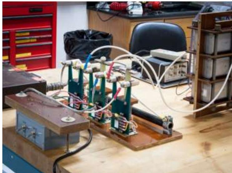
Figure 4-15. Charge/dump control circuit. The relays are opened and closed via manual switches mounted on the grey controller box. These are manipulated using a 45 cm long phenolic rod.
