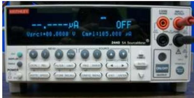
Figure 2-8. Keithley Model 2440 SourceMeter front panel.
