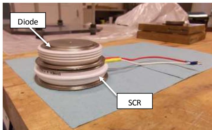
Figure 4-9. Dynex switching components. The Dynex FRD is shown in series with the Dynex SCR.
