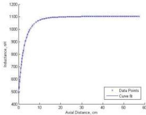
Figure 4-7. Inductance Measurement Data. The measured effective coil inductance is observed to asymptote to a value of approximately 1102 nH beyond a distance of approximately 6 cm.
