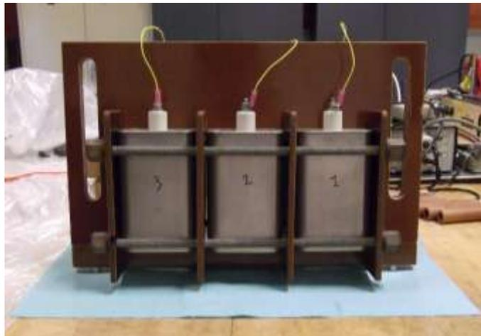
Figure 4-8. Flat-Plate Thruster capacitor bank.
