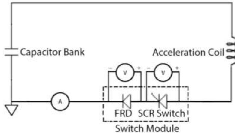
Figure 4-14. Bench-top testing circuit topology. The switch module configuration is varied.
