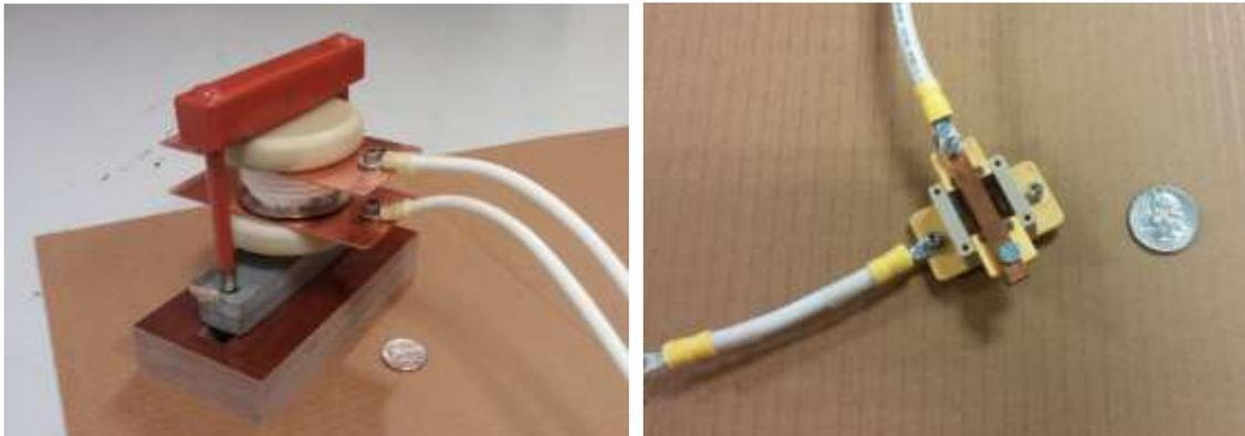
Figure 4-10. Diodes for FPT testing. a) 5.8 kV SiC PiN diode from Cree, Inc. b) 5.5 kV Si fast diode from ABB.
