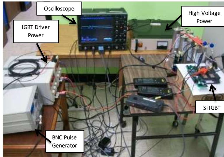
Figure 2-12. Photograph of medium current static characterization test laboratory setup.
