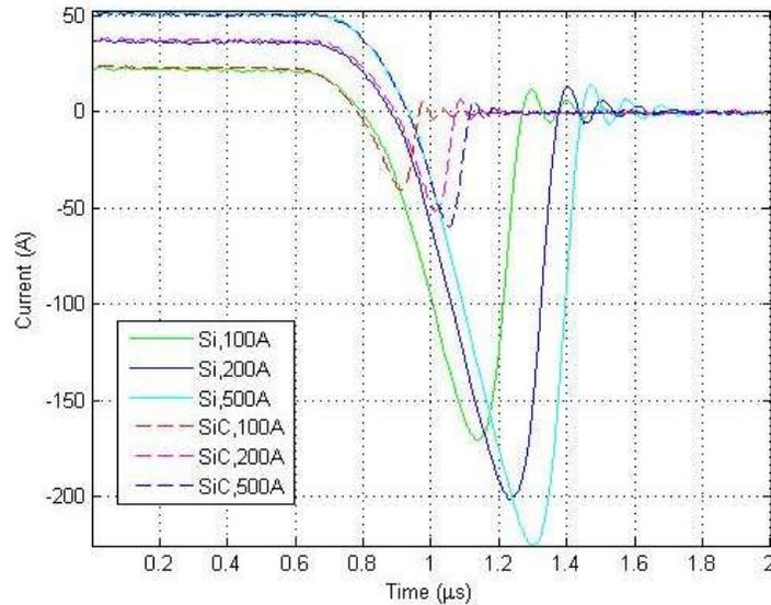
Figure 2-20. Comparison of reverse recovery waveforms for the Si and SiC diodes at varying diode forward current and 25°C.
