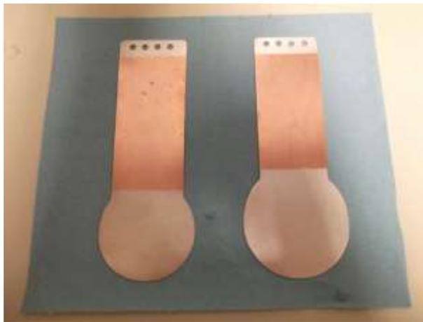
Figure 4-12. Switch module connector tabs. Silver areas were treated with Cool Amp Conducto-Lube.
