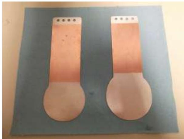
Figure 4-12. Switch module connector tabs. Silver areas were treated with Cool Amp Conducto-Lube.
