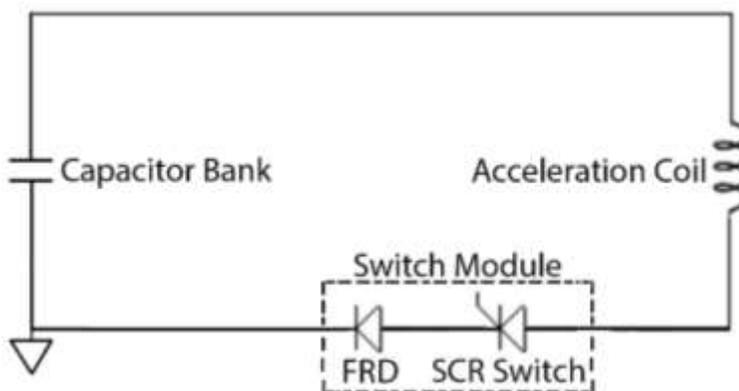
Figure 1-4. Diode-clamped IPPT circuit topology.
