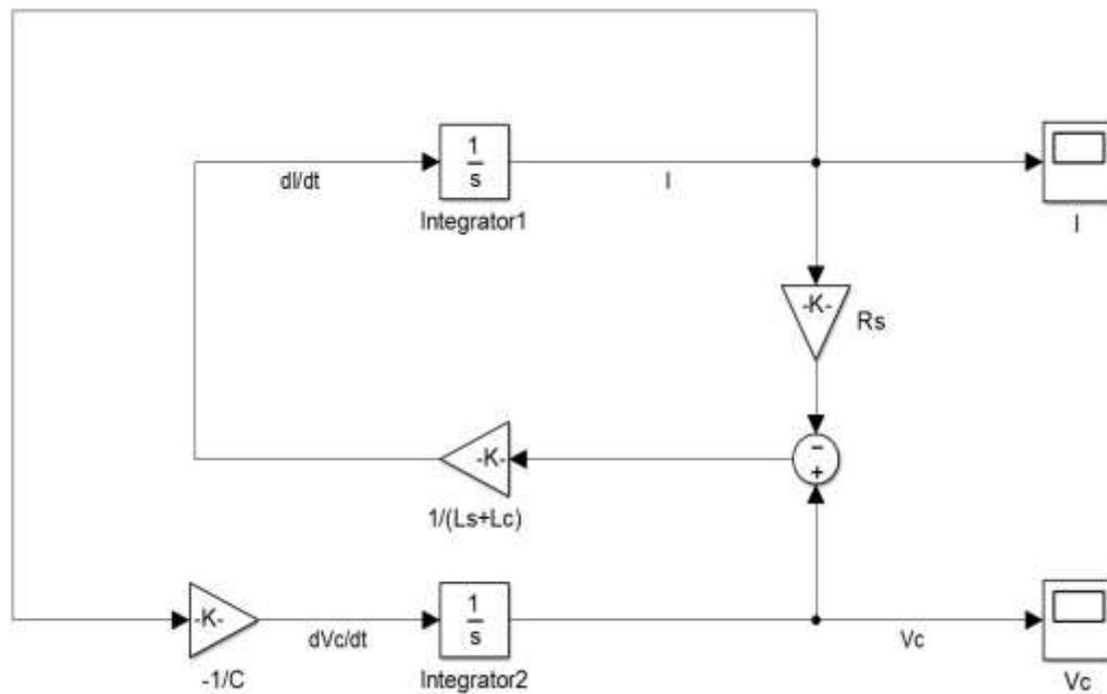
Figure 3-2. Simulink<sup>®</sup> model of RLC IPPT electric circuit model as coupled first order ODE.
