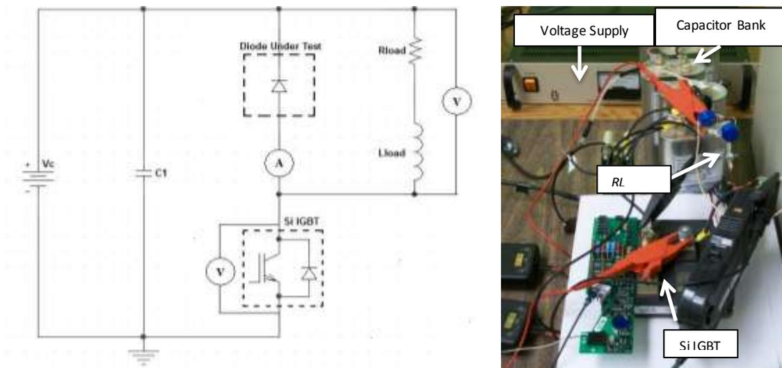
Figure 2-11. Circuit and setup used for medium current static characterization. a) Schematic representation of circuit. b) Physical setup of the circuit.
