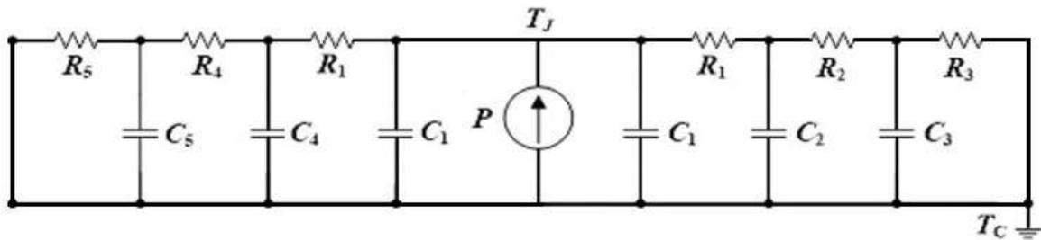
Figure 2-5. Cauer equivalent RC thermal network model for prototype Cree SiC diode.
