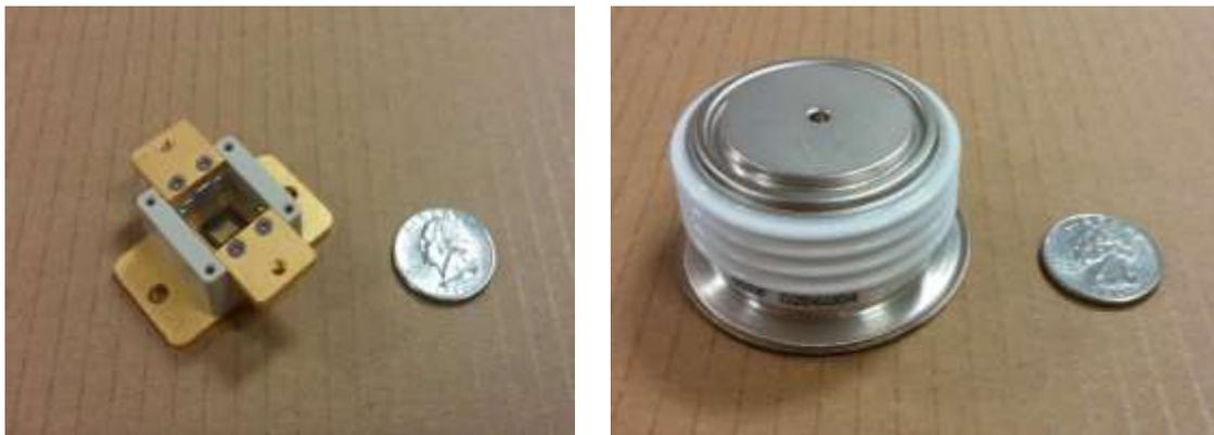
Figure 2-1. Si and SiC test diodes. a) 5.8 kV SiC PiN diode from Cree, Inc. b) 5.5 kV Si fast diode from ABB Semiconductors.
