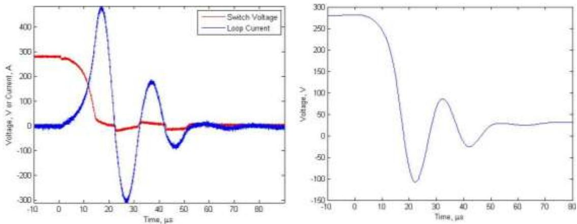
Figure 5-3. Baseline switching waveform. a) The measured switch voltage and loop current waveforms for the no-diode configuration. b) The capacitor voltage calculated from Equation 5-2. The SCR is observed to self-trigger after the gate pulse has been removed.
