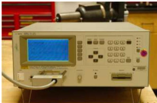
Figure 4-6. Agilent RLC Meter. An Agilent 4285A Precision RLC meter was used to collect inductance measurements of the FPT acceleration coil.
