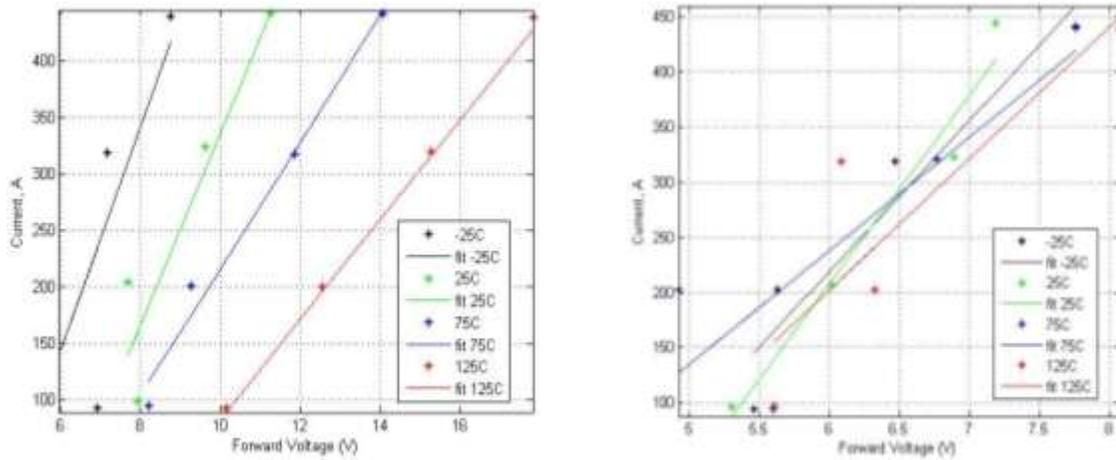
Figure 2-13. Medium current V-I characteristic data with trend lines for a) Si diode and b) SiC diode.
