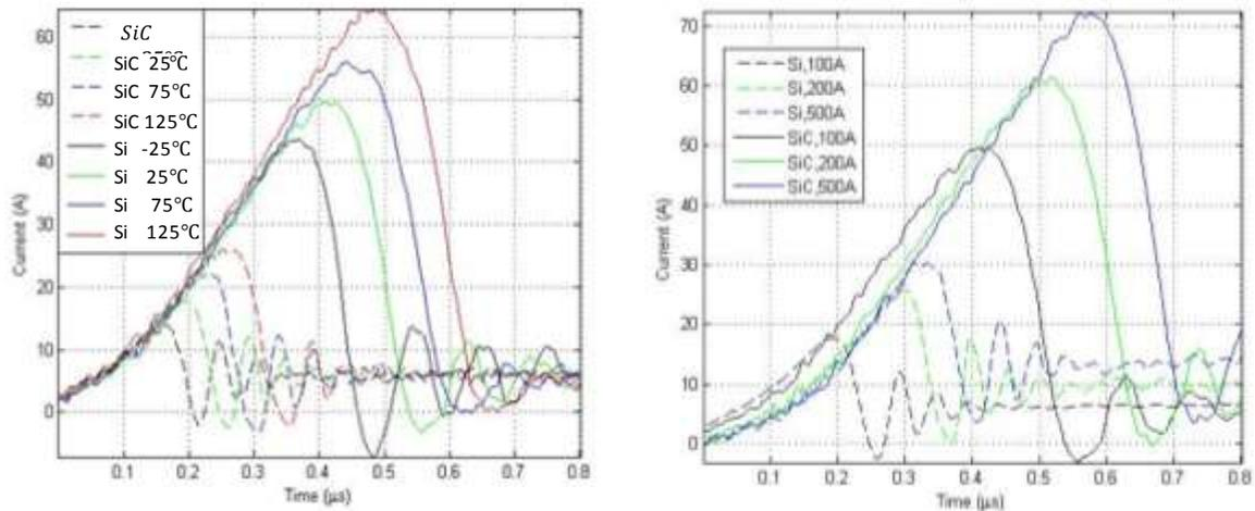
Figure 2-22. IGBT current spike waveform measured at diode turn off for a) Si and SiC diodes at  $I_L = 100\text{ A}$  and varying temperatures. b) Si and SiC diodes at  $25^\circ\text{C}$  and varying load current.
