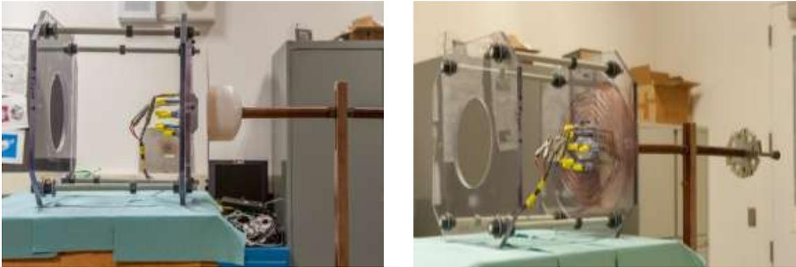
Figure 4-5. Acceleration coil connections. a) Back isometric view. b) Side view.
