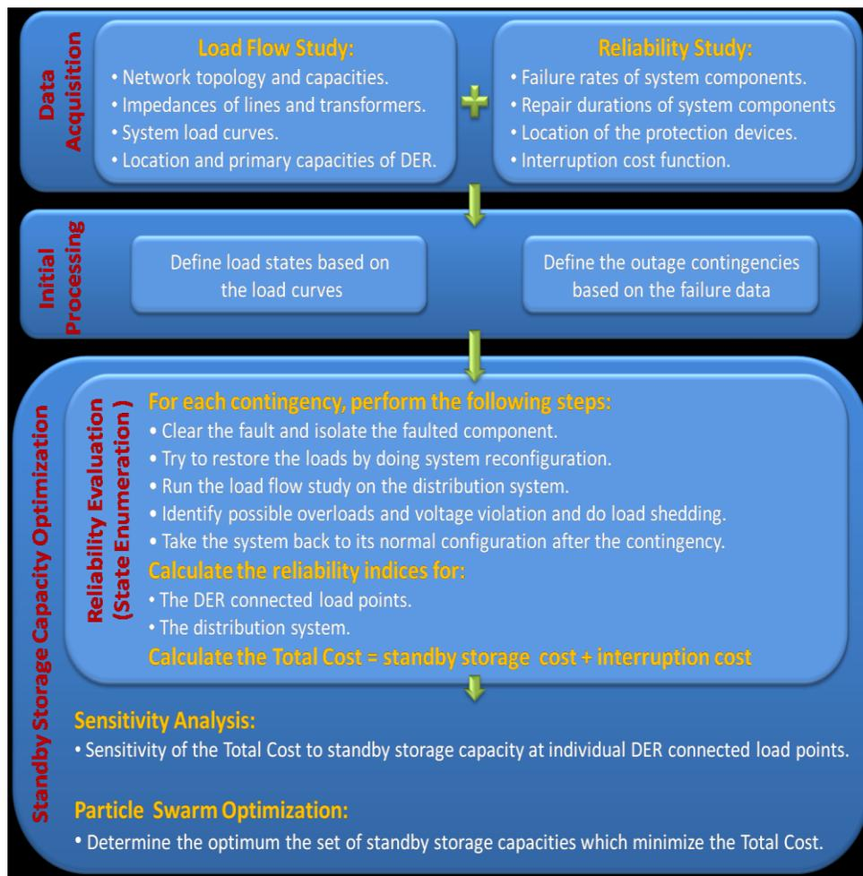
**Figure 4.15 Flowchart of the study to determine the optimum storage capacity**
