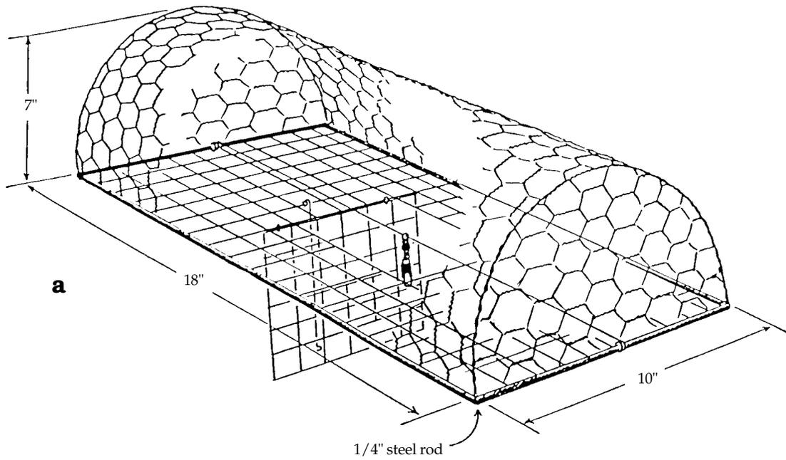
Fig. 5. (a) Big bal-chatri trap ready for nooses (door is open). (b) Method of attaching nooses.
