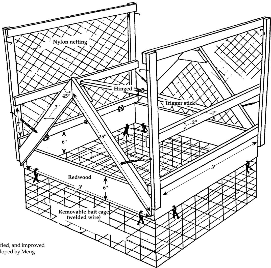
Fig. 4. The redesigned, modified, and improved Swedish goshawk trap developed by Meng (1971).
