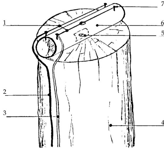
Fig. 3. The electric pole shocker.
