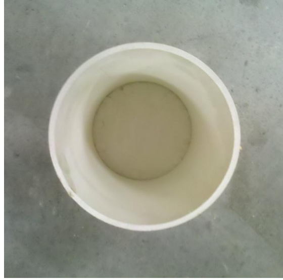
Figure 4.1 100×160 mm PVC Cylinder Mold
