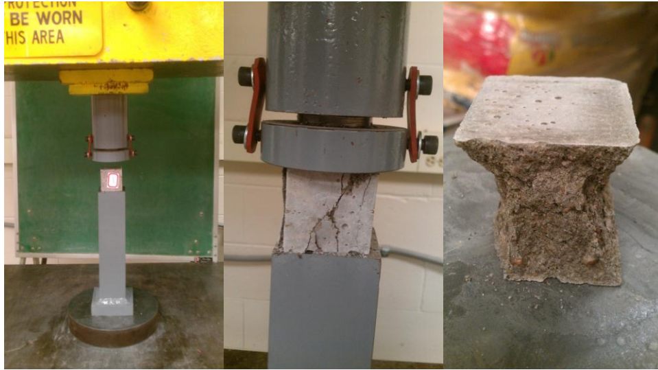
Figure 3.3 Testing of a Mortar Cube with 4% Aerogels
