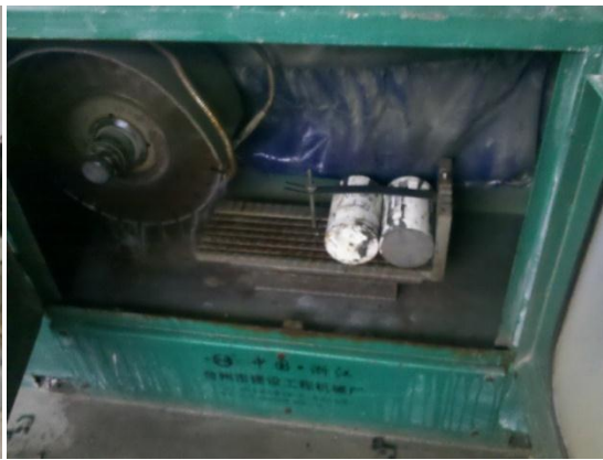
Figure 4.2 HQM Concrete Saw Cutting Machine
