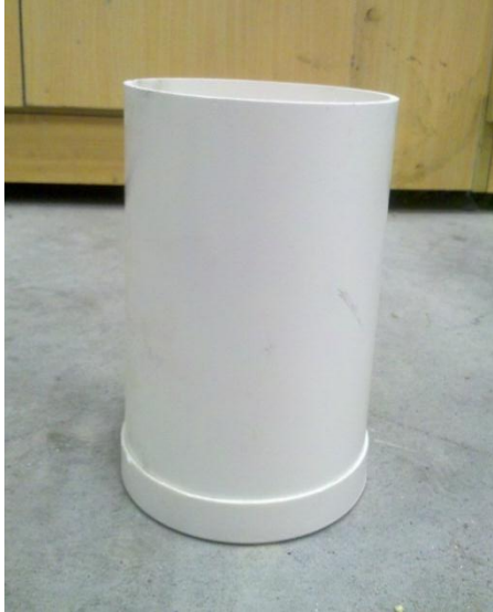
Figure 4.1 100×160 mm PVC Cylinder Mold
