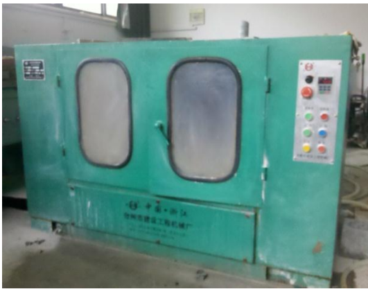
Figure 4.2 HQM Concrete Saw Cutting Machine
