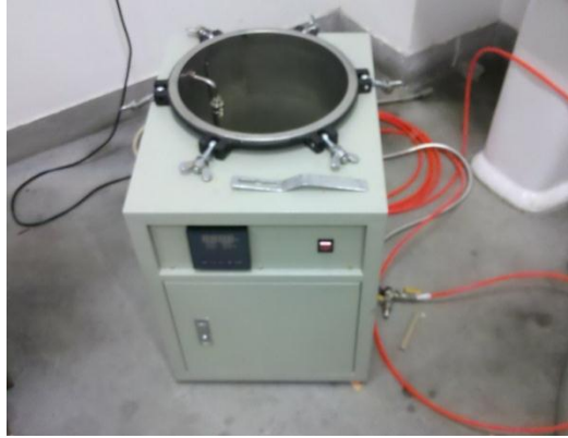
Figure 4.4 Intelligent Vacuum Saturated Concrete Machine
