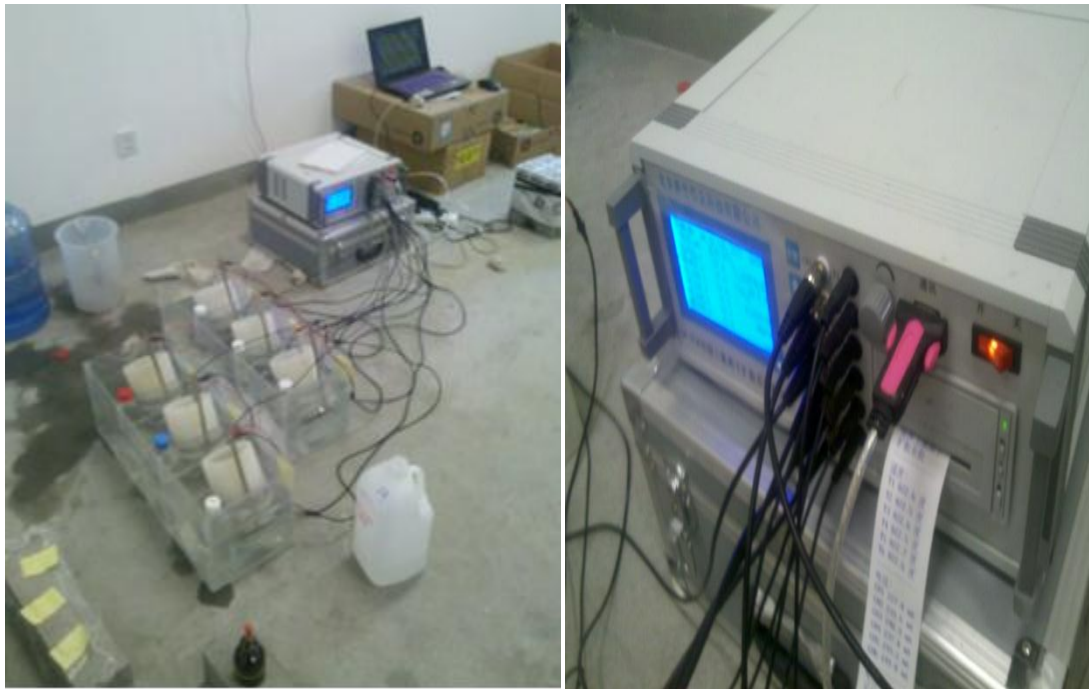
Figure 4.5 Chloride Penetration Test Setup
