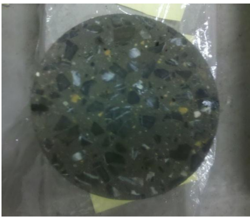
Figure 4.3 Sliced Sample with a Dimension of 100 ± 1 mm Diameter and 50 ± 2 mm Thickness
