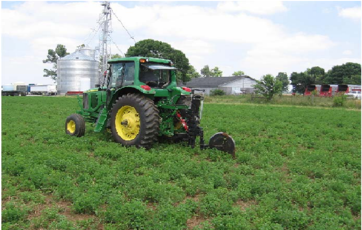
Figure2. Coulter penetrometer during the field test at UKARC
