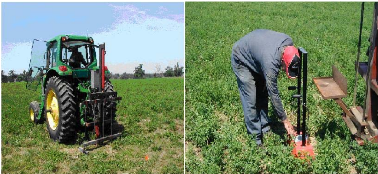
Figure3. Multi-probe soil cone penetrometer (left) and digital nuclear moisture density testing machine (right)
