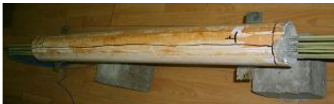
a) Setup of GFRP-coated optical fibers
