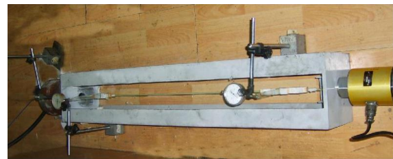
b) Steel frame for loading
