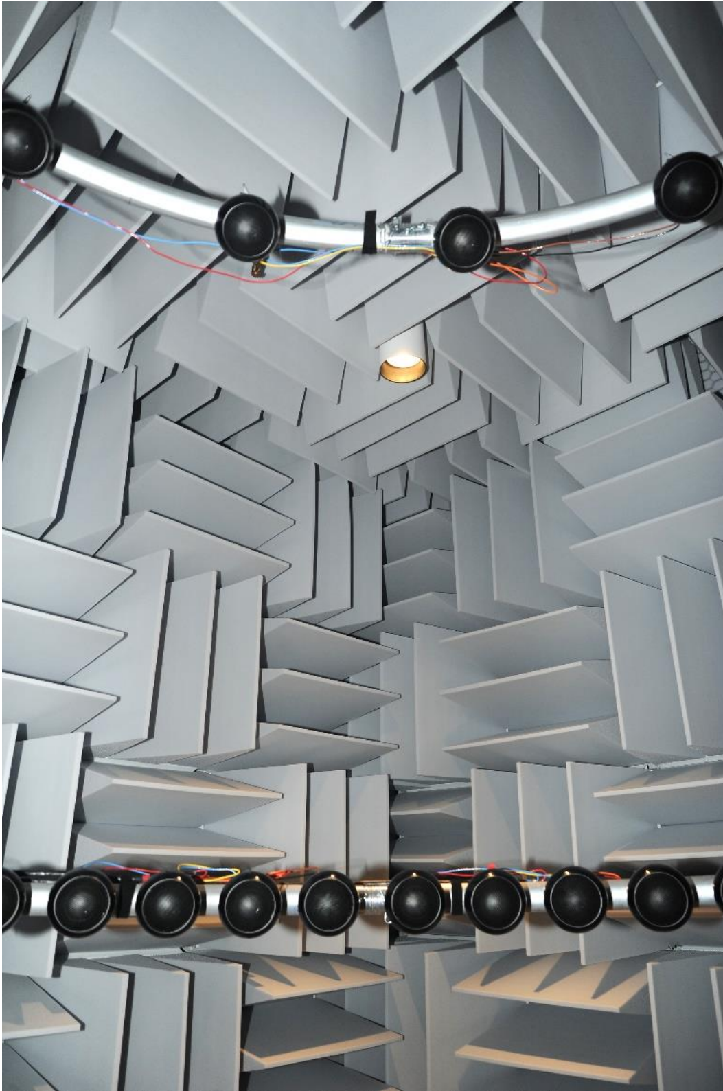
Figure 3.6: Example of strongly absorptive surfaces; photograph of the Boys Town National Research Hospital anechoic chamber courtesy of the BTNRH Marketing Department
