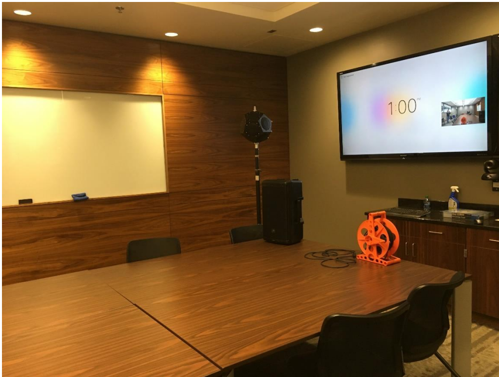
Figure 3.2: Photograph of the omnidirectional loudspeaker used for room impulse response measurements in a common talker position in Peter Kiewit Institute room 150 (a conference room); note that the other loudspeaker pictured was relevant to procedures used before the adoption of the convolution method (see Appendix B).
