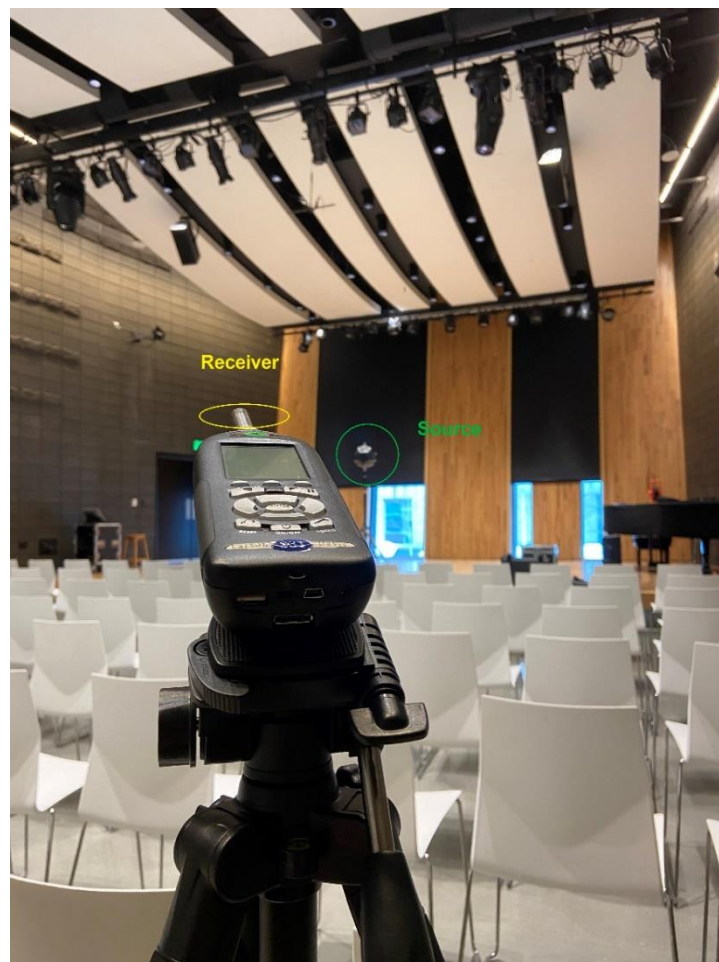
Figure 3.1: Photograph of a Larson-Davis Model 831 sound level meter being used in the Strauss Performing Arts Center recital hall (with omnidirectional loudspeaker just left of center in the background)
