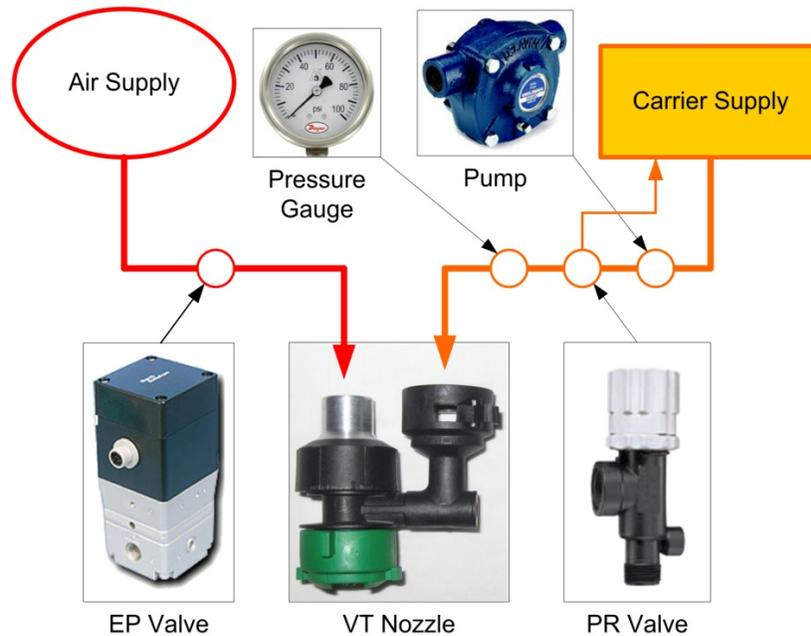
Figure 4. Test system diagram for control of carrier delivery and diaphragm air pressure to the VT nozzle during testing.
