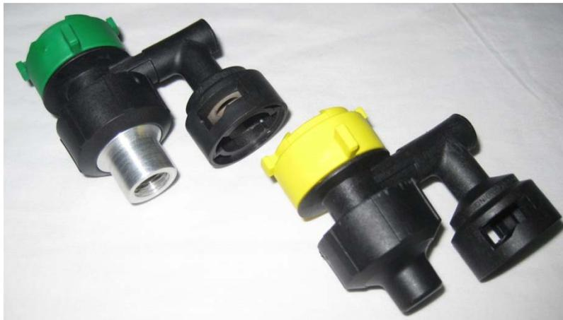
Figure 2. Original VT nozzle configuration (right) with the VT nozzle modified for testing (left).
