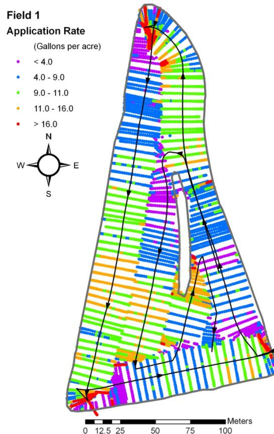
Figure 1. Estimated field coverage application rates (target rate 10 gal/ac).
