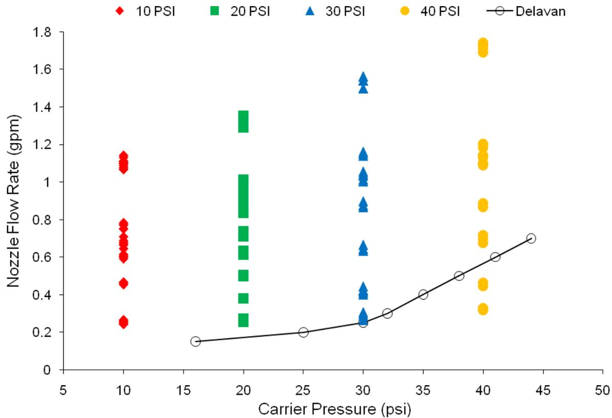
Figure 6. Nozzle flow rate versus carrier pressure as air diaphragm air pressure was adjusted (calibration curve for VT nozzle also included).
