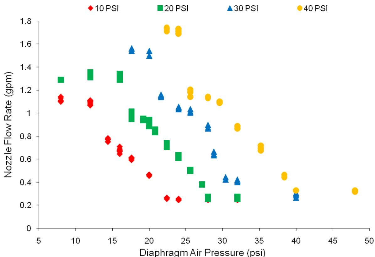
Figure 5. Nozzle flow rate versus diaphragm air pressure for 10, 20, 30, and 40 psi carrier pressures.
