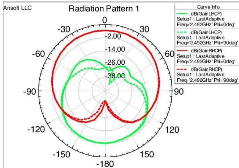
**Figure 3 : Radiation Pattern of a MSA**
