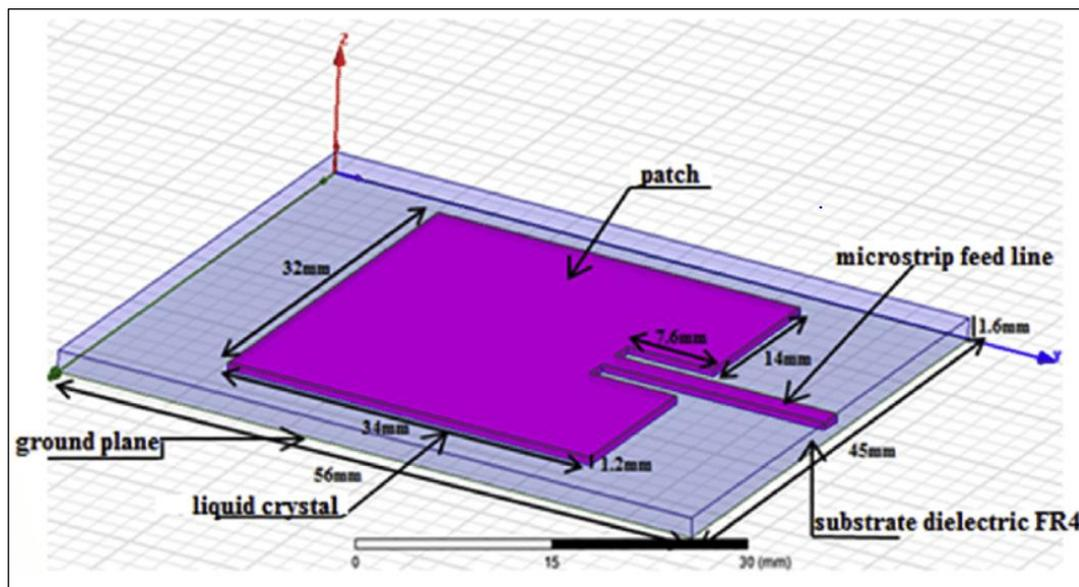
**Figure 2 : A Microstrip Patch Antenna Design using Ansys HFSS**
