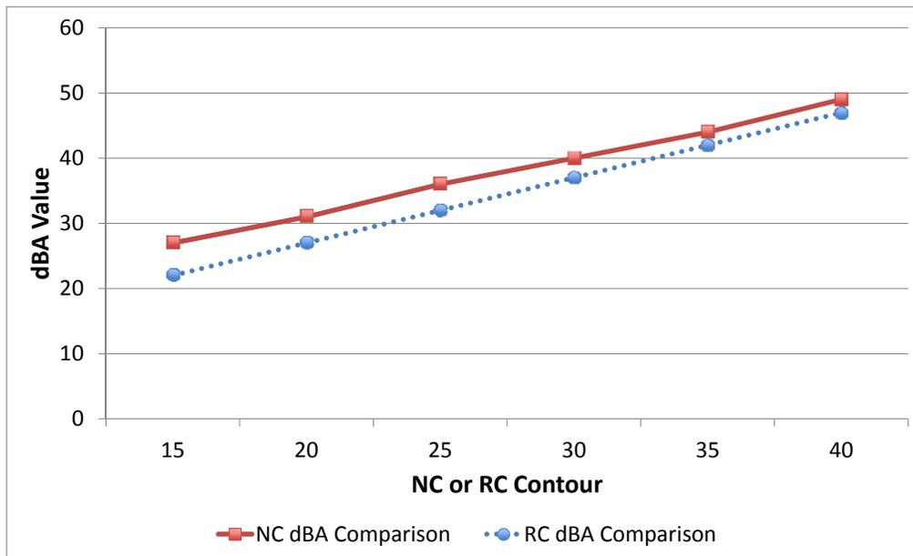
**Figure 1:** Comparison of NC and RC contours to equivalent dBA values
