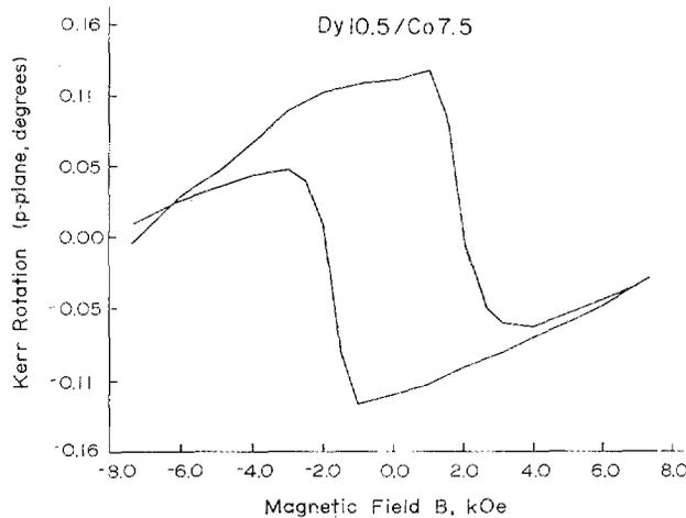
FIG. 2. Hysteresis loop for Dy 10.5/Co 7.5 showing  $p$ -plane Kerr rotation vs applied magnetic field strength. Measurements were taken at a  $60^\circ$  angle of incidence and wavelength at  $6328 \text{ \AA}$ .
