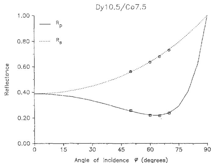
FIG. 1. Reflections vs angle of incidence for Dy 10.5/Co 7.5. Symbols represent measured values and lines represent best-fit calculated values with  $\tilde{n} = 1.28 - j1.78$ . The measurements were taken at a wavelength of 4000 Å.
