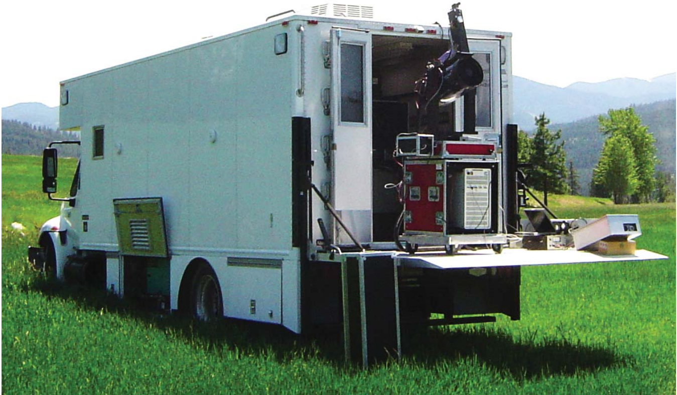
Researchers are using a truck-mounted lidar to study the dynamics of smoke plumes from wildland fires. Credit: V. Kovalev.
