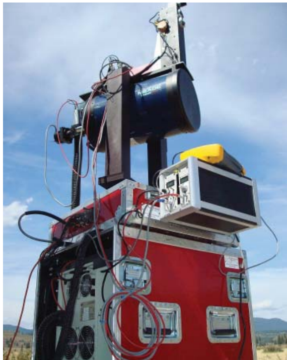
The mobile lidar setup. Credit: V. Kovalev.
