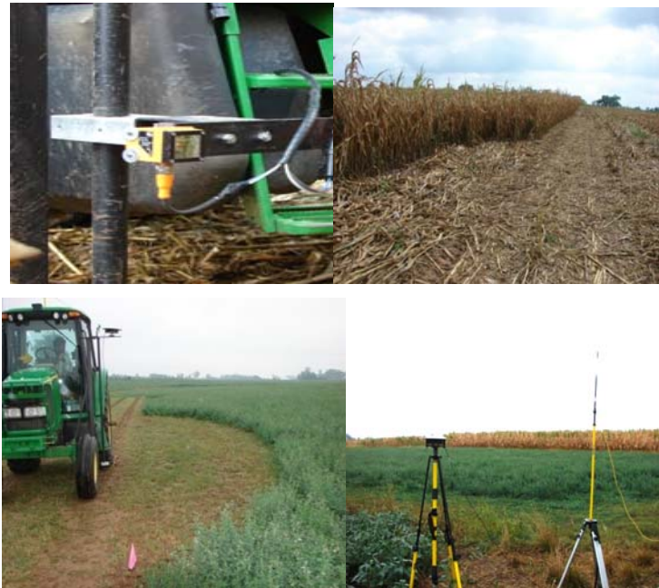
Figure 3. Sensor setup (top-left); Corn cut-crop edge (top-right); Tractor/sensor path in alfalfa cut-crop edge (bottom-left); RTK-Base station (bottom-right)
