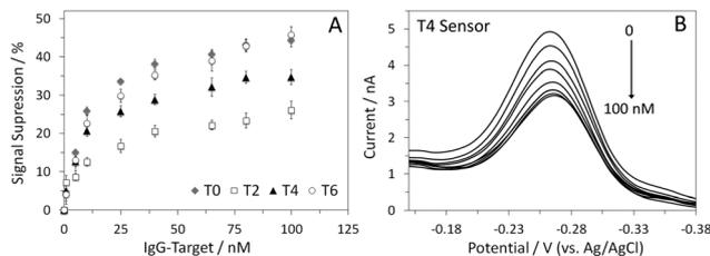
Fig. 2 Dose response curves of the four sensors obtained in Phys2 (A). The  $K_d$  was 7, 12, 8, and 10 nM for the **T0**, **T2**, **T4**, and **T6** sensors, respectively. Also shown are AC voltammograms recorded for the **T4** sensor in the presence of 1, 5, 10, 25, 40, 65, 80, and 100 nM IgG-target (B).
