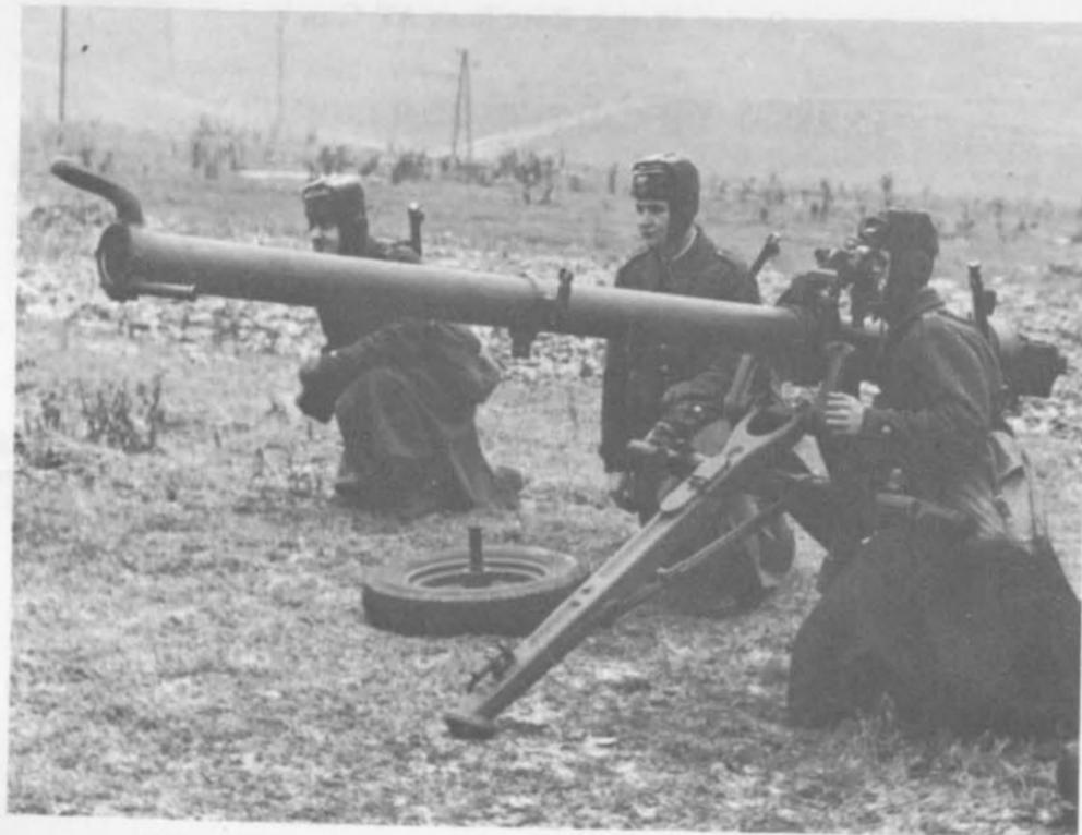
SOVIET 107-MM RECOILLESS ANTITANK GUN, B-11.
