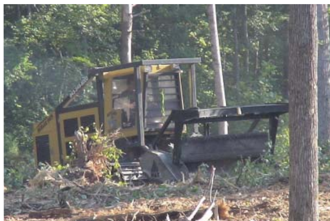
Kodiak Kutter® felled standing trees and chopped woody debris. Credit: USDA Forest Service.
