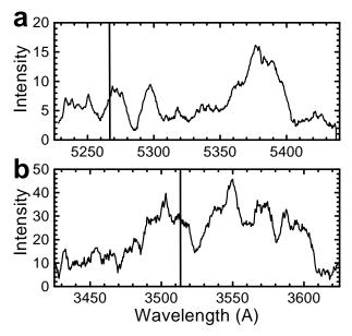
FIG. 4. Spectra of the (a) 2nd and (b) 3rd harmonics at  $\theta=90^\circ$ ,  $\phi=50^\circ$  for 0.8-J pulse energy and  $6.2\times10^{19}\text{-cm}^{-3}$  electron density. Vertical lines indicate the wavelengths of the unshifted 2nd and 3rd harmonics. The intensities are ploted in arbitrary units. The spectra do not change with variation of  $\phi$  at any specific  $\theta$ , so the angular distributions measured are not affected by the choice of filter bandwidth.
