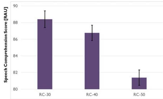
**Figure 5.** Marginal means of speech comprehension performance in Study 1, averaged across all RT scenarios for each BNL condition. Error bars indicate one standard error.
