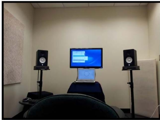
**Figure 1.** View from listener's position in the Nebraska Acoustics Testing Chamber.
