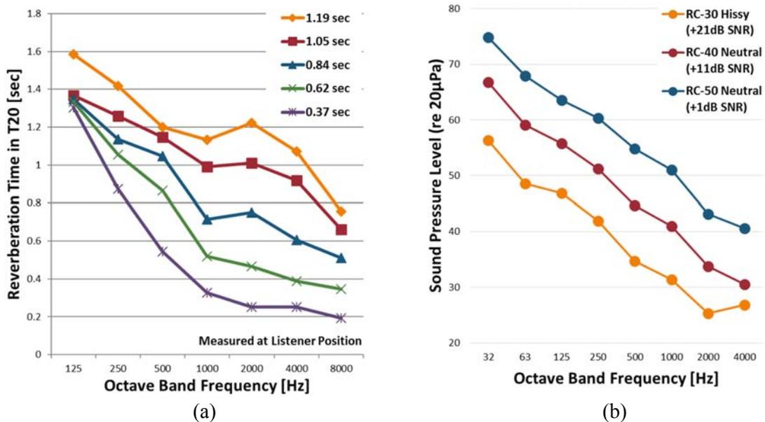
**Figure 2.** (a) Measured reverberation times (mid-frequency averages shown in legend) and (b) measured background noise levels (RC and signal-to-noise ratio values shown in legend) across octave bands at the listener position for the five RT and three BNL conditions.
