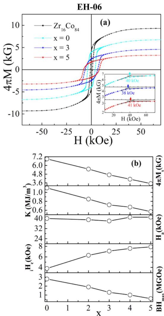
Fig. 2. Hysteresis loops of nanocrystalline  $Zr_{16}Co_{84}$  and  $Zr_{16}Co_{78-x}Mo_xSi_3B_3$  ( $x = 0, 3, 5$ ) (the inset showing saturation fields for  $x = 0, 3, 5$ ) (a) and deduced magnetic properties as a function of  $x$  (b).
