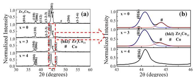
Fig. 1. XRD patterns of nanocrystalline  $Zr_{16}Co_{84}$  and  $Zr_{16}Co_{78-x}Mo_xSi_3B_3$  ( $x = 0, 3, 4$ ).
