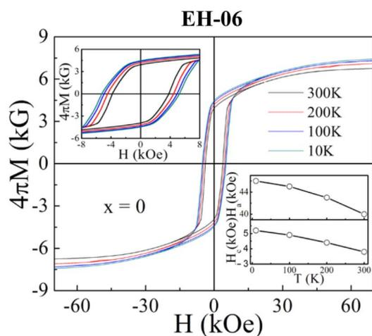
Fig. 3. Hysteresis loops at various temperature of nanocrystalline  $Zr_{16}Co_{78-x}Mo_xSi_3B_3$  ( $x = 0$ ). The upper left inset showing the enlarged part of hysteresis loops. The lower right inset showing temperature dependence of magnetocrystalline anisotropy parameter, anisotropy field, and coercive force.
