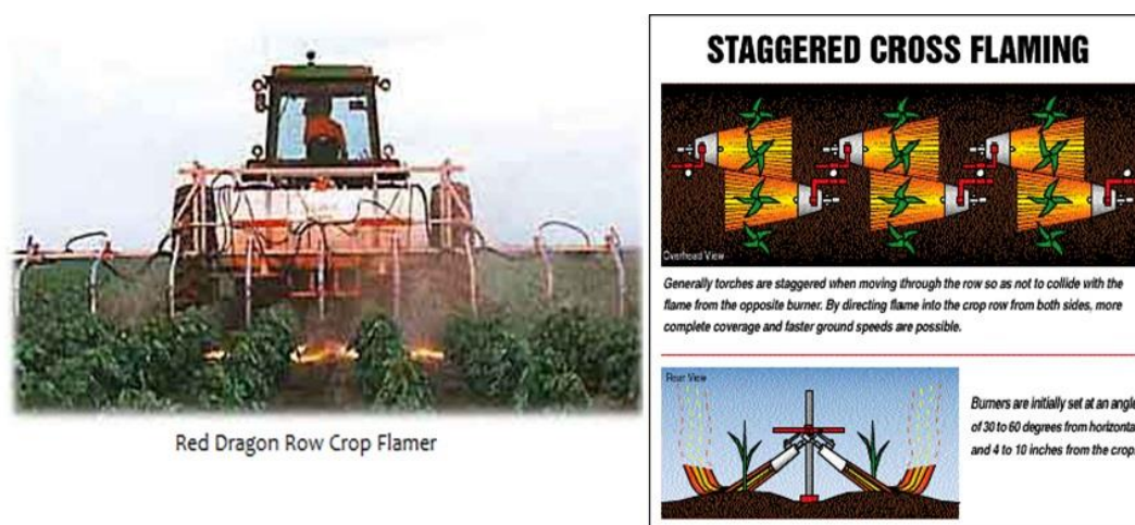
Figure 1.1. Flame-weeding unit performing cross flaming treatments as recommended by Flame Engineering of LaCrosse, KS
