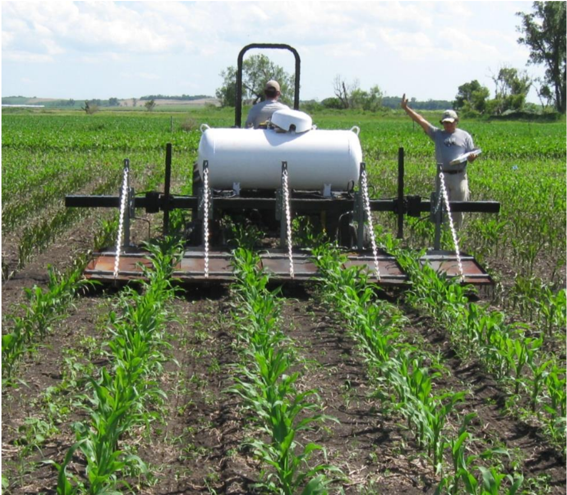
Figure 5.1. The 4-row flamer developed at the University of Nebraska performing parallel-hooded flaming (broadcast flaming) treatments in maize at six leaf–seven leaf stage. In the broadcast setup, eight torches were mounted 38 cm apart and positioned parallel to the crop row (19 cm away from each side) at 20 cm above the soil surface and angled back at 30°. Such setup provided a complete coverage of 76 cm of the inter-row space with a uniform distribution of flame and heat over the land area, and to all four rows in the plot (broadcast flaming treatment). The 4-row full flaming unit had four specially designed 1.2 m long hoods that confined the heat close to the soil surface and subsequently increase the exposure of weed to the heat. Each hood was positioned over the intra-row space and covered two torches
