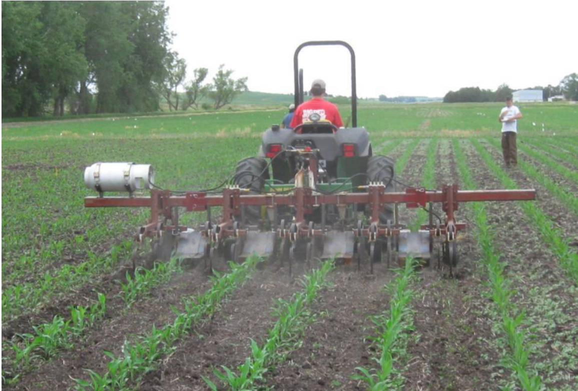
Figure 5.3. The 4-row flamer-cultivator developed at the University of Nebraska performing flaming and cultivation treatments in maize at three leaf–four leaf stage. The flamer-cultivator was built by modifying Noble Row-Runner cultivator that originally had five sweeps per gang. Two edge sweeps on each of the four gangs were replaced by 60 cm long hoods, leaving three middle sweeps to perform inter-row cultivation. Each half of the hood covered one cylindrical torch angled back at 30^\circ and mounted 15 cm away from the crop row and parallel to the slope of the hood. This setup provided 50 cm of inter-row cultivation and 30 cm of intra-row banded flaming, with 4 cm overlap between the two operations to ensure the complete (76 cm) row coverage
