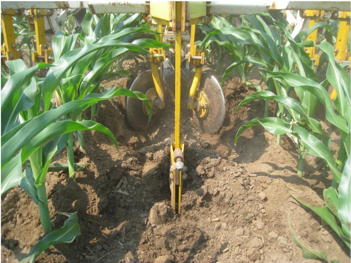
Figure 5.4. Aggressive cultivation treatment in maize at six leaf–seven leaf stage with Buffalo type cultivator. The term “aggressive cultivation” describes a cultivation method that allows throwing soil into intra-row space, which creates a small ridge that buried the flamed weeds
