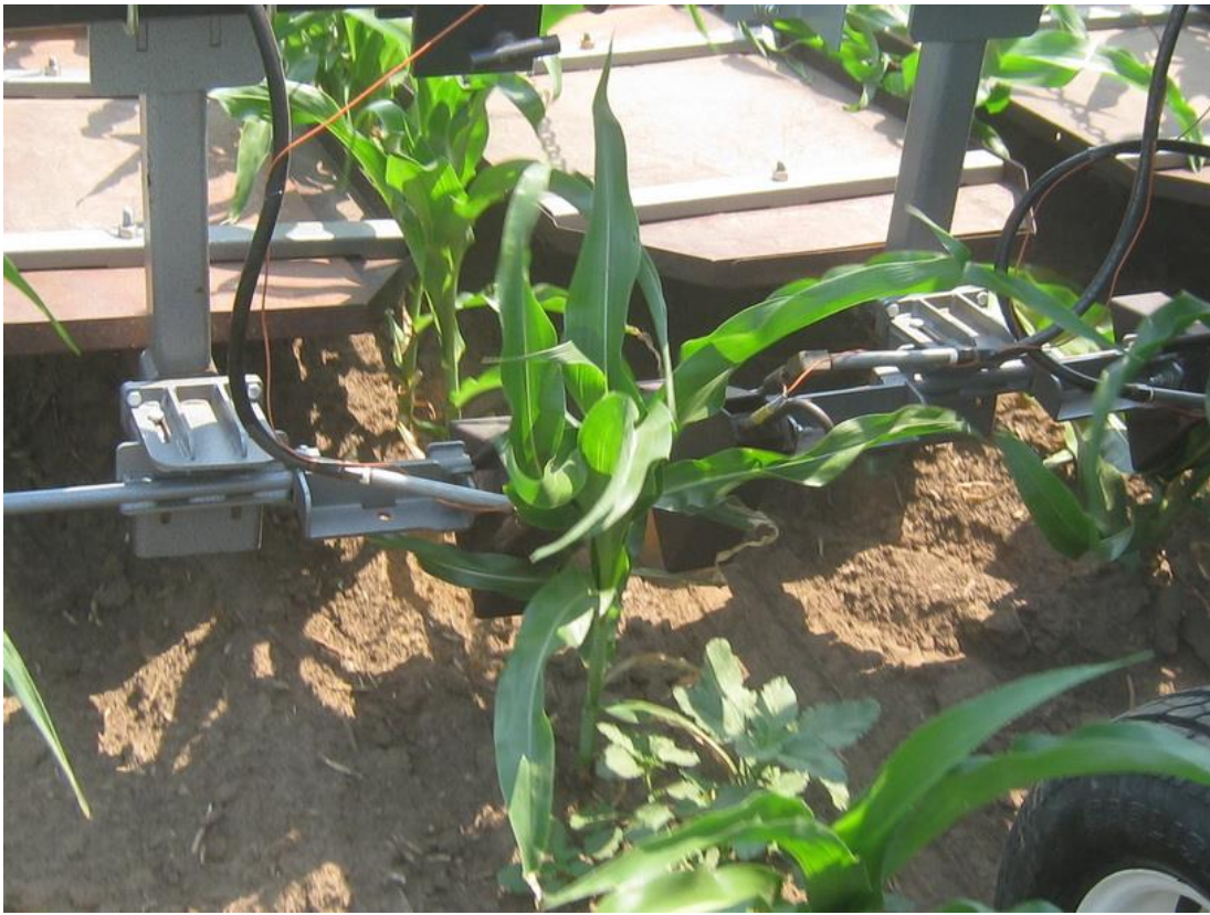
Figure 5.2. The 4-row full flamer developed at the University of Nebraska performing banded flaming treatments in maize at six leaf–seven leaf stage. In the banded setup, torches were positioned at a 30° angle toward crop row so that flame only covered a band of 30 cm of intra-row space (banded flaming treatment)
