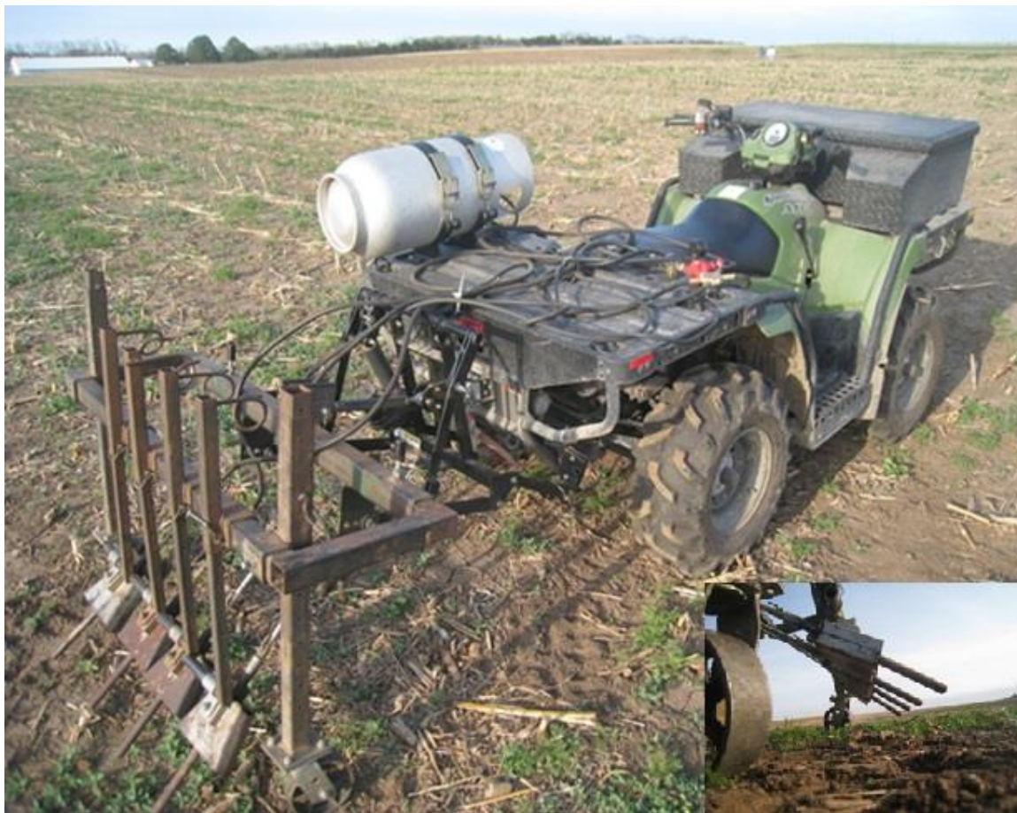
Figure 2.3. Custom built propane flamer mounted on a four-wheeler (all-terrain vehicle) with four burners “LT 2 × 8 Liquid Torch” (Flame Engineering 2007) mounted 30 cm, positioned 20 cm above the soil surface and angled back at 30°
