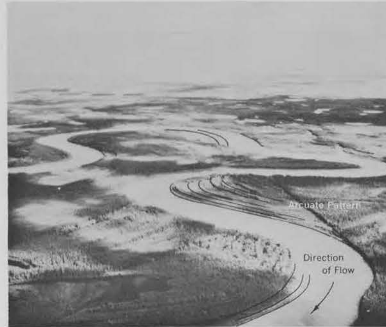
Figure 67: Meandering River The arcuate (bow-like) pattern of the downstream slopes of the meanders indicates the direction of flow.
