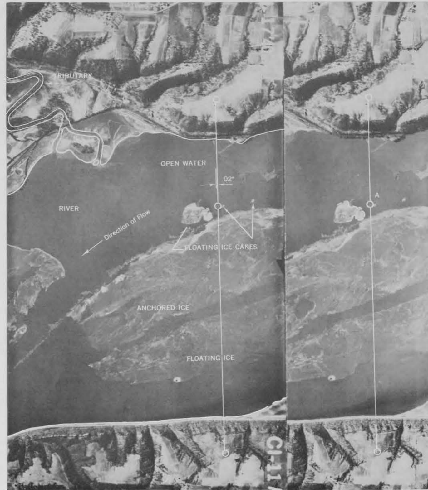
Figure 79: Measuring Surface Velocity Scale 1:20,000
