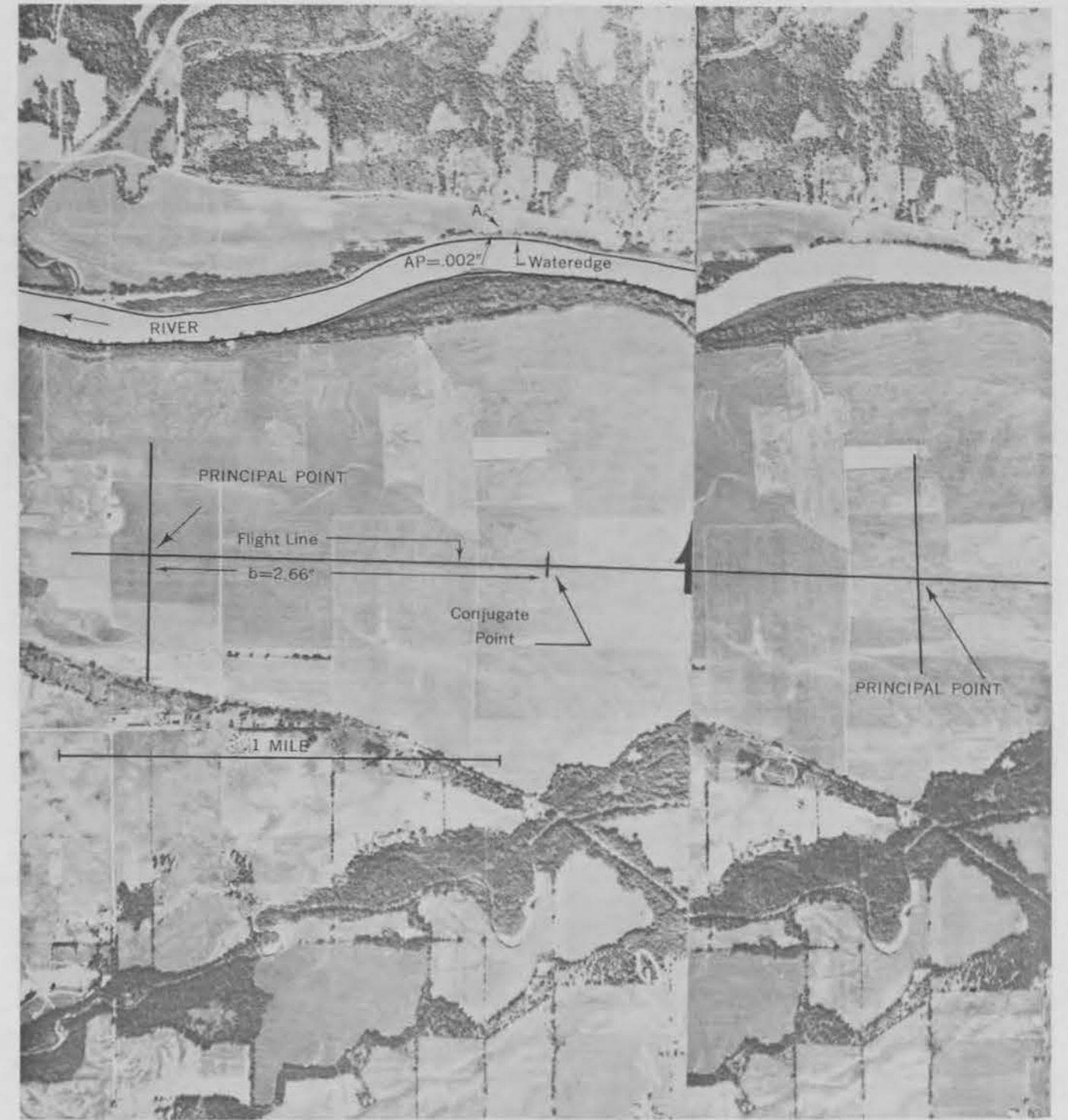
Figure 53: Bank Height Measurement Scale 1:21,000
