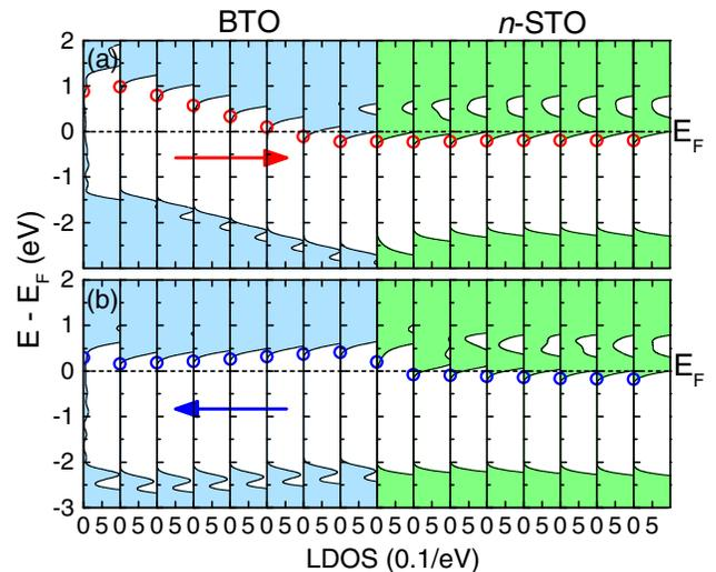
FIG. 2. Local density of states on the TiO<sub>2</sub> layers for ferroelectric polarization (a) into and (b) away from the BaTiO<sub>3</sub>/ $n$ -SrTiO<sub>3</sub> interface. Circles indicate the position of the conduction band minimum, determined from the LDOS as described in the text.
