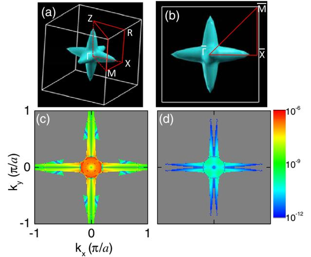
FIG. 4. (a) Fermi surface of *n*-SrTiO<sub>3</sub> and (b) its projection along the *z* direction. (c),(d)  $\mathbf{k}_{\parallel}$ -resolved transmission through the tunnel junction with polarization pointing into (c) and away (d) from *n*-SrTiO<sub>3</sub>.
