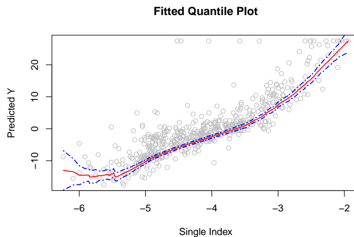
Figure 1: The R output of plot.siqr with estimated 0.25 quantiles and the 95% pointwise confidence bounds.
