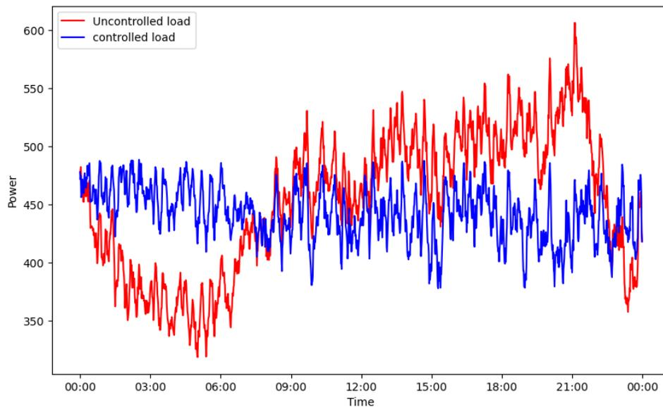
Figure 4-9: Uncontrolled load (red) and controlled load (blue) for peak load optimization only.
