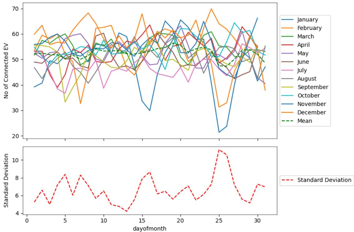
Figure 6-9: Monthly variation in No. of connected EV along with standard deviation.
