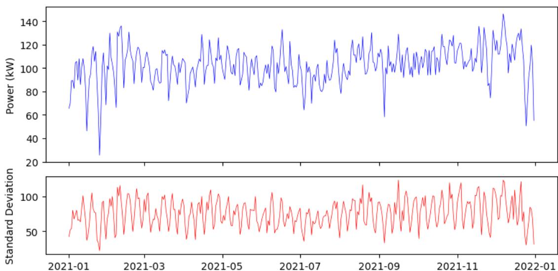
Figure 6-8: Aggregate power consumed during charging along with standard deviation per day.
