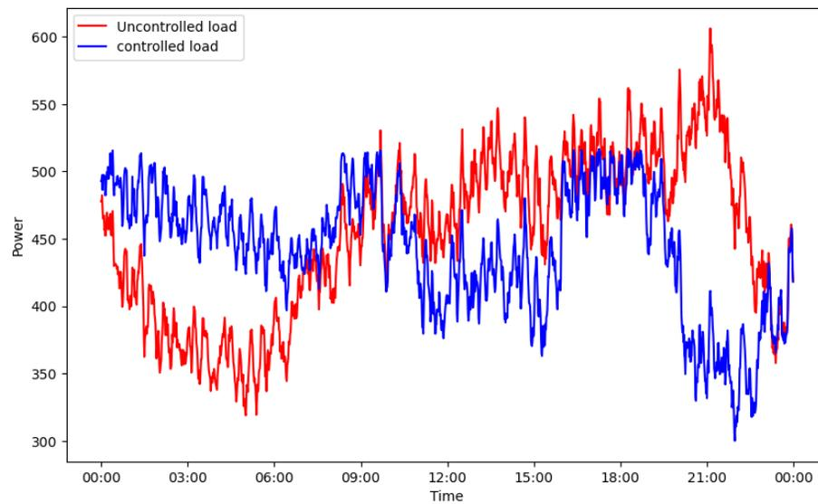
Figure 4-7: Uncontrolled load (red) and controlled load (blue) for equal cost and peak demand weights.
