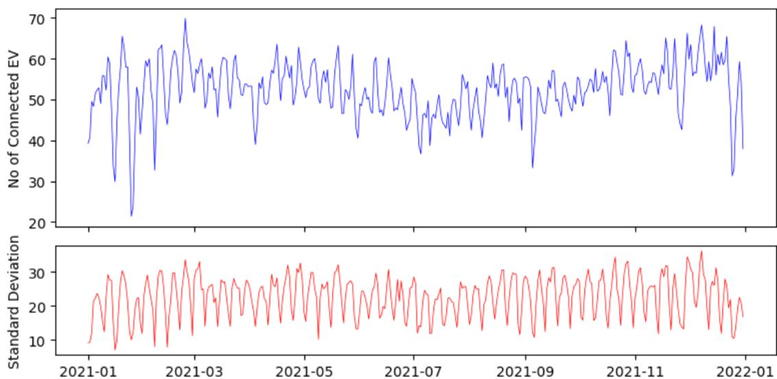
Figure 6-4: Aggregate No. of connected EV along with standard deviation each day.
