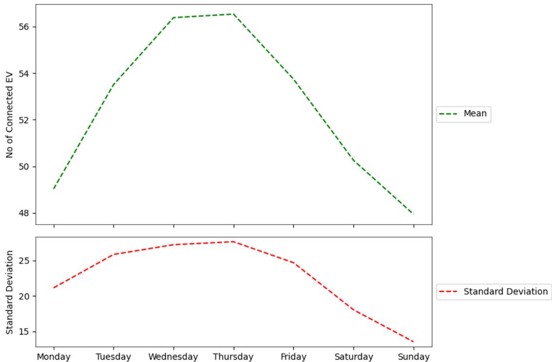
Figure 6-11: Weekly variations in average No. of connected EVs along with standard deviation.
