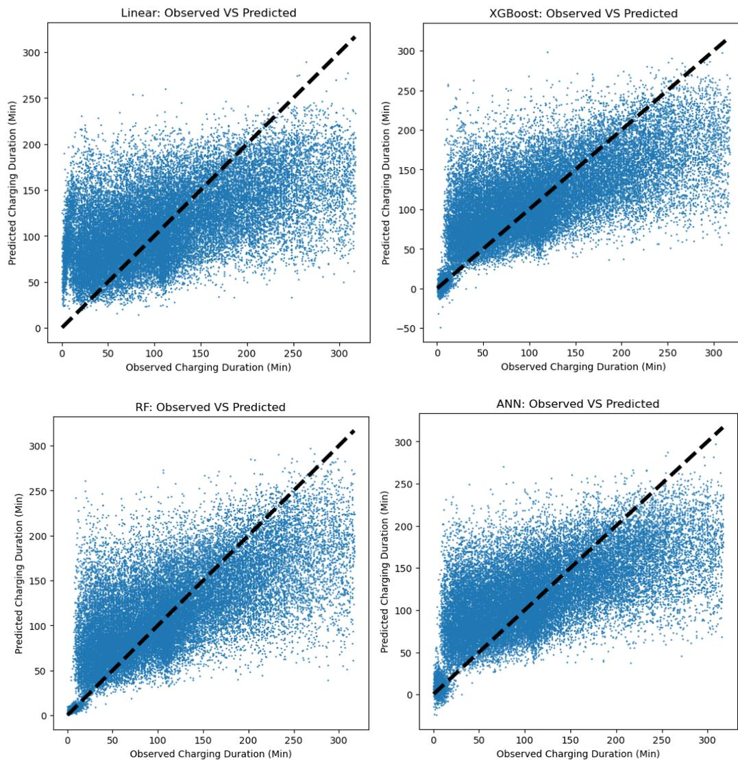
Figure 5-12: Predicted vs. Observed charging duration for each method.
