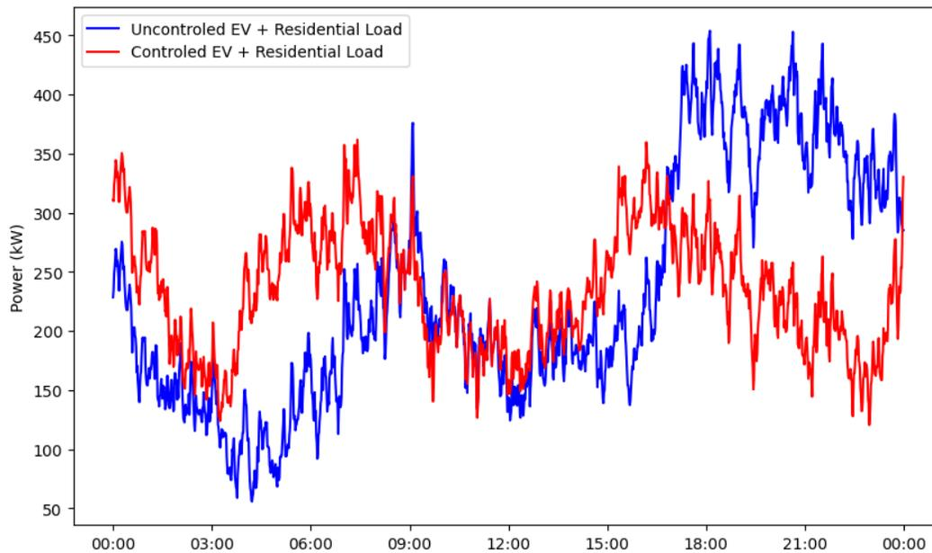
Figure 7-4: Uncontrolled load and controlled load for equal cost and peak demand weights
