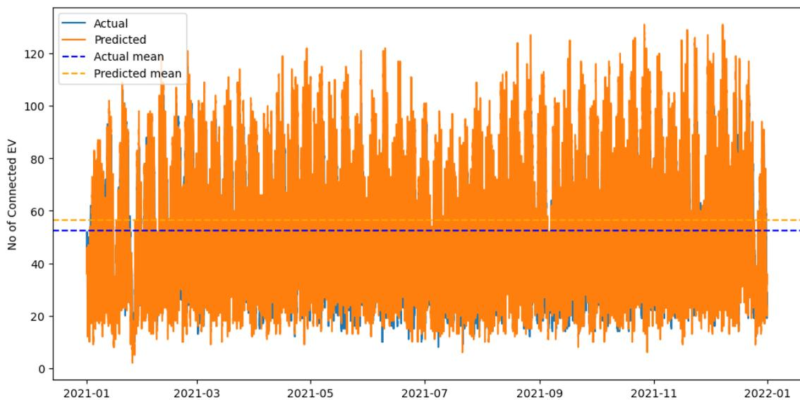
Figure 6-16: Actual vs predicted aggregate No. of EV connected per minute.
