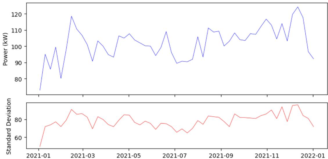
Figure 6-7: Aggregate power consumed during charging along with standard deviation per week.
