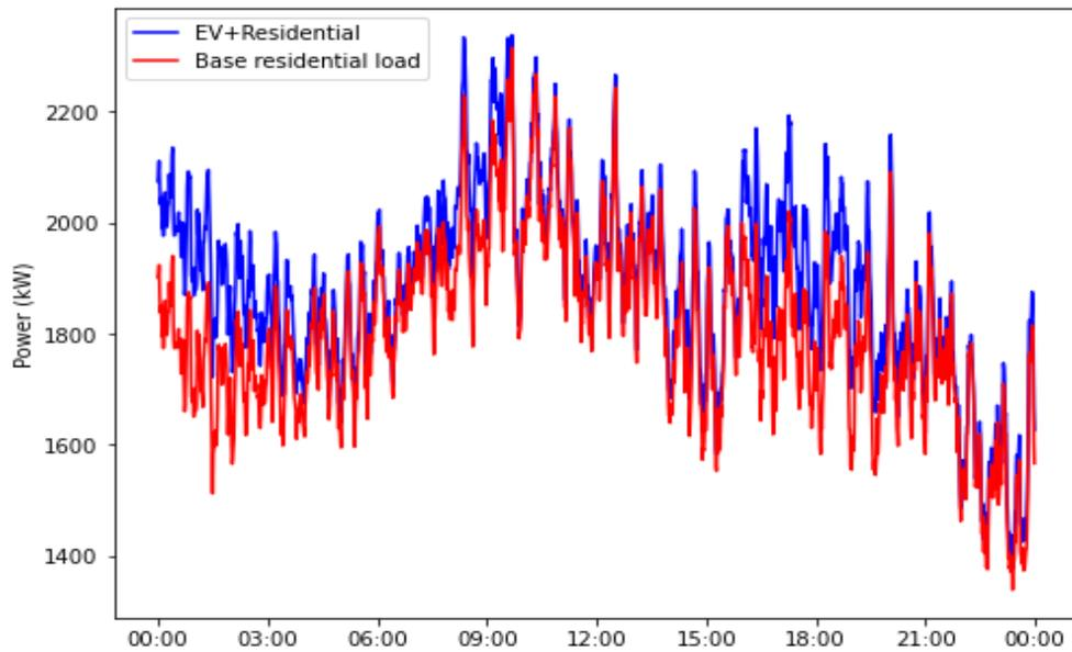
Figure 4-10: Base residential load (red) and total controlled load (blue) for a larger residential system (lower EV penetration) with equal cost and peak demand weights.
