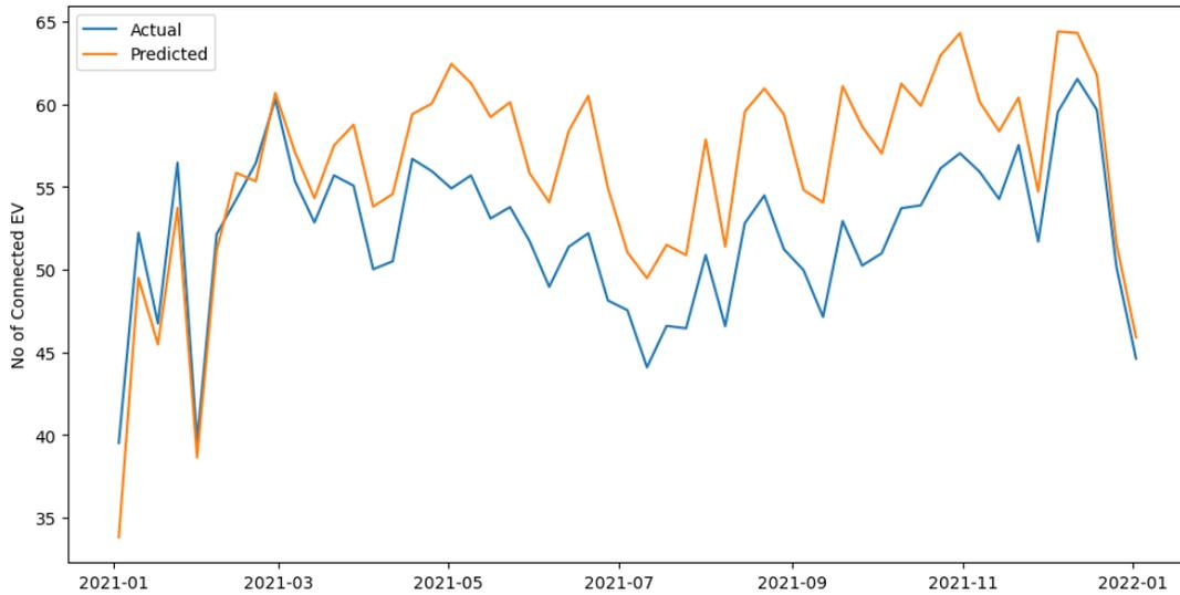
Figure 6-19: Actual vs predicted aggregate No. of EV connected per week.
