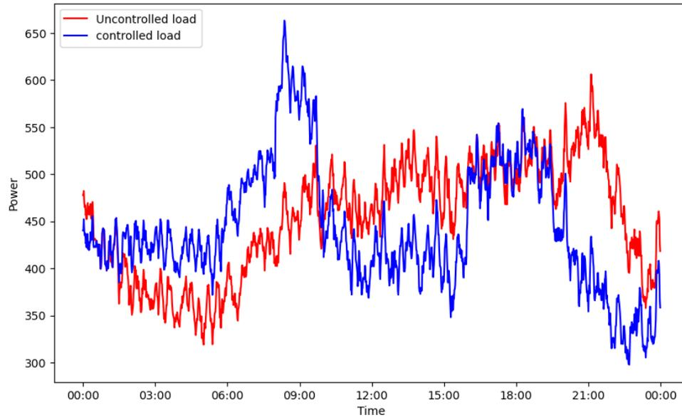
Figure 4-8: Uncontrolled load (red) and controlled load (blue) for cost optimization only.
