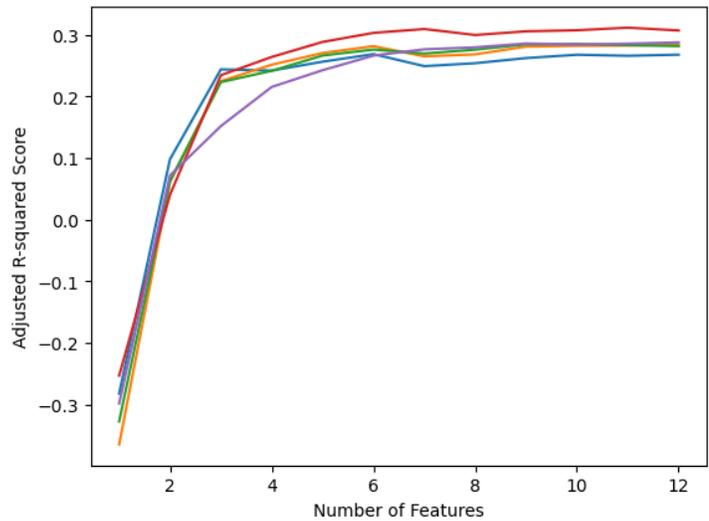
Figure 5-11: Optimal feature selection for predicting connection duration using RF method: RFECV analysis.
