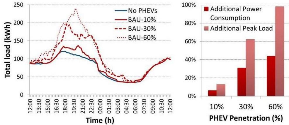
Figure 1-3: Impact of EV penetration on the power [13].
