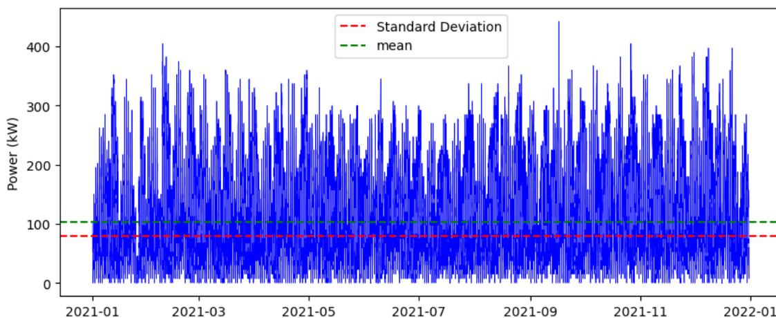
Figure 6-5: Aggregate power consumed during charging per minute.
