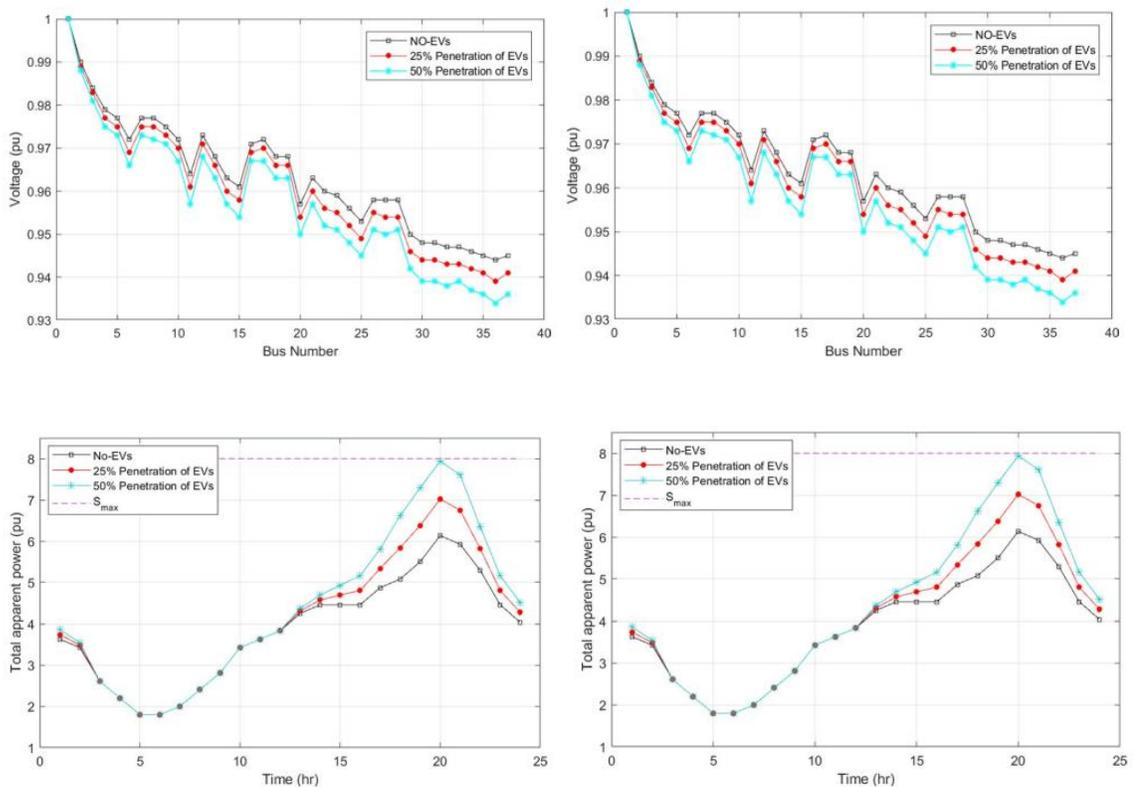
Figure 1-2: The impact of EV penetration on the distribution system [9].
