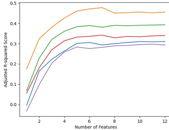
Figure 5-7: Optimal feature selection for predicting charging demand using RF method: RFECV Analysis.
