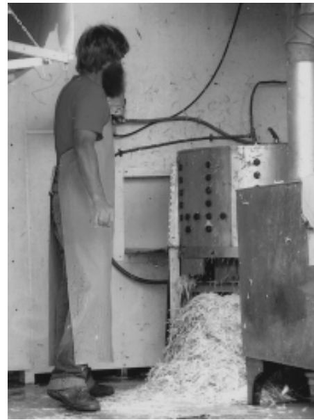
Figure 4. The two main pieces of processing equipment are the scalding tank on the right and the picker on the left.
