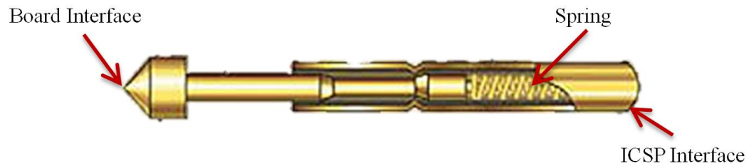
Figure 4.34: Cross section view of a pogo pin.
