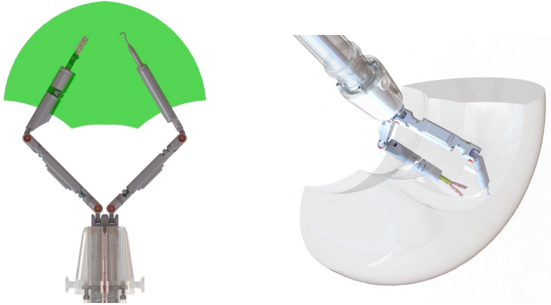
Figure 4.6: Left: EB2.0 superimposed on top of a slice of the intersecting robotic workspace at \theta_1 = 0 degrees. Right: EB2.0 with the intersecting workspace of the device.
