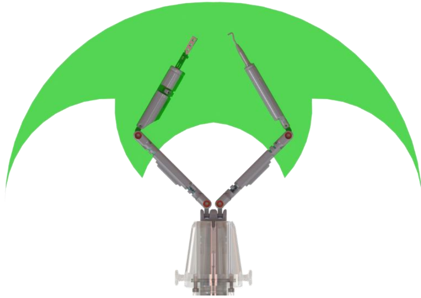
Figure 4.5: EB2.0 superimposed on top of a slice of the entire robotic workspace at \theta_1 = 0 degrees.
