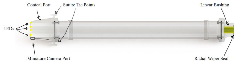
Figure 4.40: Cross section view of the insertion device for EB2.0.
