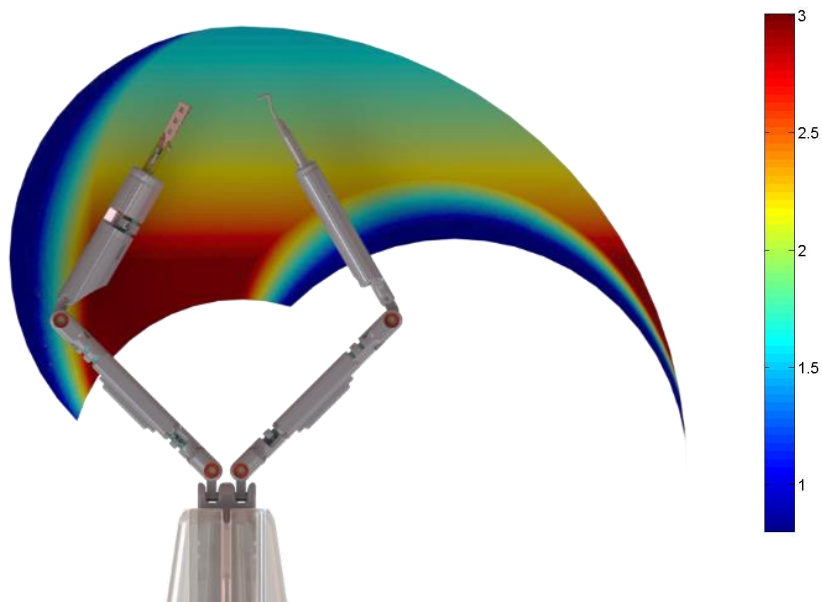
Figure 4.11: EB2.0 minimum static endpoint force, right arm (Forces are in Newtons with a scale from 0.8-3 [N]).
