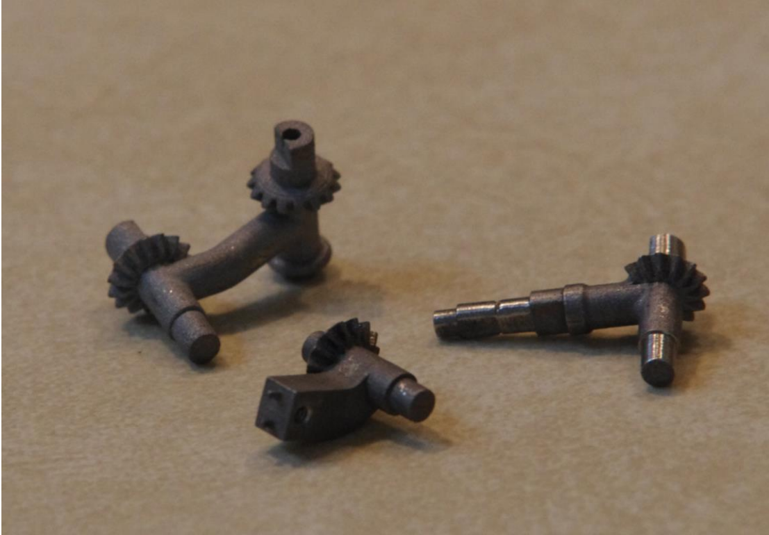
Figure 4.24: Lost wax investment cast bevel gears. The bearing seats on the far right part have been touched up. The other two parts are as cast.
