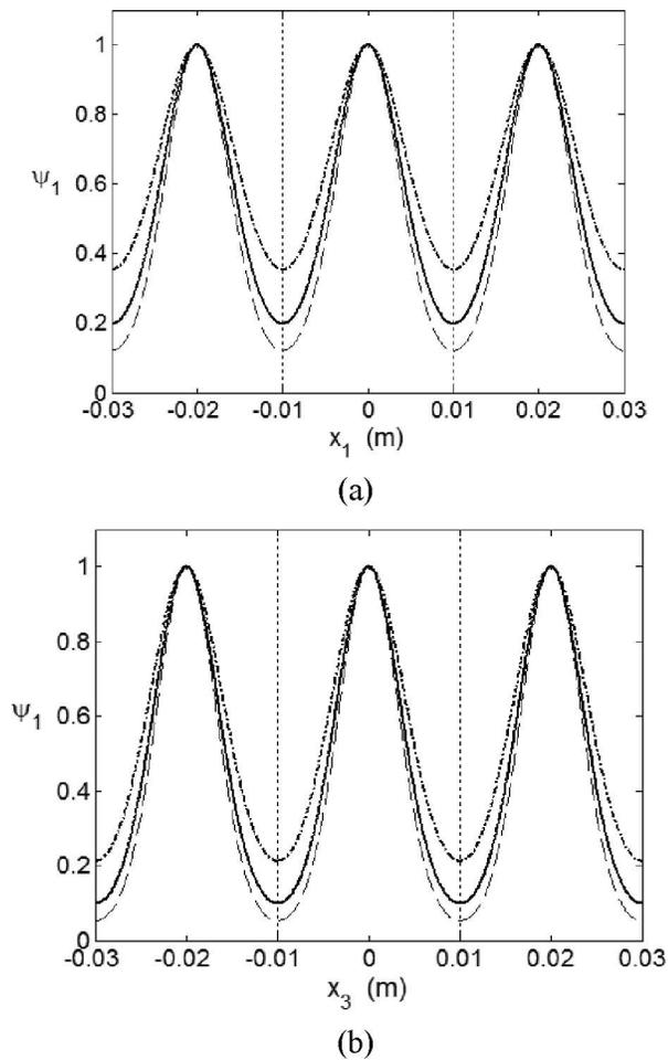
Fig. 4. Effects of  $R_0$  on vibration distribution of the first mode along (a)  $x_1$  and (b)  $x_3$  in a  $3 \times 3$  array: dash-dotted line:  $R_0 = 3\%$ ; solid line:  $R_0 = 5\%$ ; dashed line:  $R_0 = 7\%$ .
