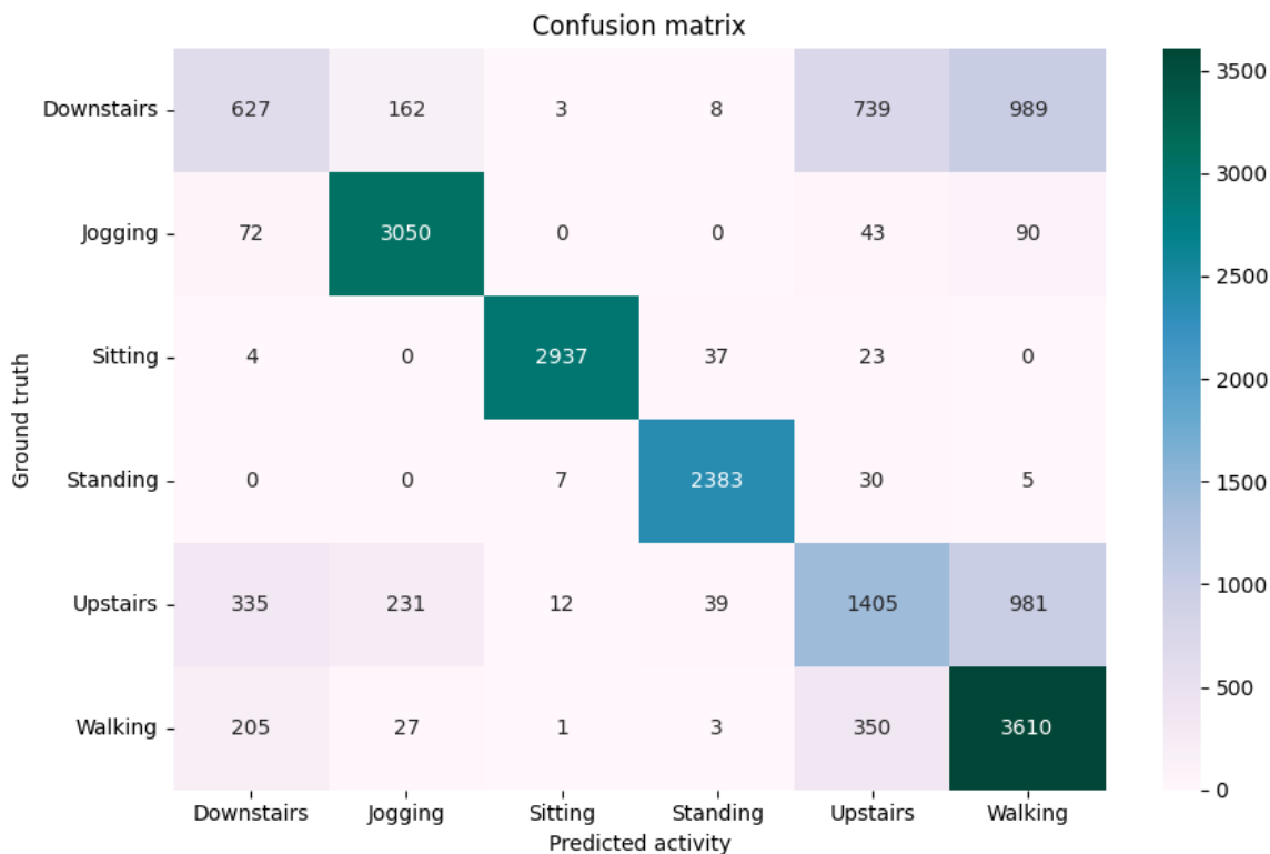
Figure A.15 Confusion matrix of RNN model run for 50 epochs, network architecture 16-10-6, accuracy 68%.
