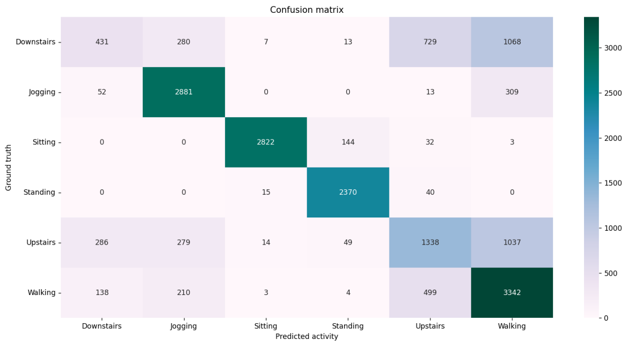
Figure A.12 Confusion matrix of CTRNN model run for 50 epochs, network architecture 4-10-6, 71.6%.
