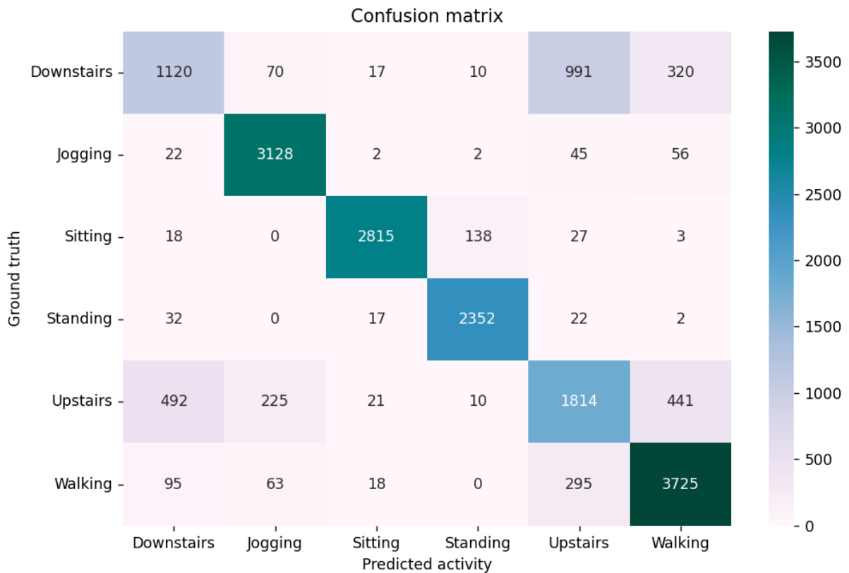
Figure A.14 Confusion matrix of RNN model run for 50 epochs, network architecture 32-10-6, accuracy 81.2%.
