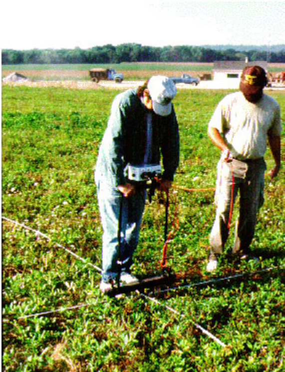
Figure 2. Forest Frost conducting a resistivity survey at Hopeton Earthworks, 1994.
