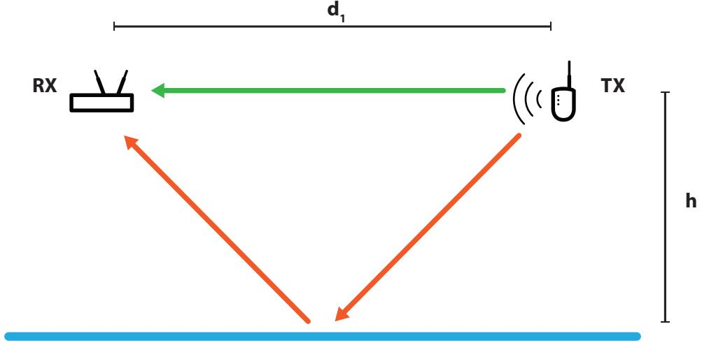
Figure 2.1.1: Two path RF propagation between a mobile transmitter (TX) and a fixed receiver (RX).
