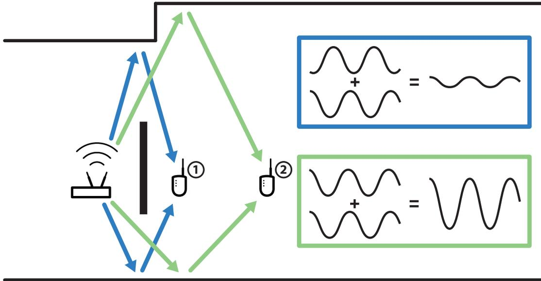
Figure 1.2.1: Multipath propagation effect on RSSI
