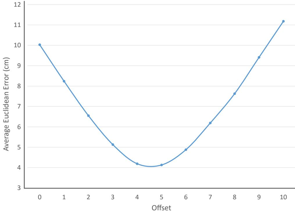
Figure 4.2.6: PF performance as a function of an output offset
