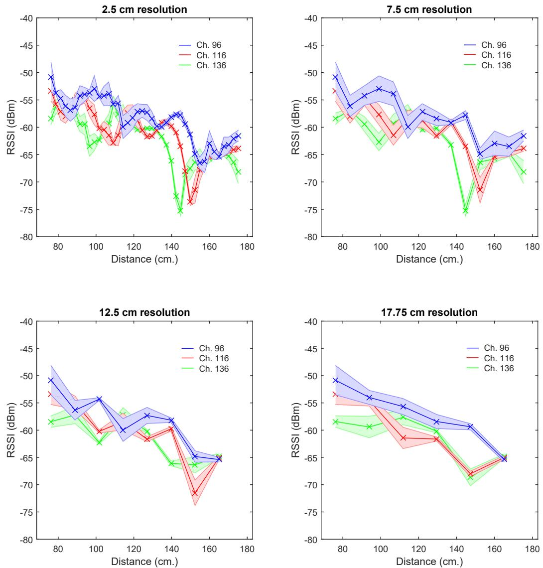
Figure 4.1.5: RSSI versus distance for different sampling resolutions
