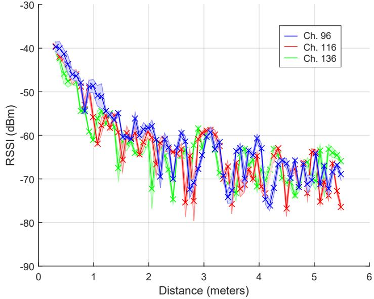
Figure 4.1.4: RSSI versus distance for line-of-sight between the anchor and watch
