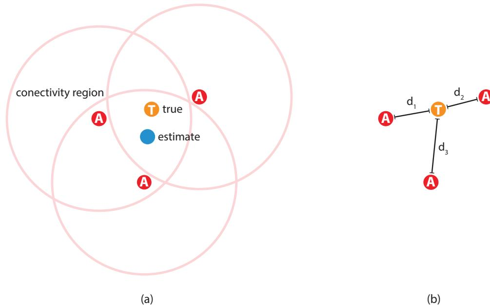
Figure 2.2.1: Sub-figure (a) illustrates range-free localization and (b) illustrates range-based localization.
