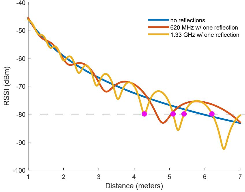
Figure 2.1.2: The plot shows RSSI as a function of distance for model in Figure 2.1.1. Two different frequencies are used.
