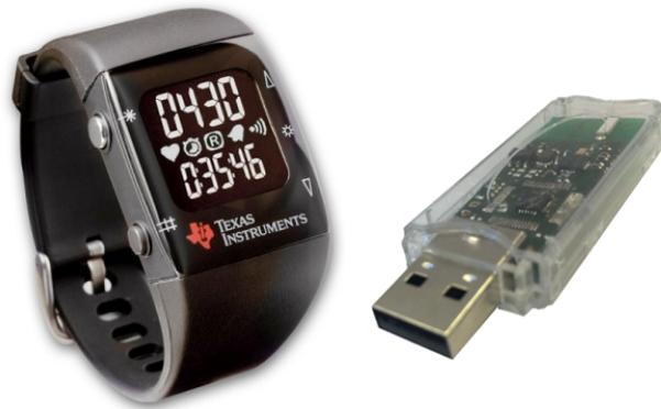
Figure 4.1.1: The TI's ez430-Chronos smart watch and Angelos Ambient
