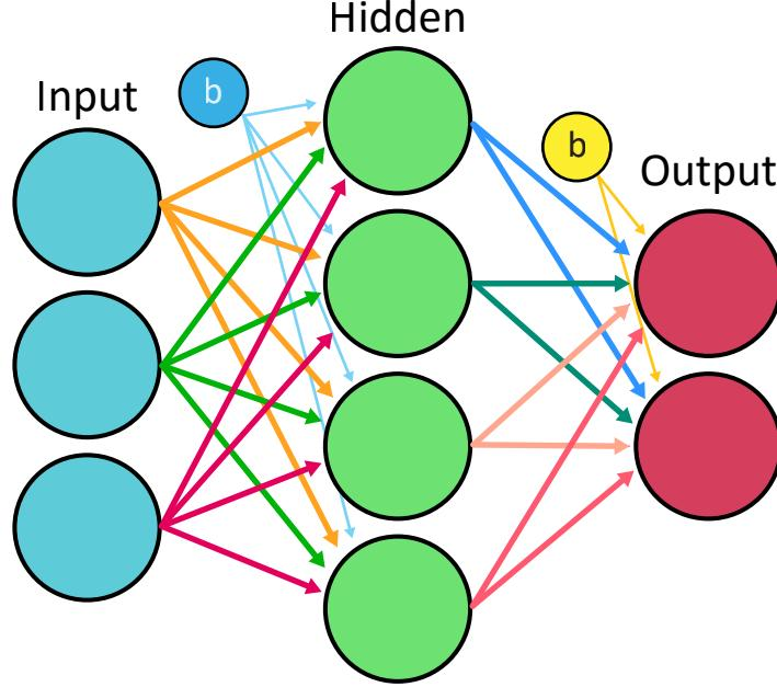
Figure 3.2.4: A three-layer feed-forward perceptron neural network
