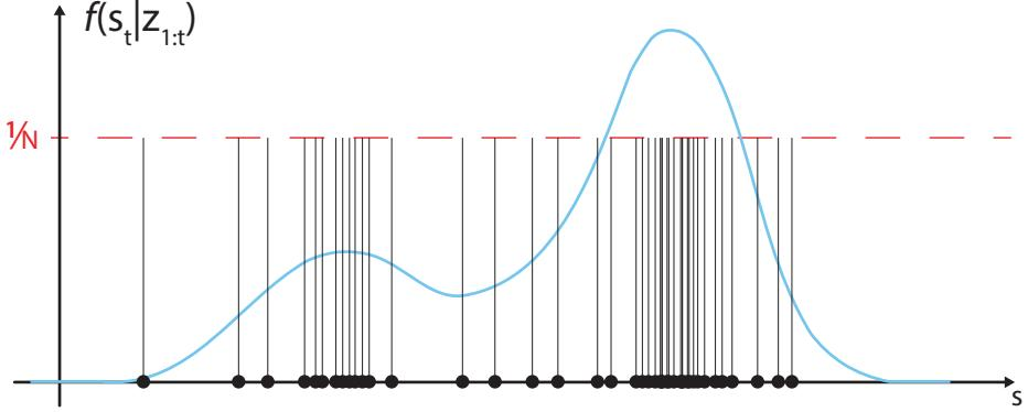
Figure 3.3.1: Particles approximate a non-Gaussian distribution
