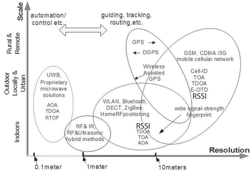
Figure 2.3.2: Outline of current wireless based positioning systems [109]
