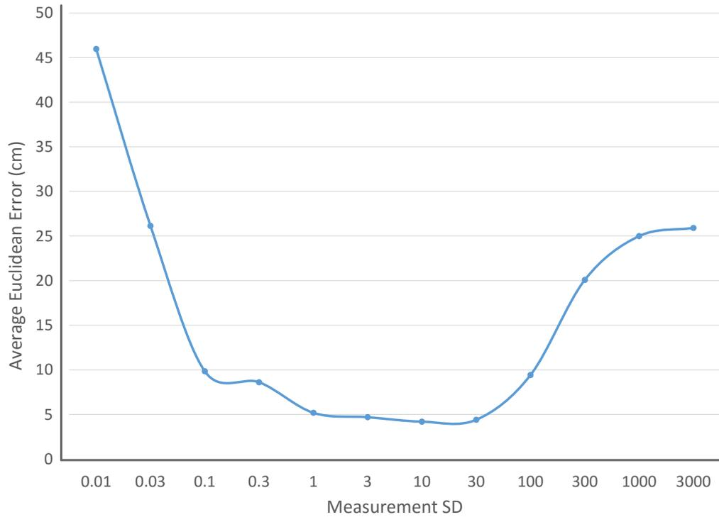
Figure 4.2.5: PF performance as a function of the measurement SD
