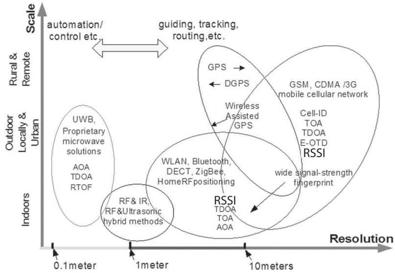
Figure 2.3.2: Outline of current wireless based positioning systems [109]
