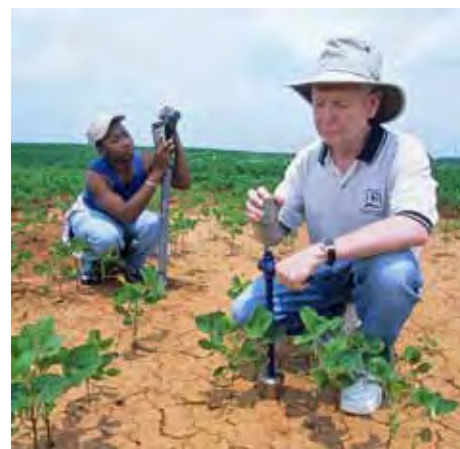
ARS hydrologist Tom Jackson and student Parmecia Jones use different methods to test soil moisture. The measurements will be compared to see which more accurately validates data obtained via satellites.
