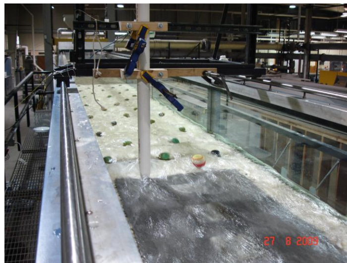
Figure 3.3 Perspective view of the prototype bridge pier during the high flow (bankfull condition) experiment
