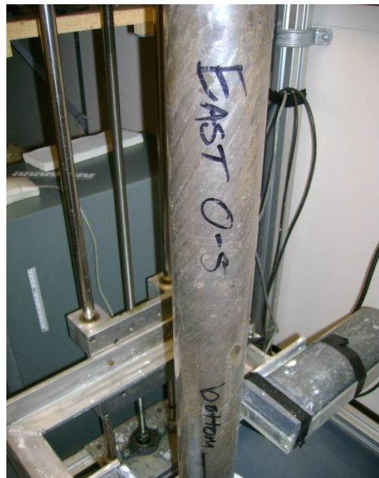
Figure 3.5 Measuring core bulk density. A section of the stream bank core was placed in a vertical frame. A ^{241}\text{Am} sealed source was moved up and down the core length in conjunction with a gamma energy detector on the other side of the core. The attenuation of the received radioactivity was indication of the core density.
