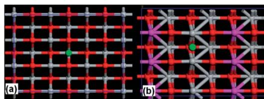
**Fig. 7** DFT calculation results for H adsorption on the surface of a perfect TiO (110) nanocrystal. (a) H adsorption before relaxation, where H is attached to the bridging site between two O atoms. (b) H adsorption after structural relaxation, where the H atom has moved to the bridging site between two Ti atoms. H, Ti and O atoms are designated by green, gray and red/pink spheres, respectively. For the relaxed structure, Ti atoms that show magnetic moments are designated by pink in (b).
