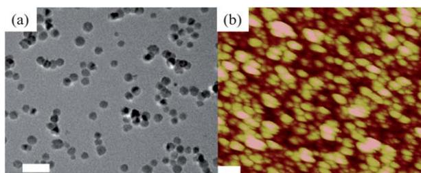
**Fig. 1** Images of TiO clusters: (a) Examination of cluster size with transmission-electron microscopy. (b) Examination of the film topography with atomic-force microscopy. For TEM examination, as-produced TiO clusters are deposited on a copper grid. For AFM examination, a TiO cluster film is fabricated on a silicon substrate. The scales are 50 nm (TEM) and 100 nm (AFM), respectively.
