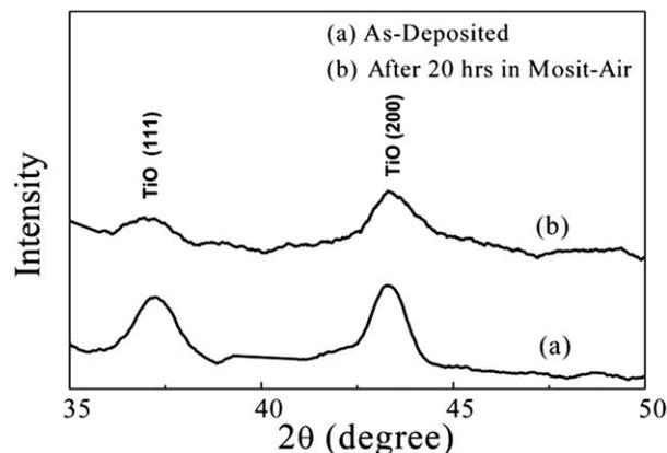
**Fig. 2** Structural analysis of the TiO cluster film with X-ray diffraction: (a) after deposition and (b) after exposure to moisture at a temperature of 50 °C for 20 hours. The rock salt structure is maintained after moisture exposure.
