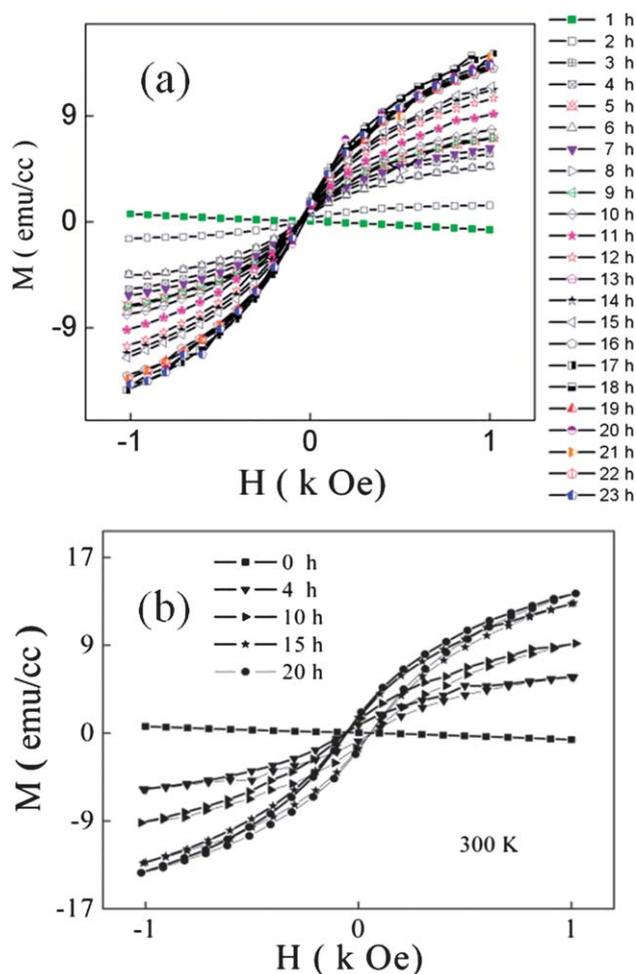
**Fig. 3** Evolution of magnetism for the TiO cluster film during exposure to moisture examined with SQUID: (a) half hysteresis loops for the TiO cluster film, measured after each hour of storage in moist air. (b) Representative hysteresis loops for the TiO cluster film after different durations in moist air (0, 4, 10, 15 and 20 hours).
