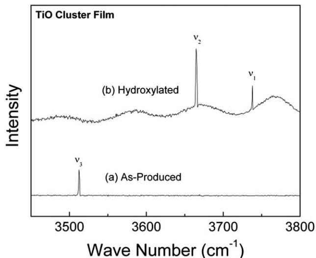
**Fig. 4** Raman spectra of the TiO cluster film: (a) after deposition and (b) after 20 hours of storage in moist air. As-produced clusters show a single peak at  $3512\text{ cm}^{-1}$  which can be attributed to adsorbed water. In contrast, after 20 hours of exposure to moisture, the Raman spectra of the cluster film show two peaks  $\nu_1$  at  $3664\text{ cm}^{-1}$  and  $\nu_2$  at  $3737\text{ cm}^{-1}$ , corresponding to the two nonequivalent hydroxyls.
