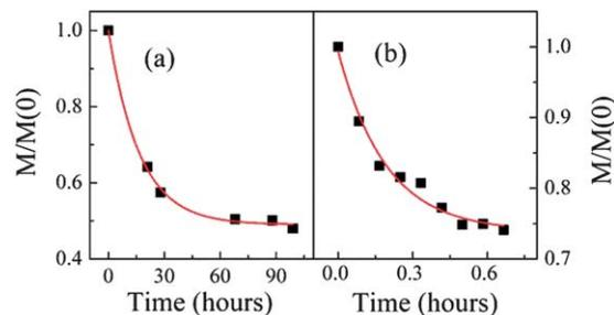
**Fig. 5** Magnetization relaxation for a TiO cluster film (squares): (a) relaxation in ambient air after reaching equilibrium in moist-air. (b) Relaxation of the magnetization of the TiO cluster film during oxygen annealing at  $450\text{ }^\circ\text{C}$  after reaching the equilibrium value in moist air. Solid lines are exponential fits.
