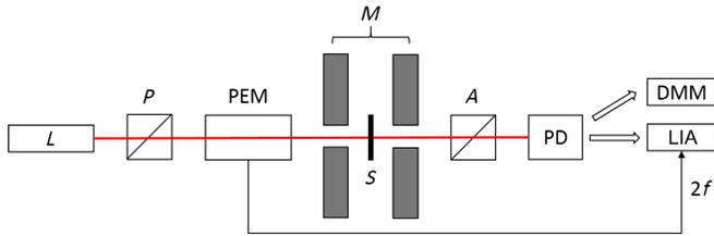
FIG. 1. Optical setup for EFIF effect. *L*, laser; *P*, polarizer; PEM, photoelastic modulator; *M*, electromagnet; *S*, sample inside ultra-high vacuum chamber; *A*, analyzer with automated rotational stage; PD, photodetector; DMM, digital multimeter; LIA, lock-in amplifier.
