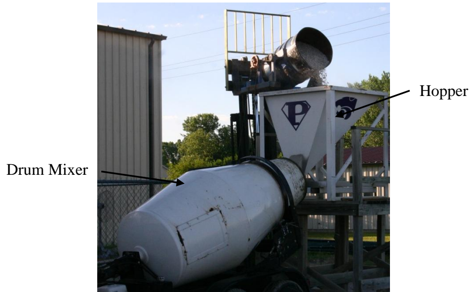
Figure 3.7 Adding Aggregates to Mixer
