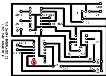
**Figure 4.2 Real sample with defect circled in red**
