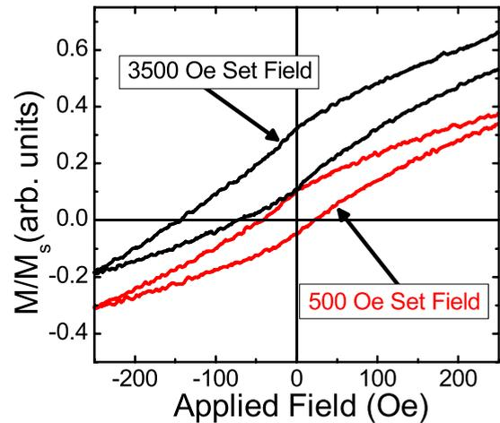
FIG. 2. (Color online) Two minor in-plane, [Co/Pt]/NiO magnetization loops, one from  $+3.5$  kOe to  $-250$  Oe and one from  $+500$  to  $-250$  Oe. The asymmetry in the in-plane magnetization increases with increasing set field.
