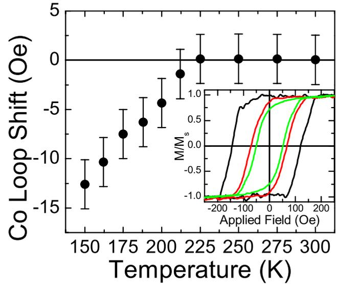
FIG. 4. (Color online) Co loop shift as a function of temperature. The loop shift decreases linearly with temperature with a  $T_B$  of 225 K. The inset shows the hysteresis loop at three representative temperatures (150, 225, and 300 K).
