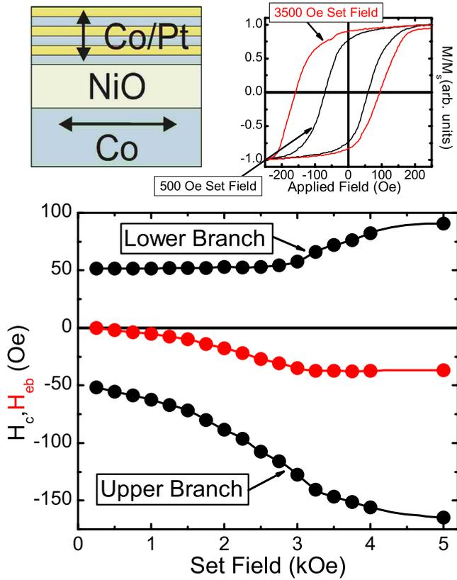
FIG. 3. (Color online) In-plane exchange bias of the Co/NiO/[Co/Pt] heterostructure as a function of  $H_{\text{set}}$ , where the structure is indicated in the upper left inset. The  $H_c$  for the upper and lower branches is also given; notice the lower branch shows no change until 2.75 kOe, above which the upper and lower branches show equal but opposite changes. Two representative loops taken at different  $H_{\text{set}}$  are shown in the upper right inset.
