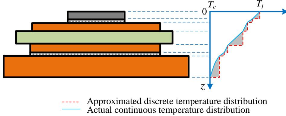
Fig. 3.3: Illustration of the temperature distributions in the layers of an IGBT module estimated by the conventional lumped Cauer-type TEC and the actual continuous temperature distribution of the IGBT module in the steady-state condition.
