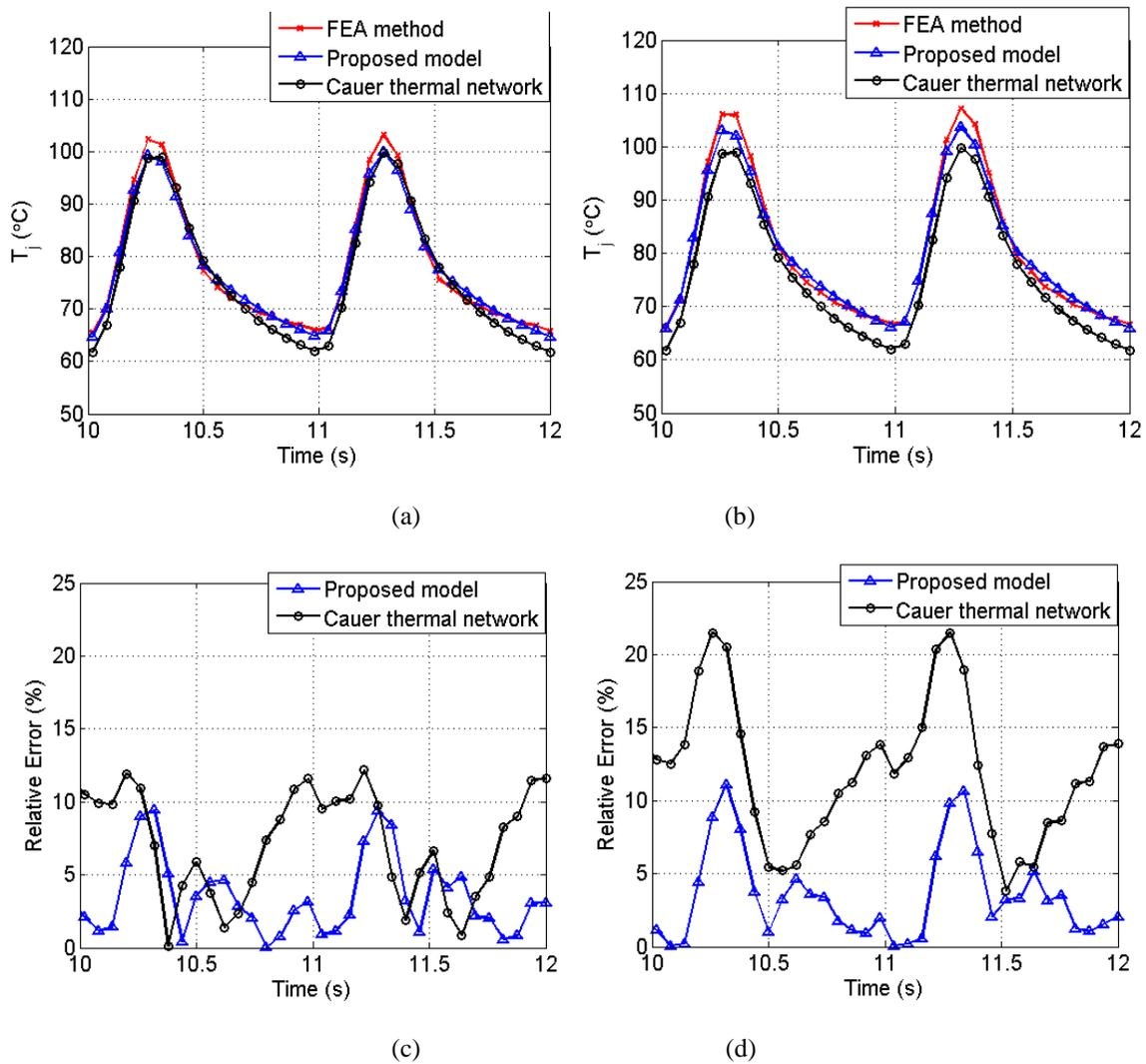
Fig. 5.12: Comparison of different models for the cases of 3.5-mm solder cracks and 5-mm solder cracks under the dynamic load condition: (a) junction temperature (3.5-mm solder crack); (b) junction temperature (5-mm solder crack); (c) relative error (3.5-mm solder crack); and (d) relative error (5-mm solder crack).
