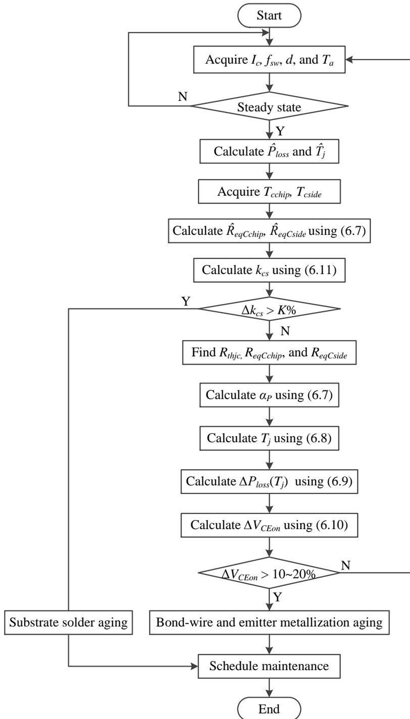
Fig. 6.3: The flowchart of the implementation of the aging monitoring method using two case temperatures.
