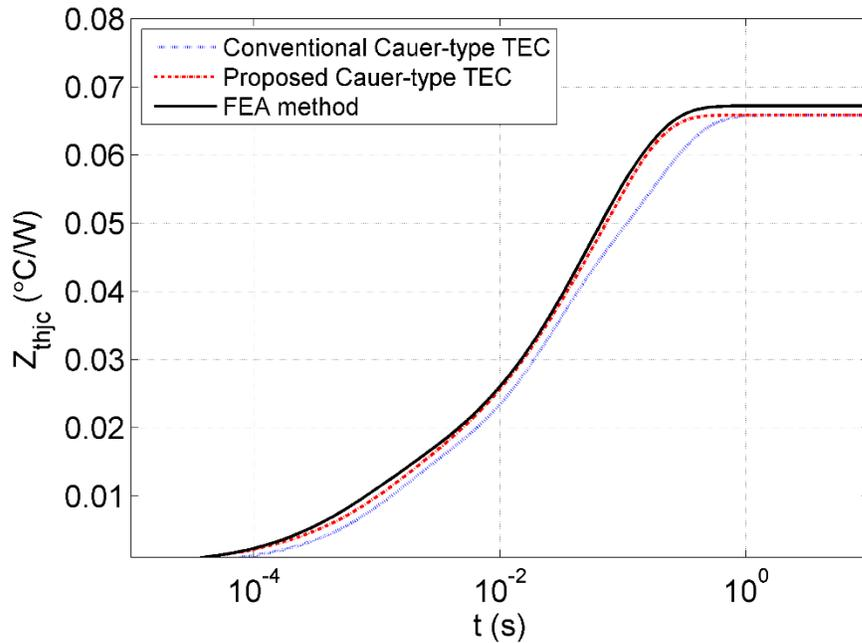
Fig. 3.6: Comparison of the transient thermal impedances from junction to case obtained from the conventional Cauer-type TEC model, the proposed Cauer-type TEC model, and the FEA model.
