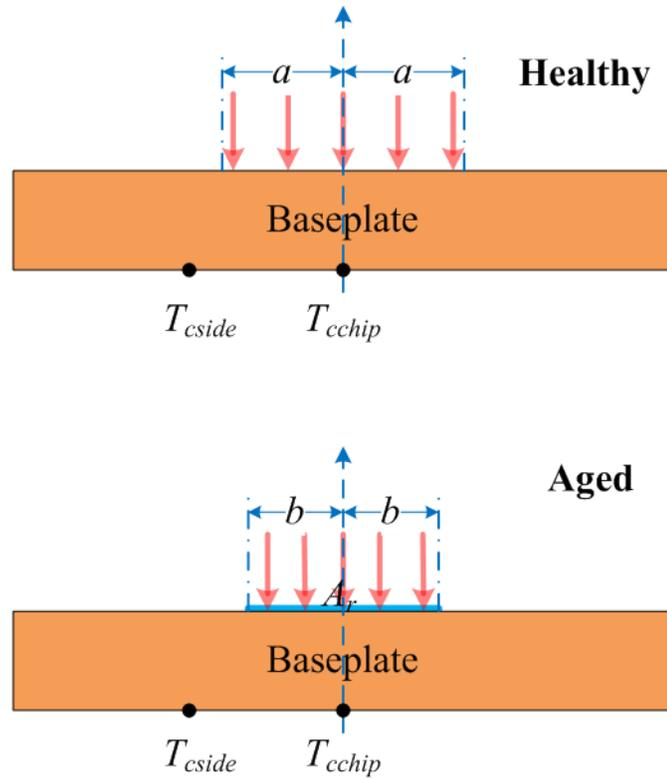
Fig. 5.3: IHCP using case temperature to estimate the effective heat flux area.
