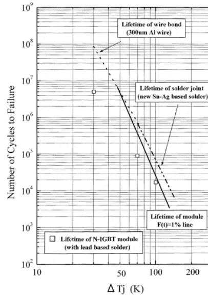
Fig. 1.4: An example of a power cycling curve [16].
