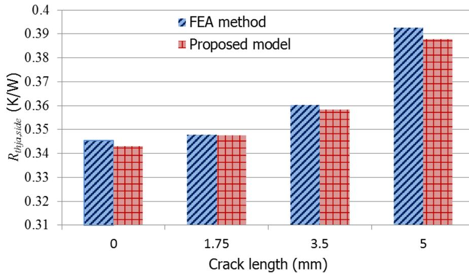
Fig. 5.11: Comparison of  $R_{thja,side}$  calculated by the FEA method and the proposed model.
