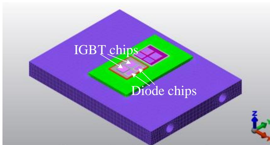
Fig. 3.5: The model of a CM400-12NF IGBT module with a cold plate built in Autodesk Simulation Multiphysics.
