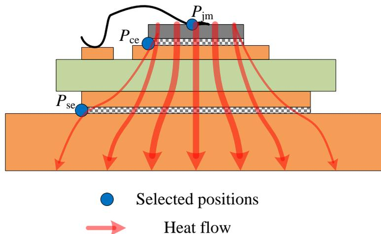
Fig. 7.2: Selected points and heat flows inside an IGBT module.
