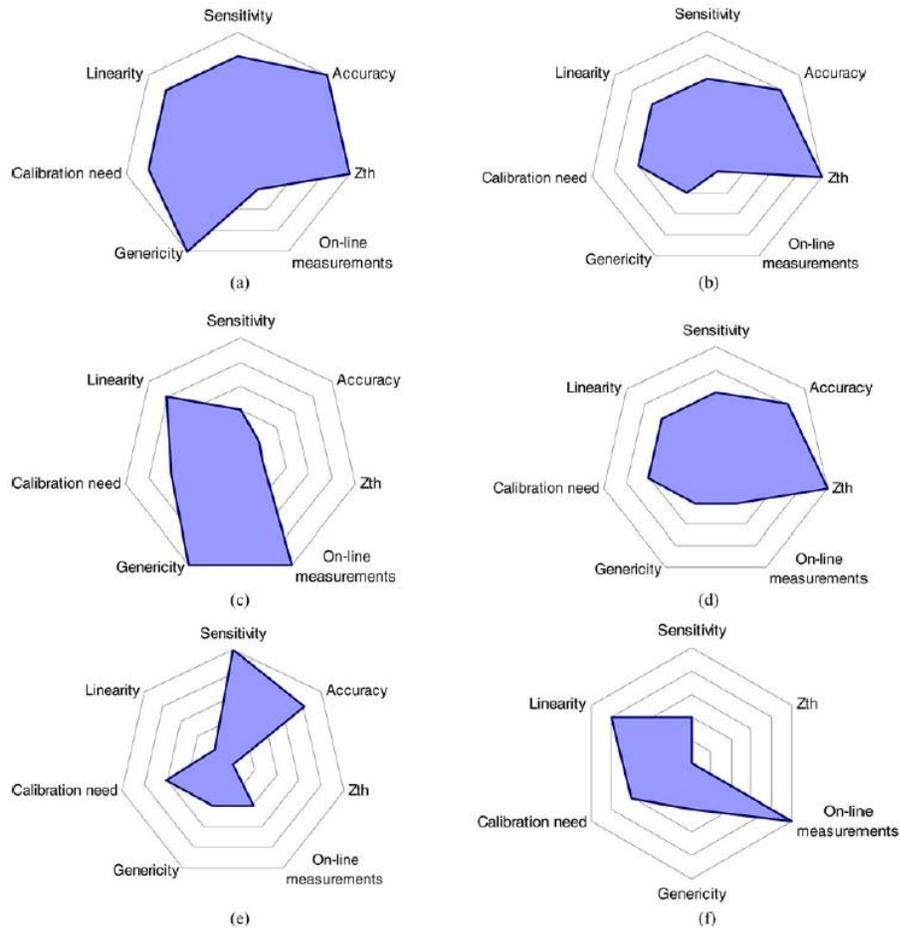
Fig. 2.4: Comparison of the different TSEPs [49]. (a) Voltage under a low current (diode, IGBT, MOSFET in OFF-state). (b) Threshold voltage. (c) Voltage under a high current. (d) Gate-emitter voltage. (e) Saturation current. (f) Switching times.
