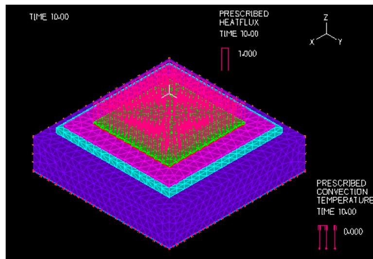
Fig. 7.7: FEA model of the general IGBT module.
