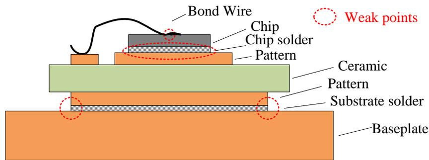
Fig. 1.3: Architecture of an IGBT module with the weak points circled by dashed lines.
