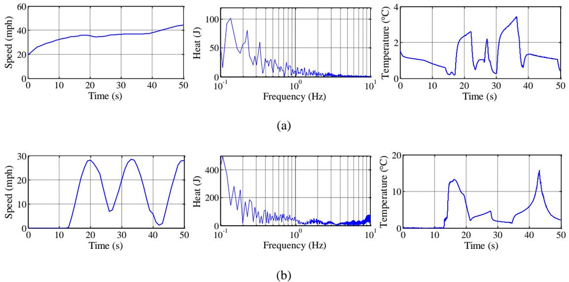
Fig. 7.10: Speeds of HEV, frequency spectra of heat generation, and temperatures of  $P_{se}$  for loading (a) and loading (b).
