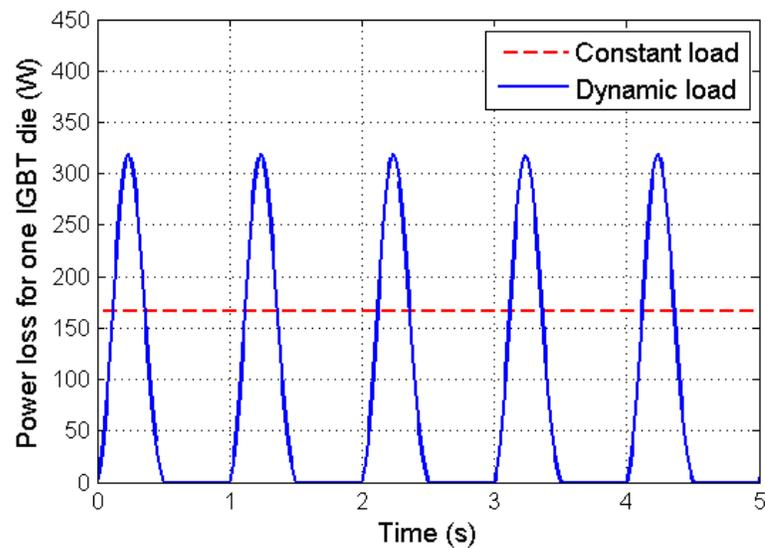
Fig. 5.9: Power loss profiles of constant load and dynamic load cases for one IGBT chip.
