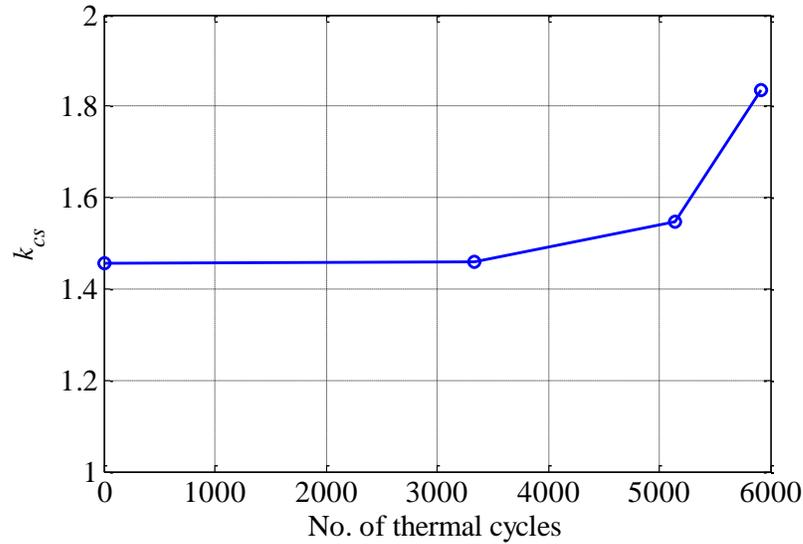
Fig. 6.11: Evolution of  $k$  during the thermal cycling test of the IGBT module.
