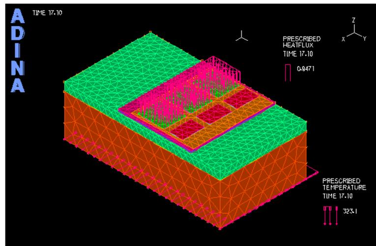
Fig. 5.6: The model of one-sixth of a CM1400 IGBT module built in ADINA.
