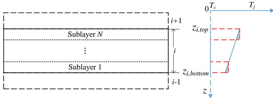
Fig. A.1: The temperature distribution approximation error of the  $i$ th layer subdivided into  $N$  sublayers.
