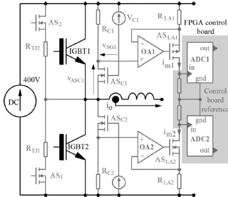
Fig. 2.3:  $V_{CEon}$  measurement scheme (parallel diodes are not drawn) in [46].
