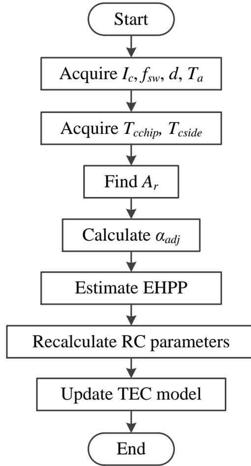
Fig. 5.5: Schematic of the proposed online adaptive TEC model.
