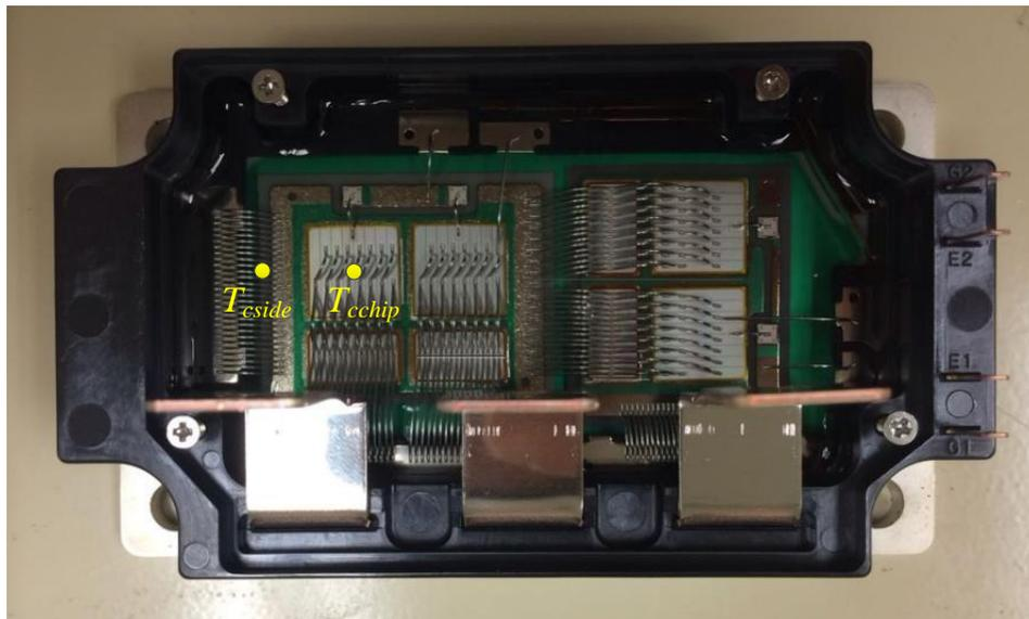
Fig. 6.4: The test IGBT module with the positions of the two thermal sensors placed on the bottom surface of the baseplate (top view from the upper side of the module).
