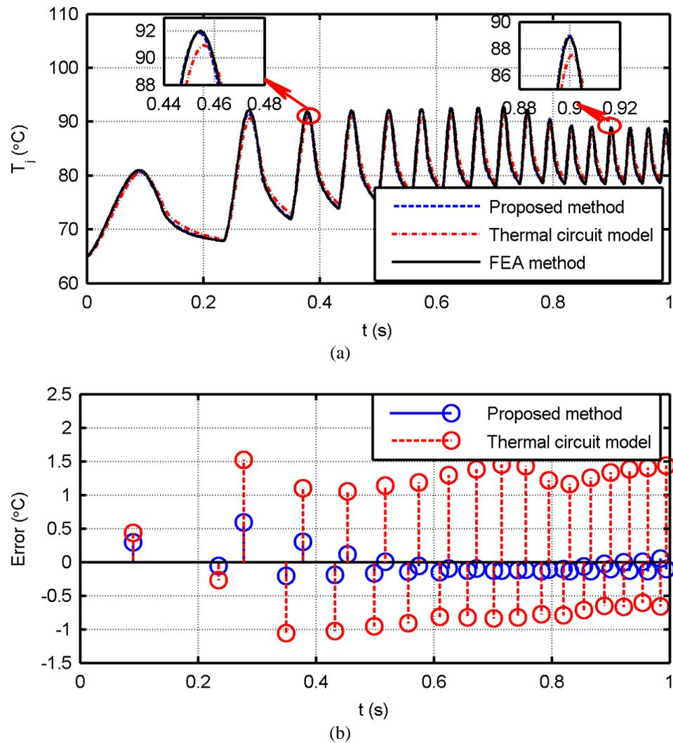
Fig. 7.5: Comparison of  $T_j(t)$  estimated by the three methods when the inverter was operated with a transient load: (a) junction temperature and (b) error at peaks and valleys with respect to the FEA method.
