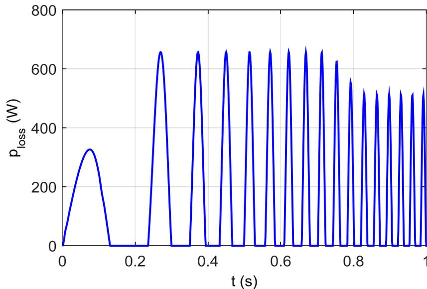
Fig. 4.4: Total power loss profile of the IGBT chips in one switch of the IGBT module in a transient load condition.
