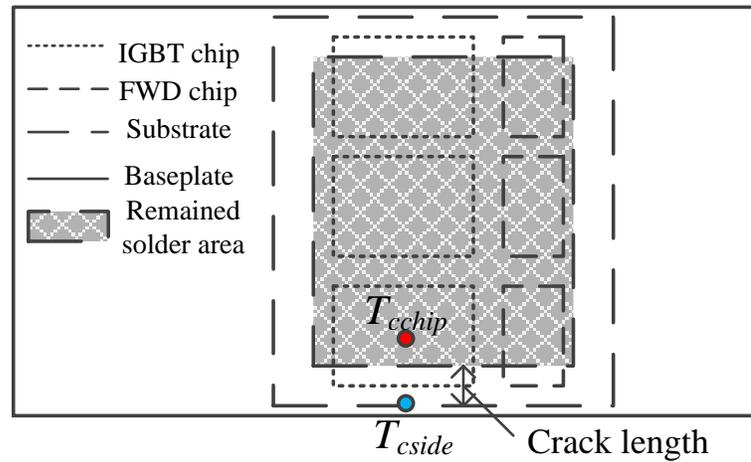
Fig. 5.7: Baseplate side view of the IGBT module.
