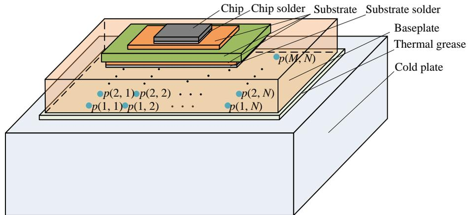
● Selected points at the bottom surface of the baseplate for 2D case temperature measurements
