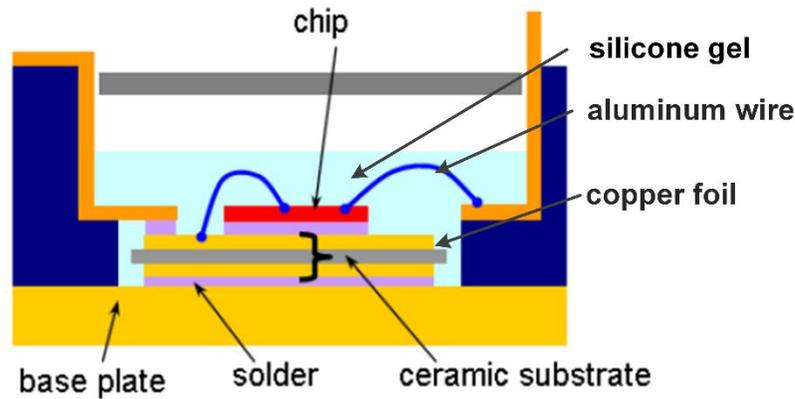
Fig. 1.2: Cross-sectional view of the structure of a Mitsubishi IGBT module [7].
