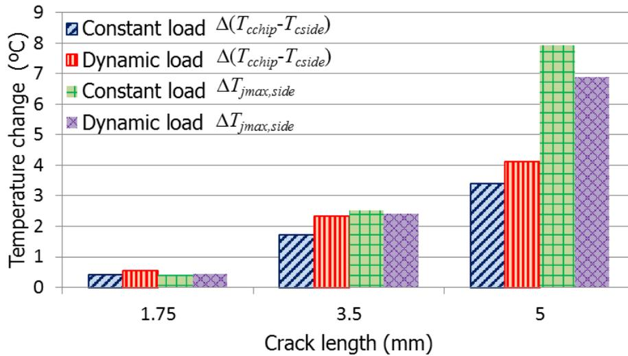
Fig. 5.10: Changes in nonuniformity of the case temperature distribution and maximum junction temperature in the three substrate solder crack cases in constant and dynamic load conditions.
