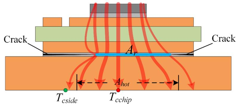
Fig. 5.2: The EHPP in an IGBT module when cracks developed from the edge to the center in the substrate solder layer.
