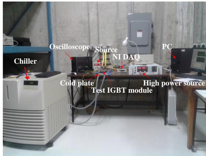
Fig. 6.8: Experimental setup for validation of the proposed method: (a) the schematic and (b) the actual setup.
