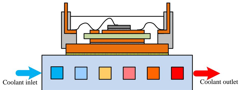
Fig. 4.1: An IGBT module (only one chip is shown) cooled by a cold plate.
