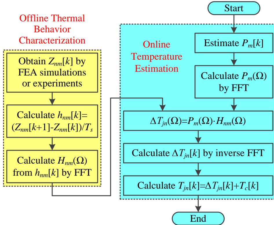
Fig. 7.1: The flowchart of the proposed method.
