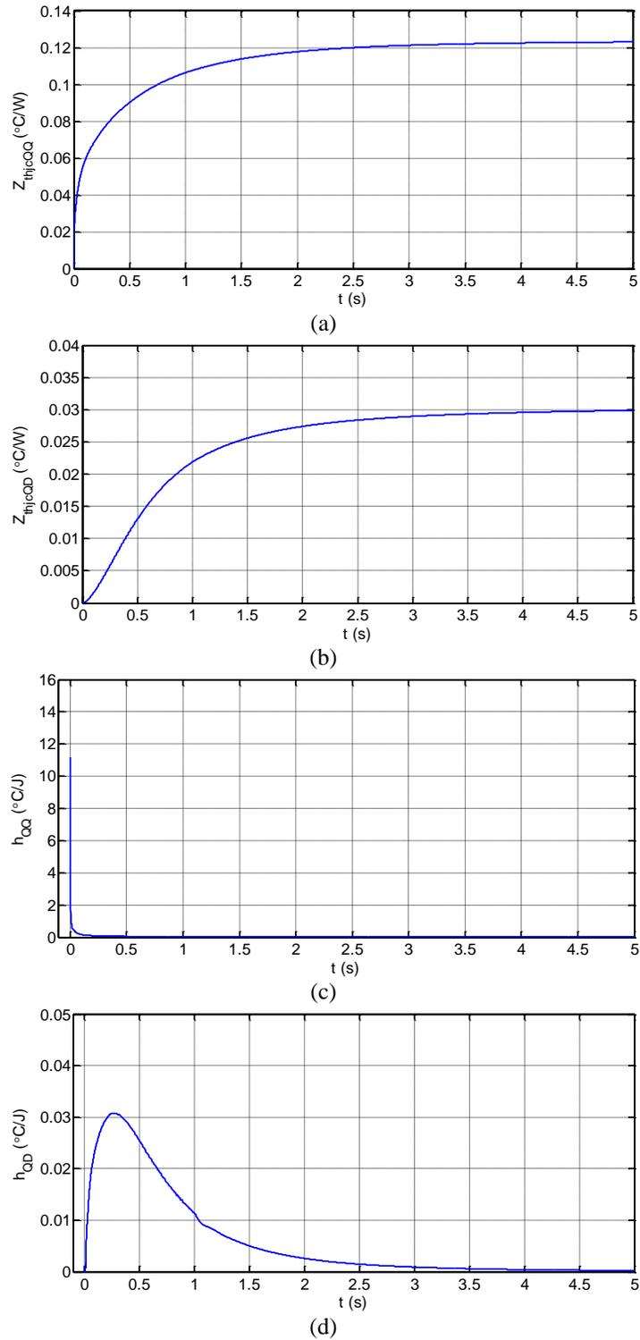
Fig. 7.4: The transient thermal impedance responses from the junction of the IGBT chip to the case and the corresponding LTI system responses: (a)  $Z_{thjcQQ}(t)$ ; (b)  $Z_{thjcQD}(t)$ ; (c)  $H_{QQ}(t)$ ; and (d)  $H_{QD}(t)$ .
