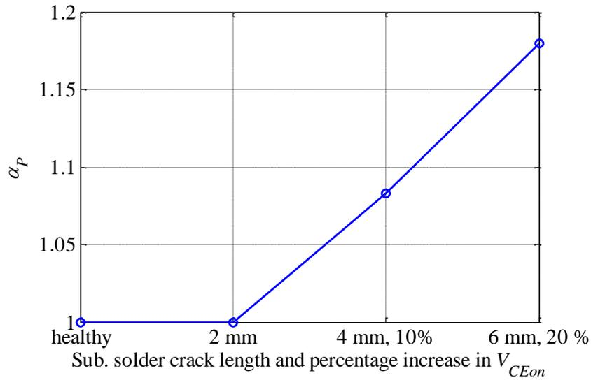
Fig. 6.7: Calculated  $\alpha_P$  during the aging process of the IGBT module.
