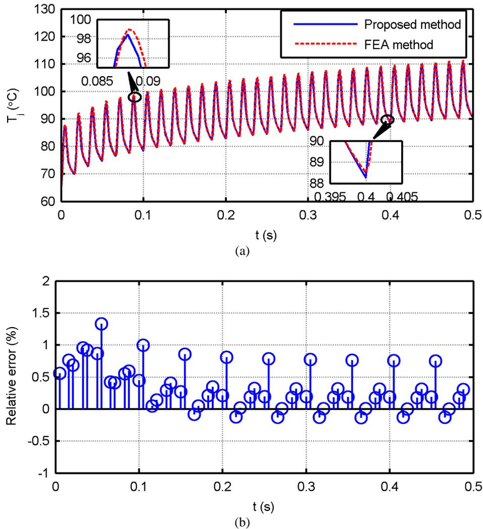
Fig. 7.6: Comparison of  $T_j(t)$  estimated by the proposed method and the FEA method when the inverter was operated at a constant operating condition: (a) junction temperature and (b) relative error at peaks and valleys with respect to the FEA method.
