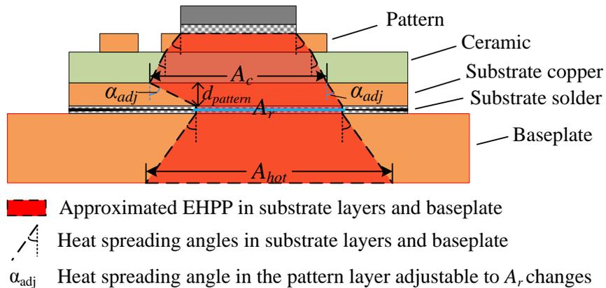
Fig. 5.4: The approximated EHPP for an IGBT module with substrate solder cracks.
