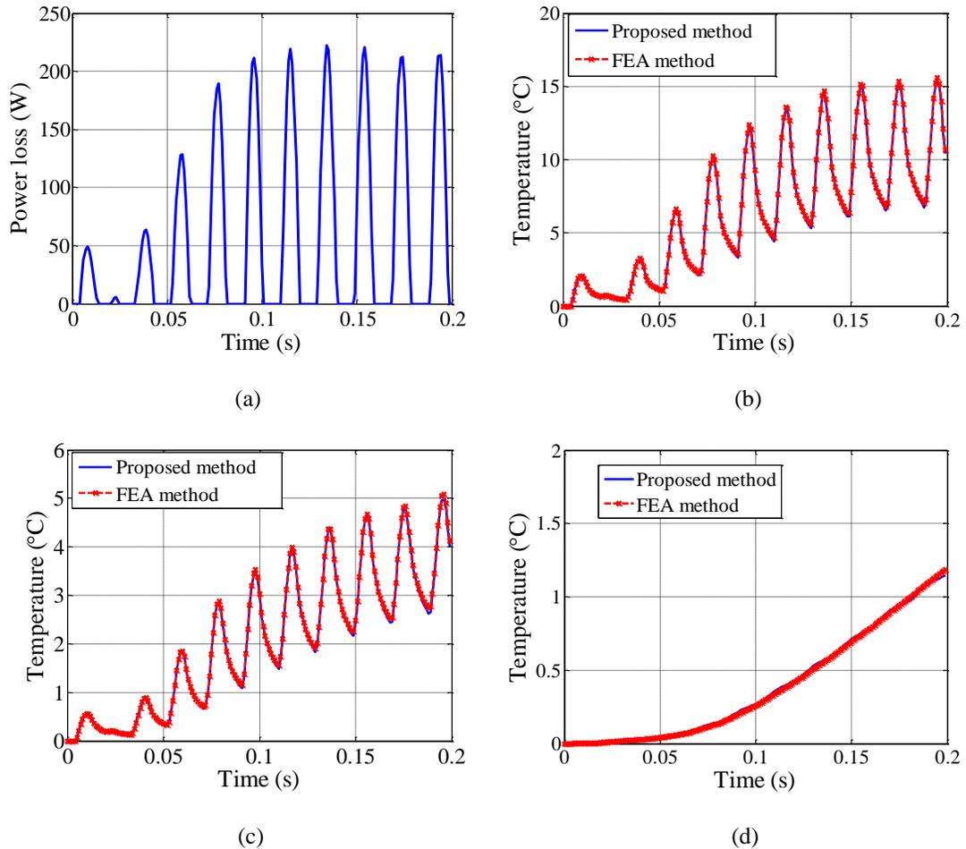
Fig. 7.9: Comparison of the proposed method with the FEA method. (a) The power loss and the transient temperatures estimated by the two methods at (b)  $P_{jm}$ , (c)  $P_{ce}$ , and (d)  $P_{se}$ .
