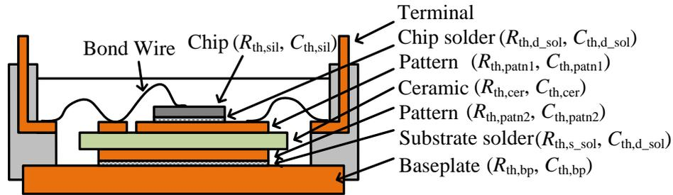
Fig. 3.1: The architecture of an IGBT module with Cauer-TEC RC parameters.
