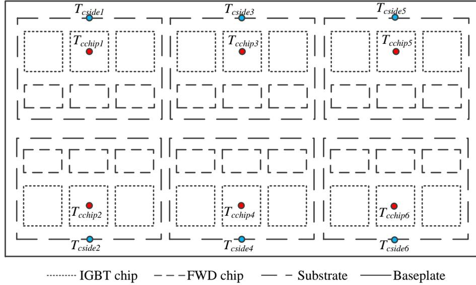
Fig. 6.2: The placement of thermal sensors on the bottom surface of the baseplate of a three-phase inverter module having six IGBT switches.
