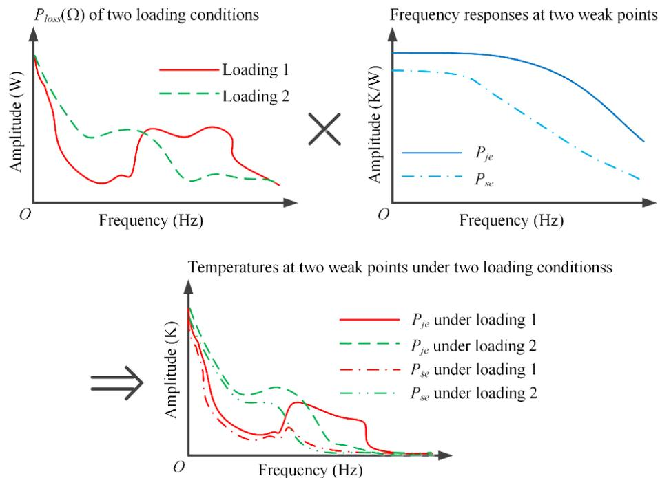
Fig. 7.3: Temperature information of  $P_{jm}$  and  $P_{se}$  under two different loading conditions.
