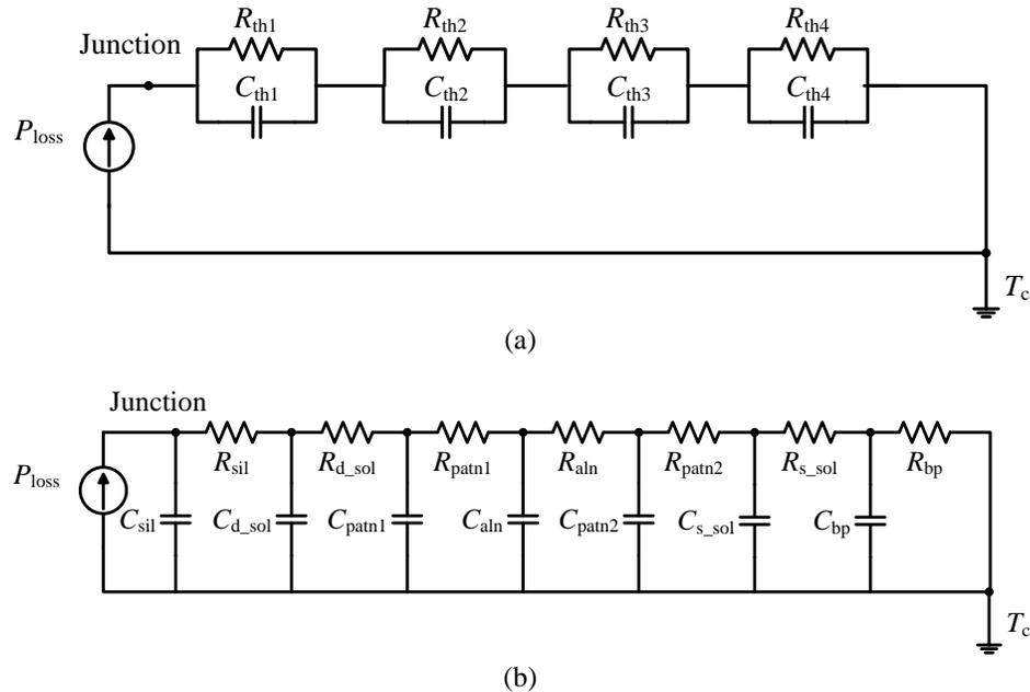
Fig. 2.1: TEC thermal models: (a) Foster-type and (b) Cauer-type.
