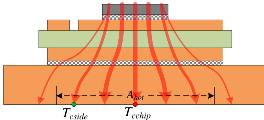
Fig. 5.1: The EHPP in a healthy IGBT module.
