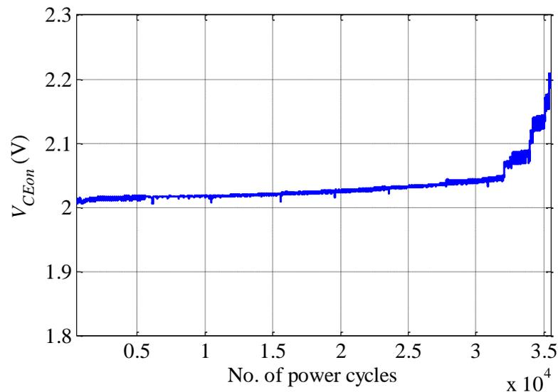
Fig. 6.12: Evolution of  $V_{CEon}$  during the power cycling test of the IGBT module.
