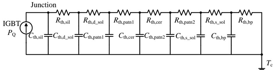
Fig. 3.2: The conventional lumped Cauer-type TEC for an IGBT module.
