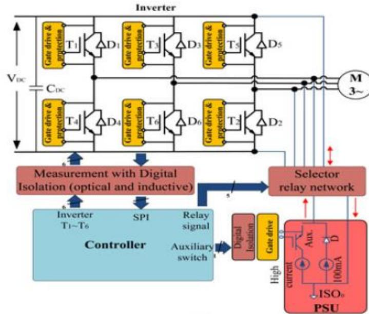
Fig. 2.2: Schematic diagram of the in situ measurement circuitry for IGBTs on electric vehicles in [45].
