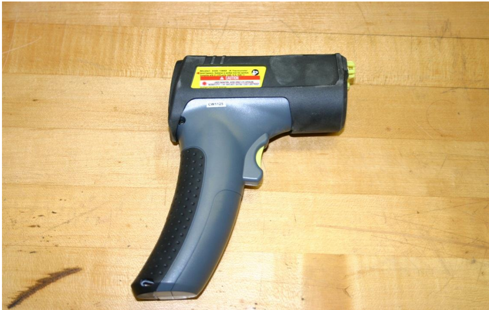
Figure 2.15 Infrared thermometer used to measure temperature of steel rail
