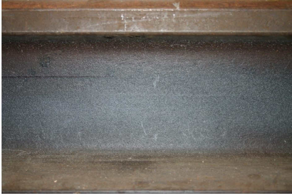
Figure 2.1 Steel rail with paint to protect surface correlation
