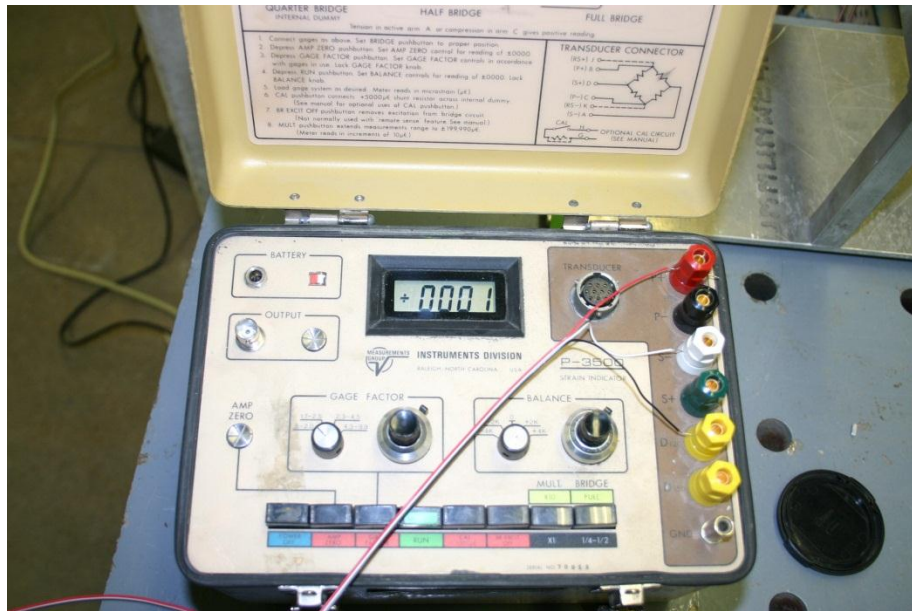
Figure 2.13 P-3500 Strain Indicator used to read strain gauge values
