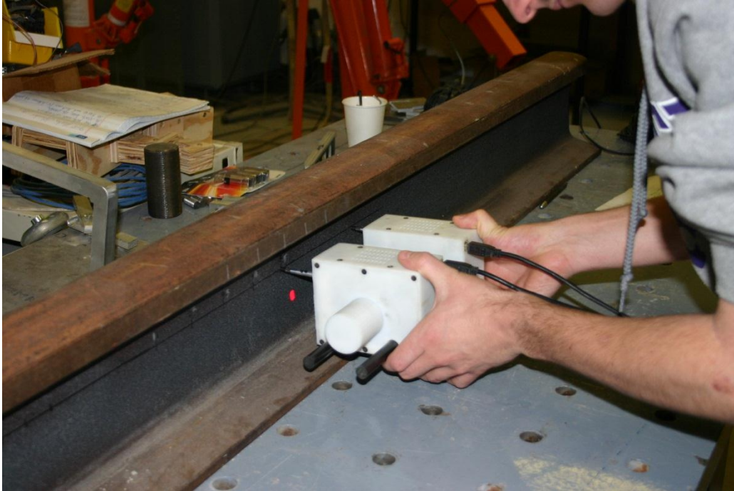
Figure 2.2 Taking base readings using the hand held method
