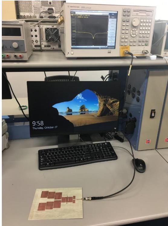
Figure 4.42 Measurement of prototype 1.90GHz Yagi-Uda patch antenna (1)
