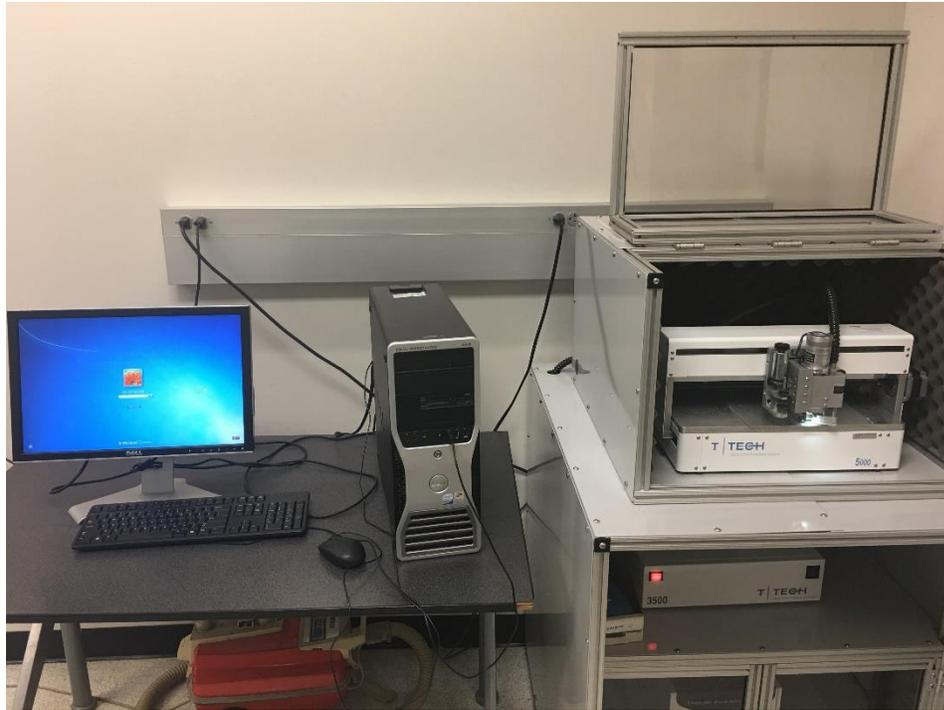
Figure 4.37 The T Tech mill machine controlled by a computer
