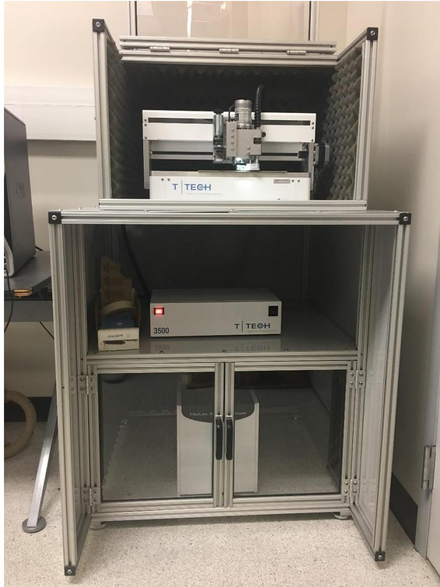
Figure 4.36 The T Tech mill machine used to build the proposed antenna
